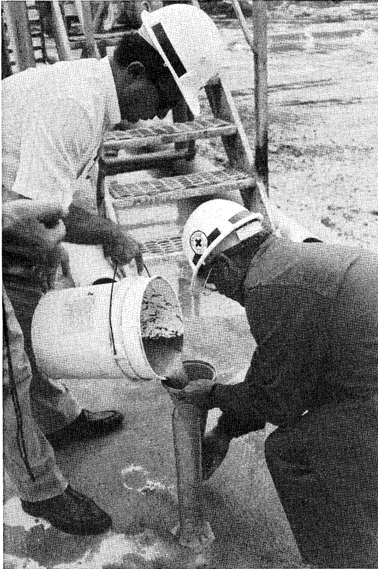
Figure 5. Filling Marsh flow cone with grout sample
