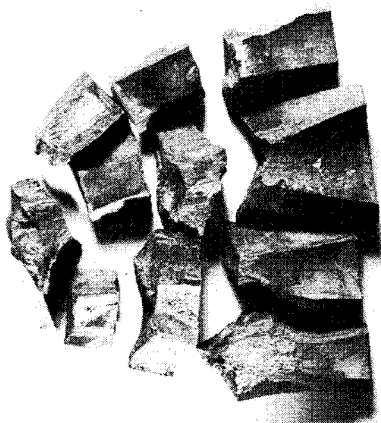
(c) 8 Parts tantalum carbide and 1 part zirconium carbide.
