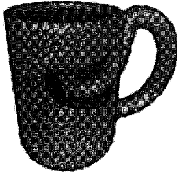
Figure 7.3: A Klein mug , a variation on the famous 1-sided surface. The handle and sidewalls are controlled by cylinder tools. Variational blend surfaces join the cylinders into a globally smooth, non-orientable surface. A hole has been cut in the side to show “interior” structure.
