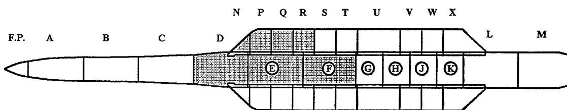
Figure 25. Compartment Flooded - Case 10.
