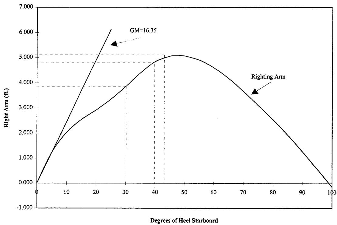
Figure 20. Case 6, Righting Arm and GM Curve.
