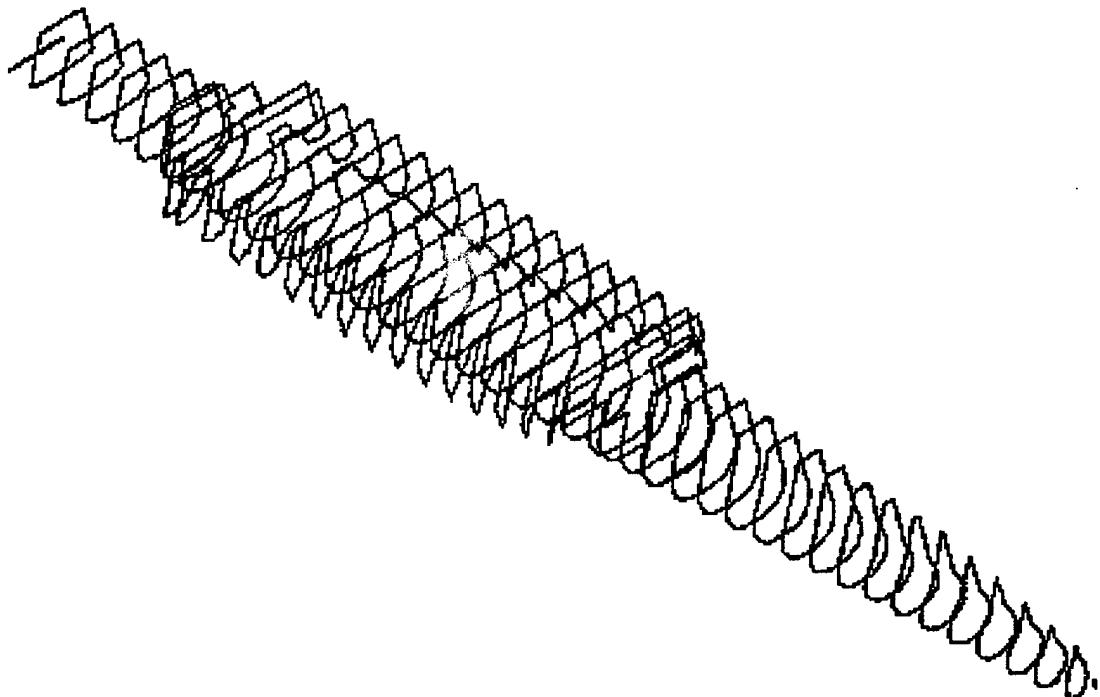
**Figure 2. Isometric Projection of Trimaran's Hull.**
