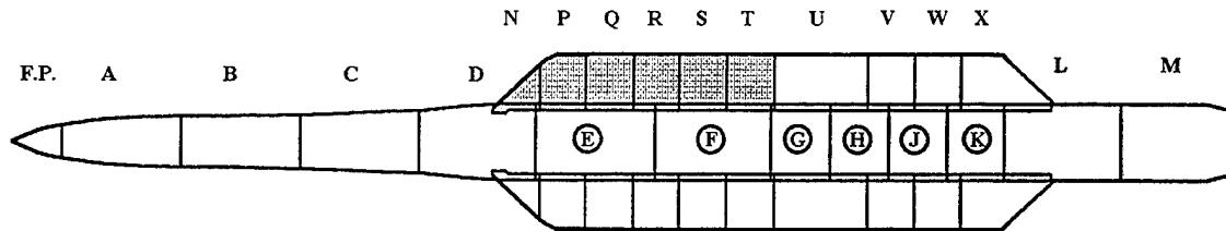
Figure 21. Compartment Flooded - Case 7.
