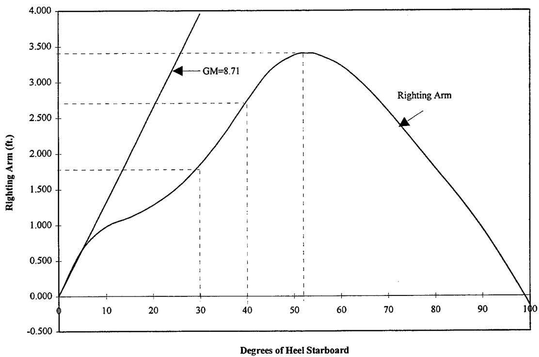
**Figure 18. Case 5, Righting Arm and GM Curve.**
