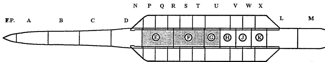
Figure 19. Compartment Flooded - Case 6
