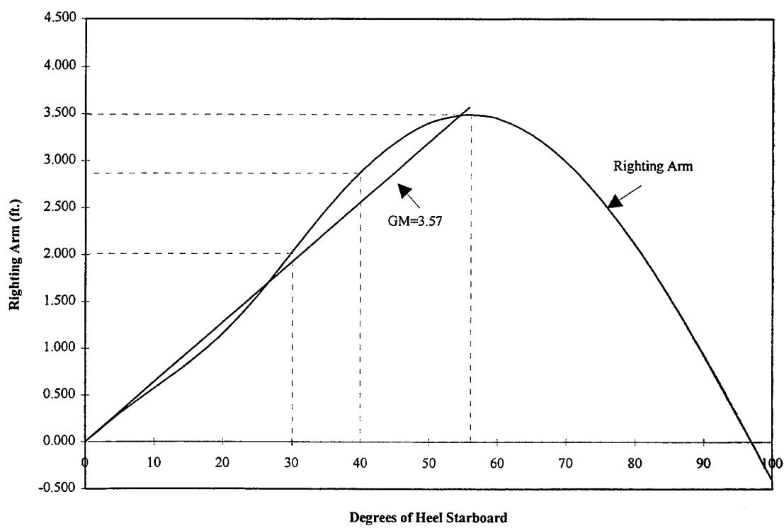
**Figure 12. Case 2, Righting Arm and GM Curve.**
