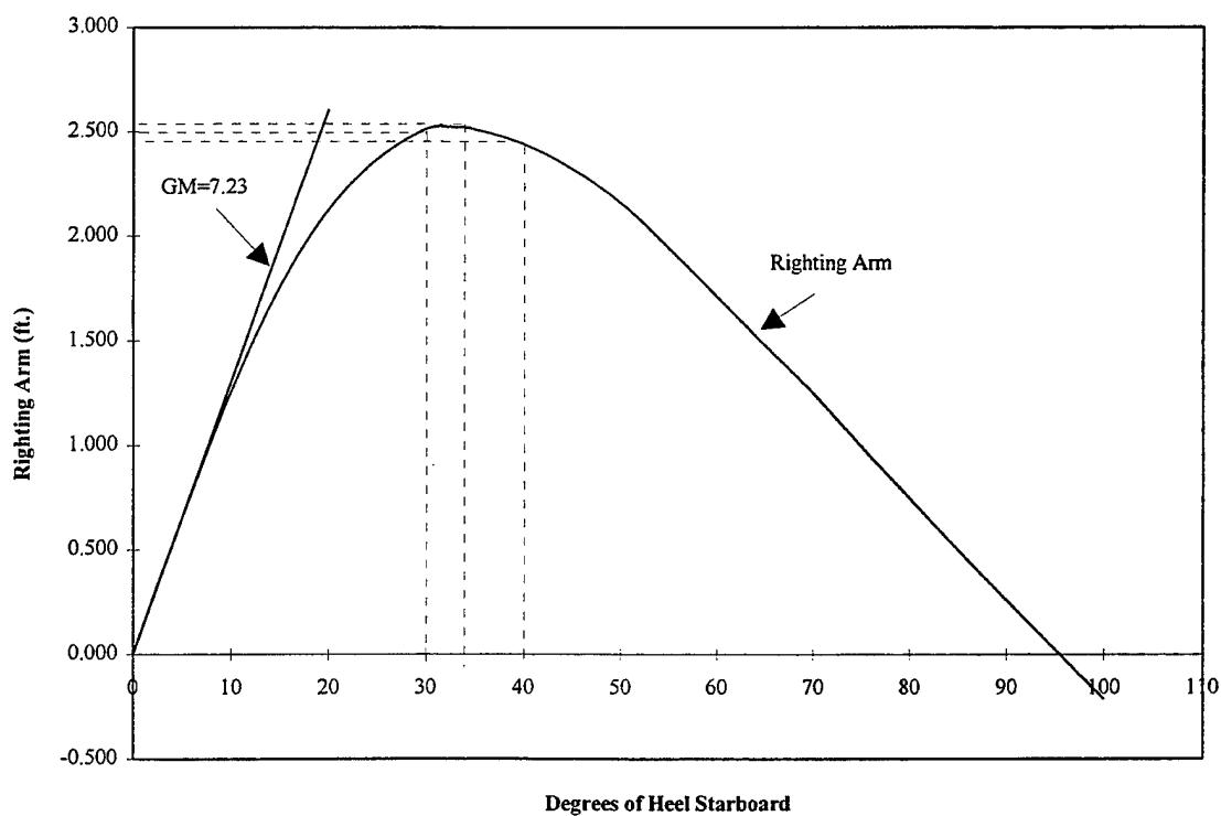
Figure 14. Case 3, Righting Arm and GM Curve.
