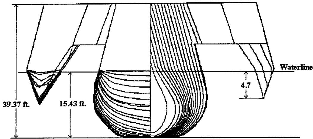
**Figure 5. Trimaran Hull, Body Plan.**
