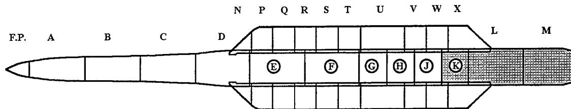
**Figure 17. Compartment Flooded - Case 5.**
