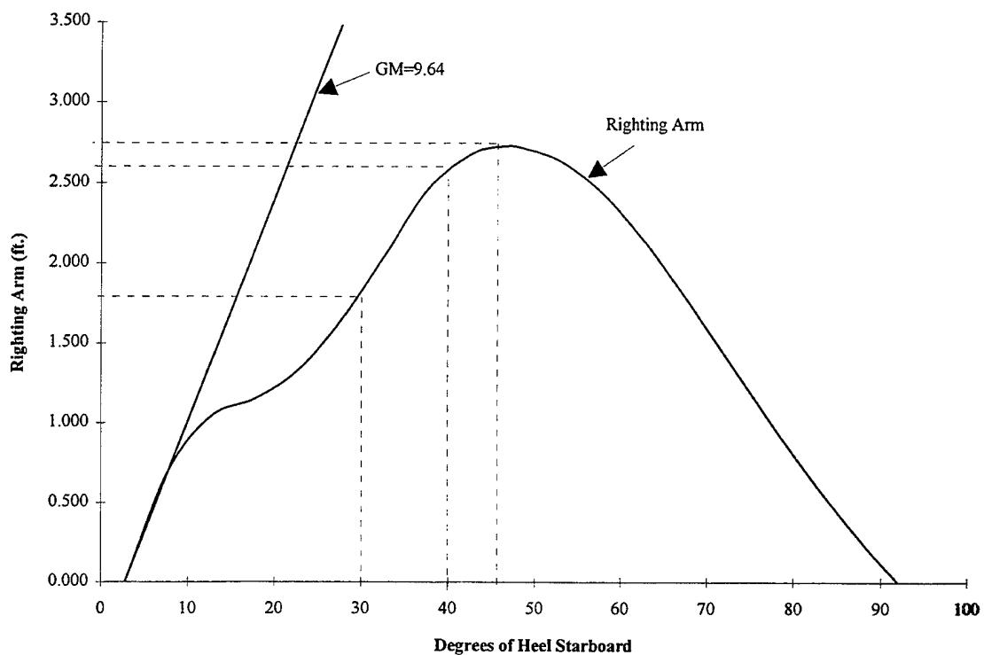
**Figure 24. Case 9, Righting Arm and GM Curve.**
