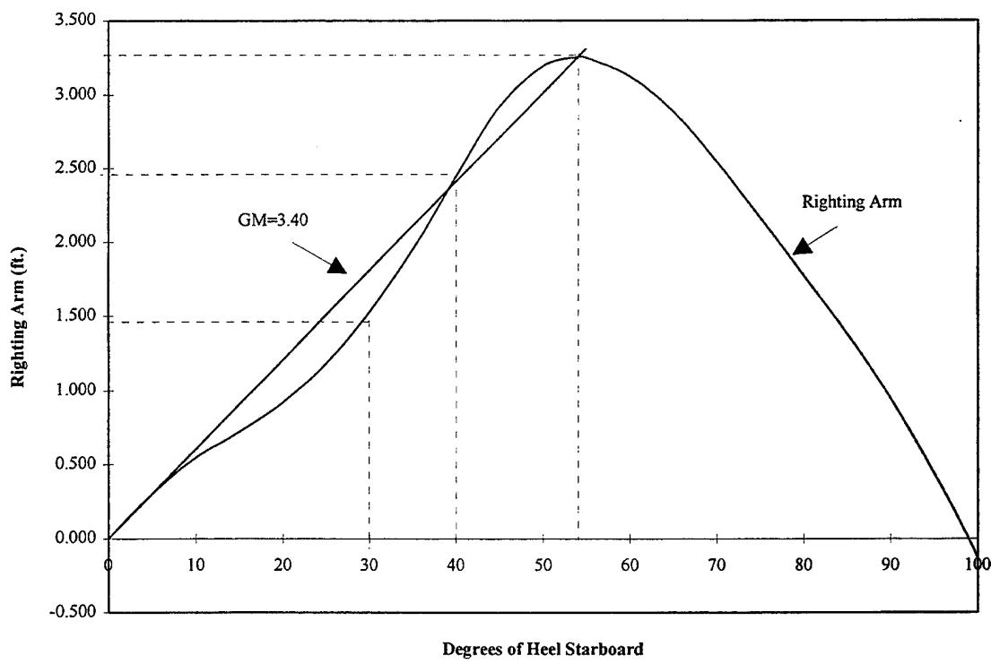
Figure 16. Case 4, Righting Arm and GM Curve.
