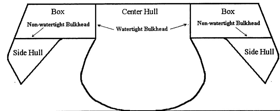
**Figure 8. Watertight Division Between Center and Side Hulls.**
