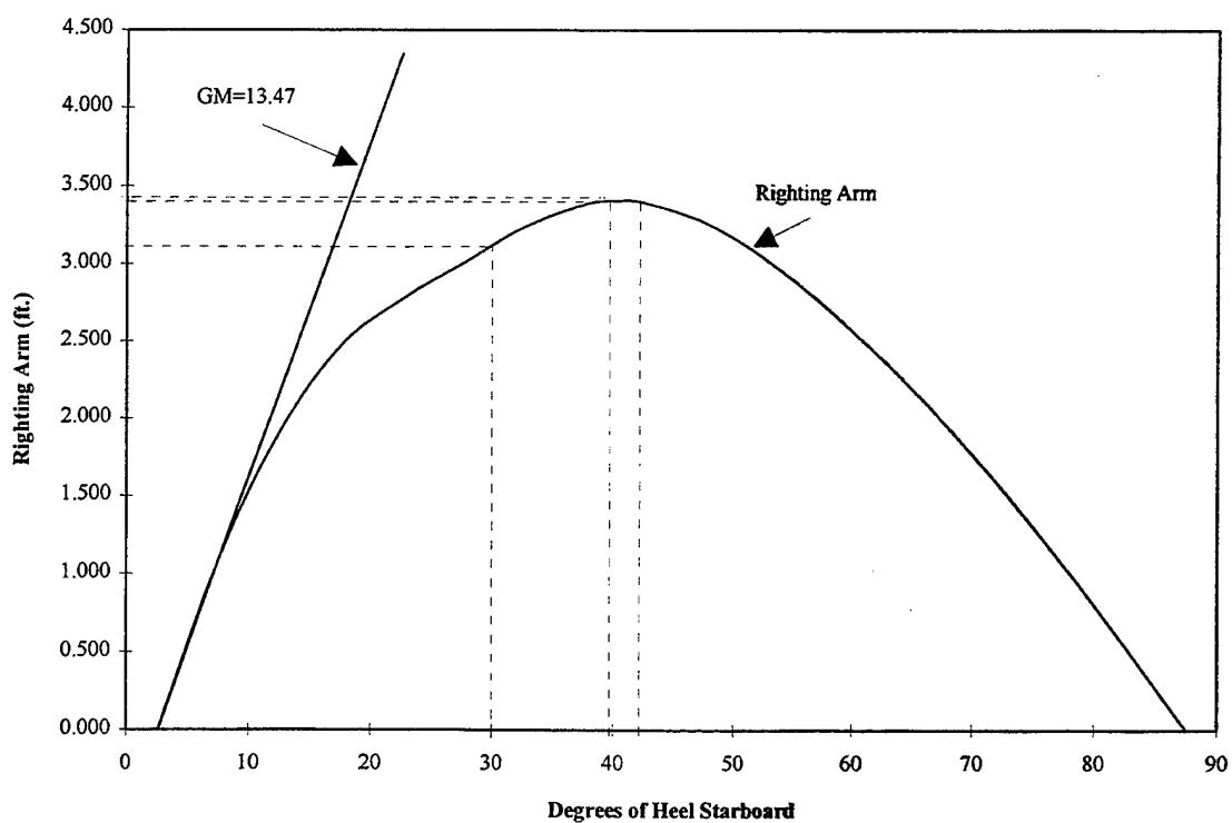
Figure 26. Case 10, Righting Arm and GM Curve.
