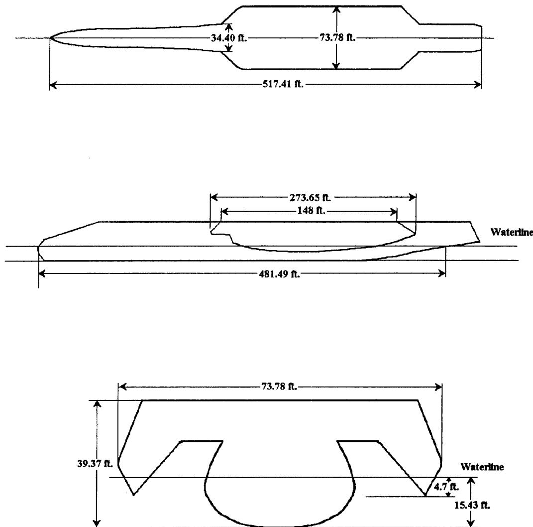
**Figure 1. Trimaran Model Characteristics.**
