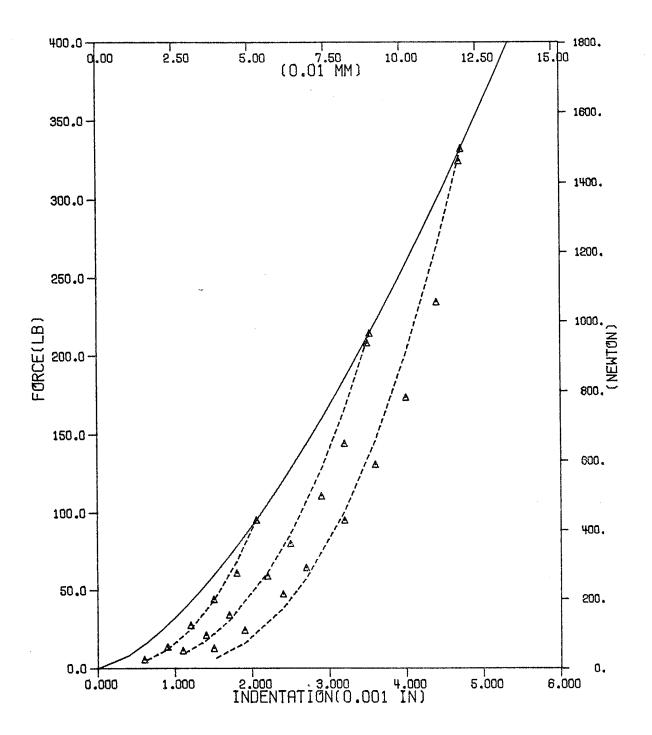
Fig. 15 - Unloading curves for graphite/epoxy with 50.8 mm(2")-span, 25.4 mm(1")-width, and 12.7 mm(0.5") indentor using  $\alpha_{\rm Cr}$  = 0.0803 mm (0.00316").
