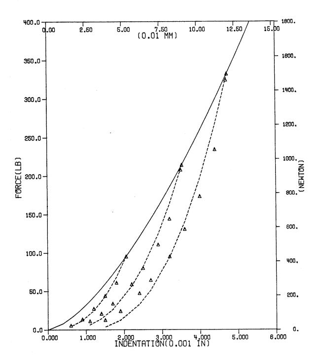
Fig. 13 - Unloading curves for graphite/epoxy with 50.8 mm(2")-span, 25.4 mm(1")-width, and 12.7 mm(0.5") indentor using area fit.
