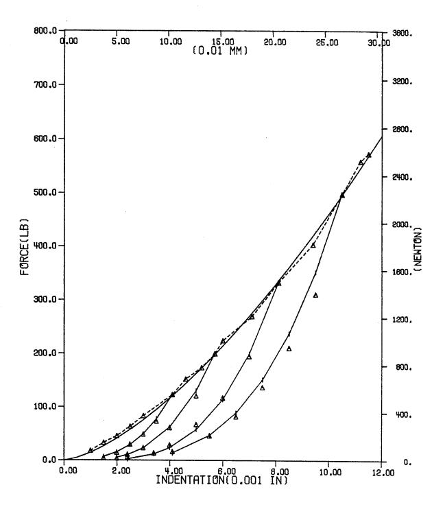
Fig. 9 - Unloading curves for glass/epoxy with q = 3.0, 50.8 mm(2")-span, and 6.35 mm(0.25") indentor.
