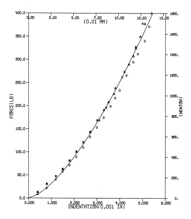
Fig. 6 - Least-square fit for loading with n = 1.5 for graphite/epoxy with 50.8 mm(2")-span, 25.4 mm(1")-width, and 12.7 mm(0.5") indentor.
