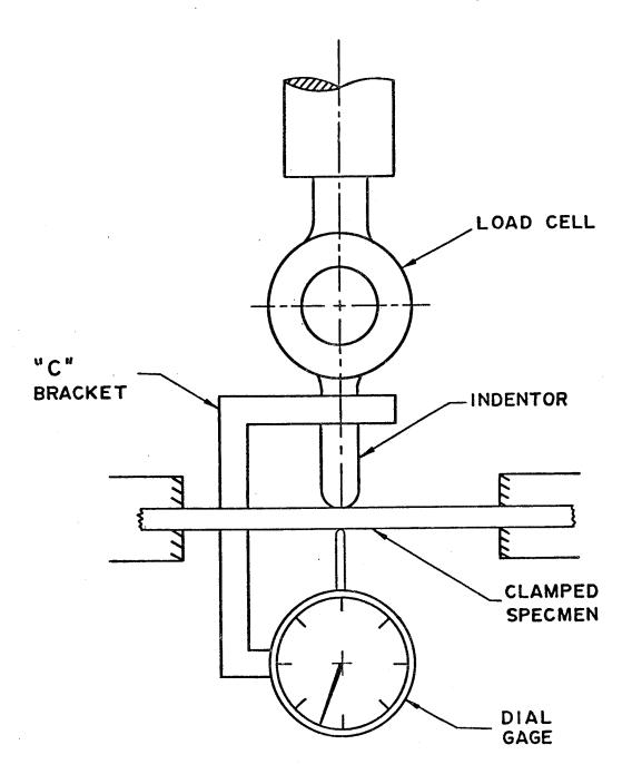
Fig. 1 Indentation test set-up
