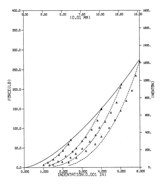
Fig. 14 - Unloading curves for graphite/epoxy with 50.8 mm(2")-span, 25. mm(1")-width, and 6.35 mm(0.25") indentor using  $\alpha_{cr}$  = 0.0803 mm(0.00316").
