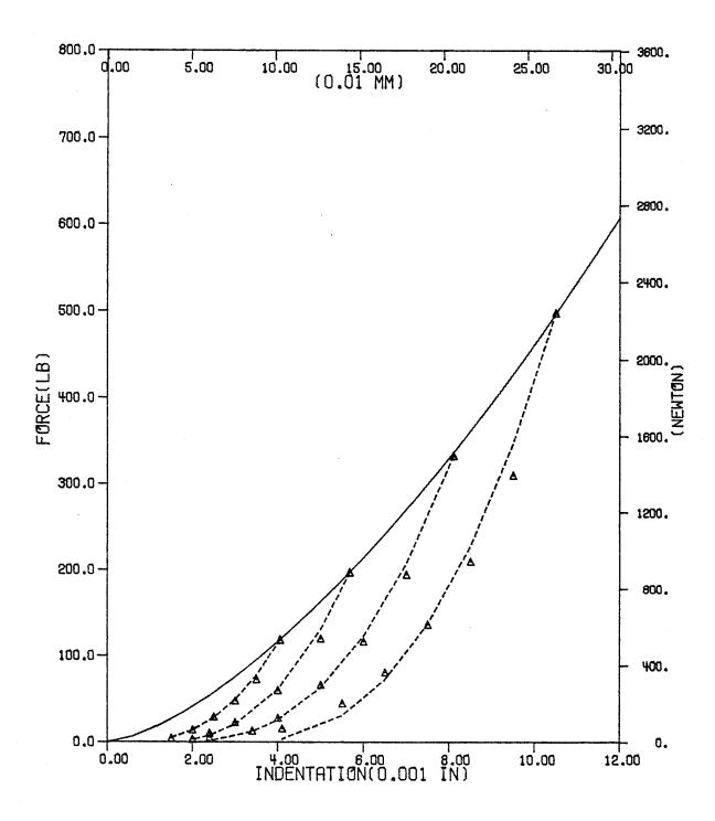
Fig. 10 - Unloading curves for glass/epoxy with 50.8 mm(2")-span and 6.35 mm(0.25) indentor using area fit.
