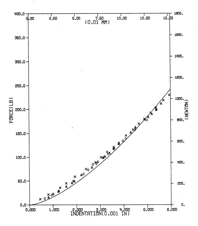
Fig. 5 - Least-square fit for loading with n = 1.5 for graphite/epoxy with 101.6 mm(4")-span, 25.4 mm-width, and 6.35 mm(0.25") indentor.
