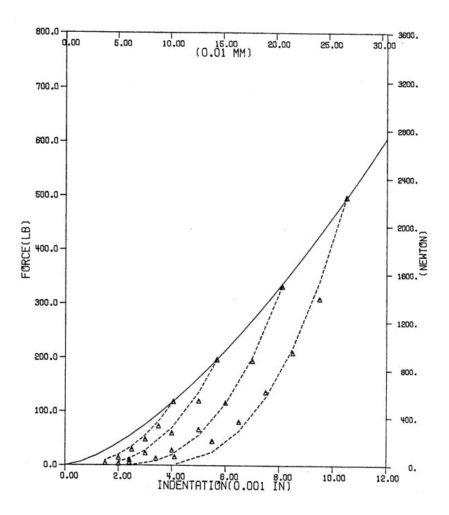
Fig. 11 - Unloading curves for glass/epoxy with 50.8 mm(2")-span and 6.35 mm(0.25") indentor using  $\alpha_{\rm cr}$  = 0.102 mm(0.004").
