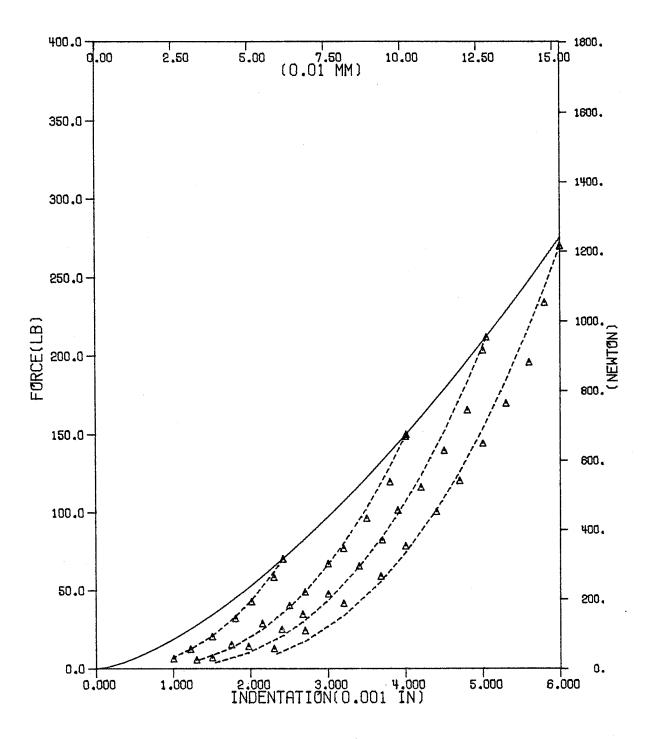
Fig. 12 - Unloading curves for graphite/epoxy with 50.8 mm(2")-span, 25.4 mm(1")-width and 6.35 mm(0.25") indentor using area fit.
