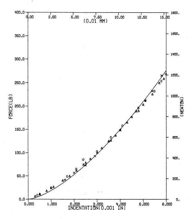
Fig. 4 - Least-square fit for loading with n = 1.5 for graphite/epoxy with 50.8 mm(2")-span 25.4 mm-width, and 6.35 mm (0.25") indentor.
