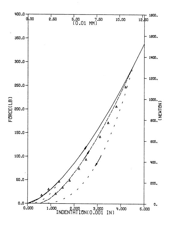
Fig. 17 - Reloading curves for graphite/epoxy with 101.6 mm(4")-span and 12.7 mm(0.5") indentor.
