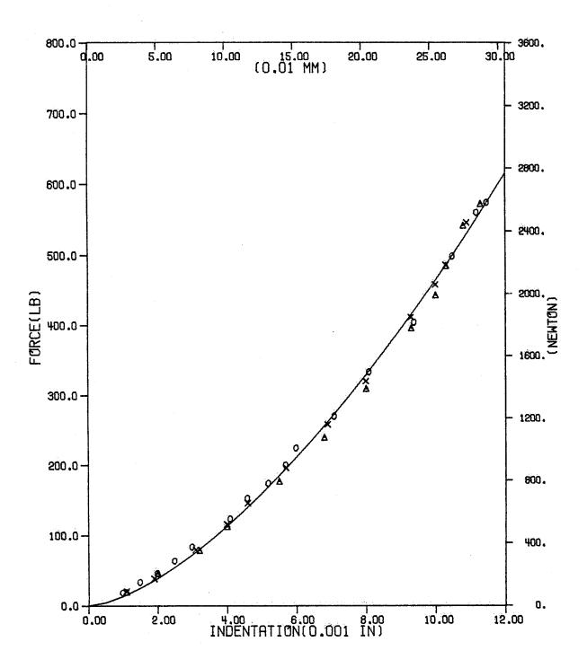
Fig. 2 - Least-square fit for loading for glass/epoxy with 50.8 mm(2")span and 6.35 mm (0.25") diameter indentor.
