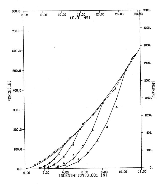
Fig. 8 - Unloading curves for glass/epoxy with q = 2.5, 50.8 mm(2")-span and 6.35 mm(0.25") indentor.
