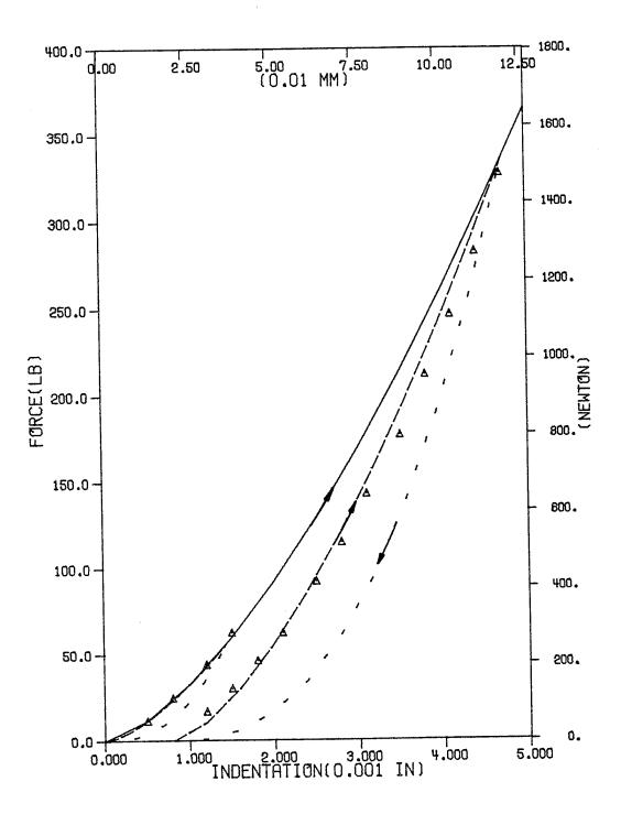
Fig. 16 - Reloading curves for graphite/epoxy with 50.8 mm(2")-span and 12.7 mm (0.5") indentor.
