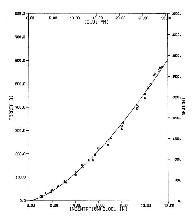
Fig. 3 - Least-square fit for loading with n = 1.5 for glass/epoxy with 50.8 mm(2")-span and 6.35 mm( $\overline{0.25}$ ") diameter indentor.
