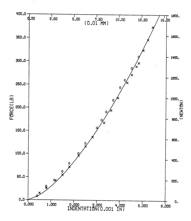
Fig. 7 - Least-square fit for loading with n = 1.5 for graphite/epoxy with 101.6 mm(4")-span, 25.4 mm(1")-width, and 12.7 mm(0.5") indentor.
