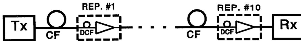
Fig. 1. Schematic diagram of system in computer simulations.
