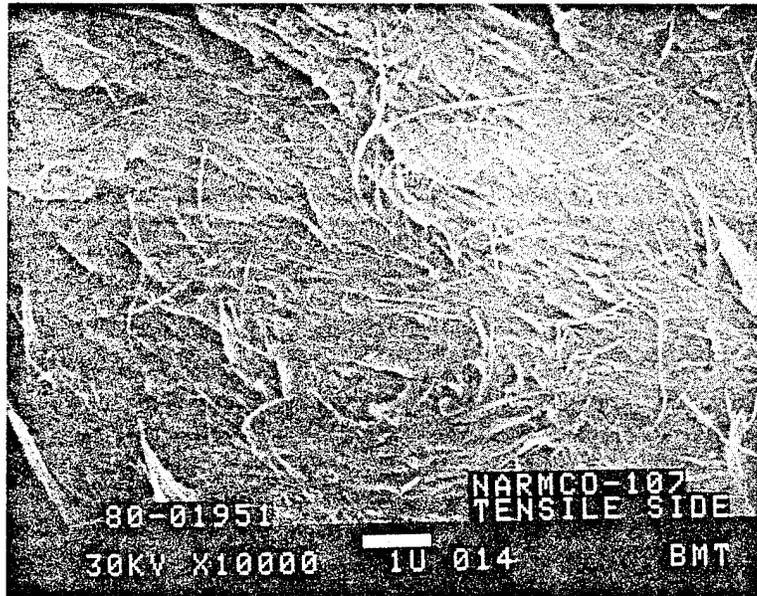
Figure 44. Hairy Appearance, Possible Elastomer Formation, Narmco 107 (10,000X)
