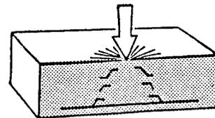
Figure 49. Compression Shear, Narmco 107 (500X)
