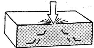
Figure 35. Compression Fracture, Air Logistics 1 (16X)
