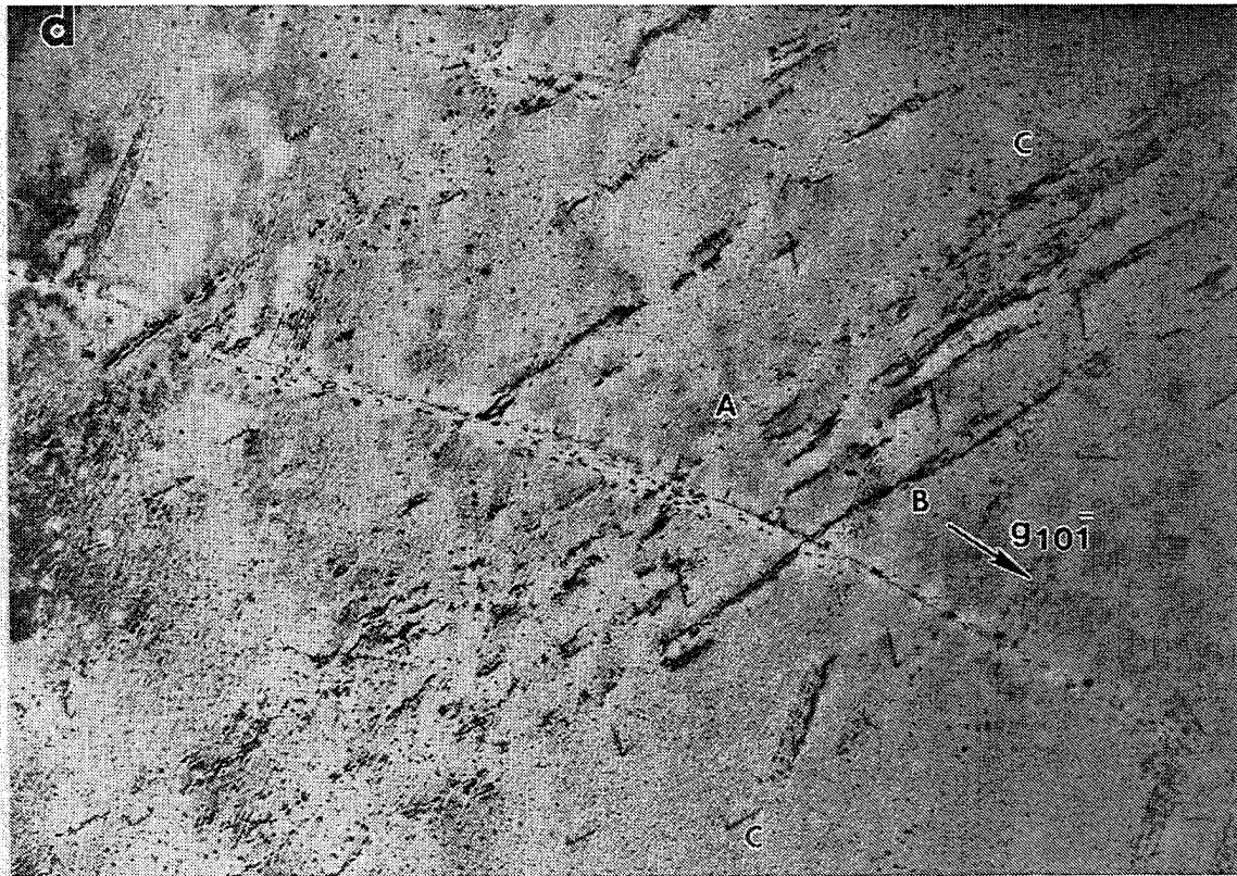
Figure 83(cont.). Dislocation structure and g \cdot b analysis for NiAl alloy D176 deformed along [001] at room temperature. a) general area of analysis, b) g110 , c) g011 close to the Z.A. [011] , d) g101 , e) g110 , and f) g011 close to the Z.A. [011] .
