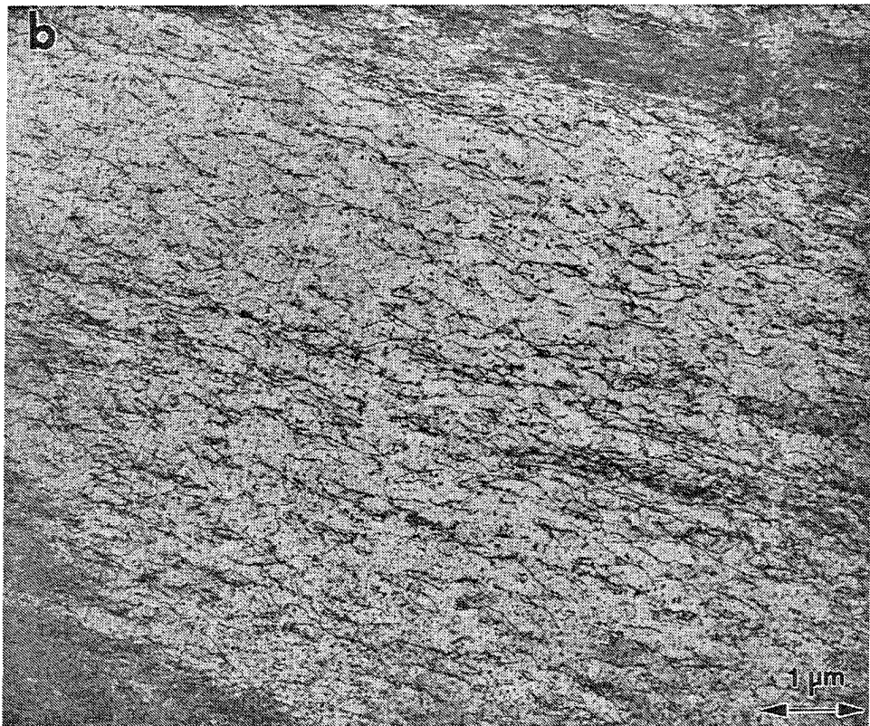
Figure 92. Dislocation structure in [011] D176 sample deformed at a) 1000 K and b) 1144 K. Both samples were deformed to approximately 2% plastic strain toward the end of region I.
