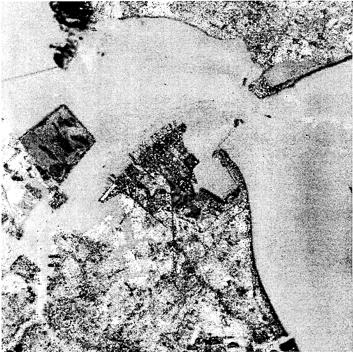
Figure 33: Second principal component image of Norfolk, Virginia. Input for principal component analysis was four radar bands and three visible color bands
