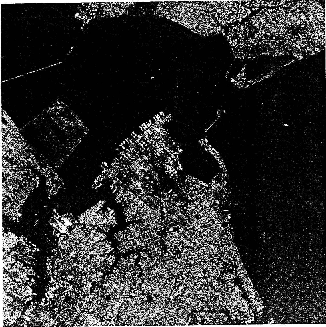
Figure 42: Third principal component image of Norfolk, Virginia. Input for principal component analysis was four radar bands.
