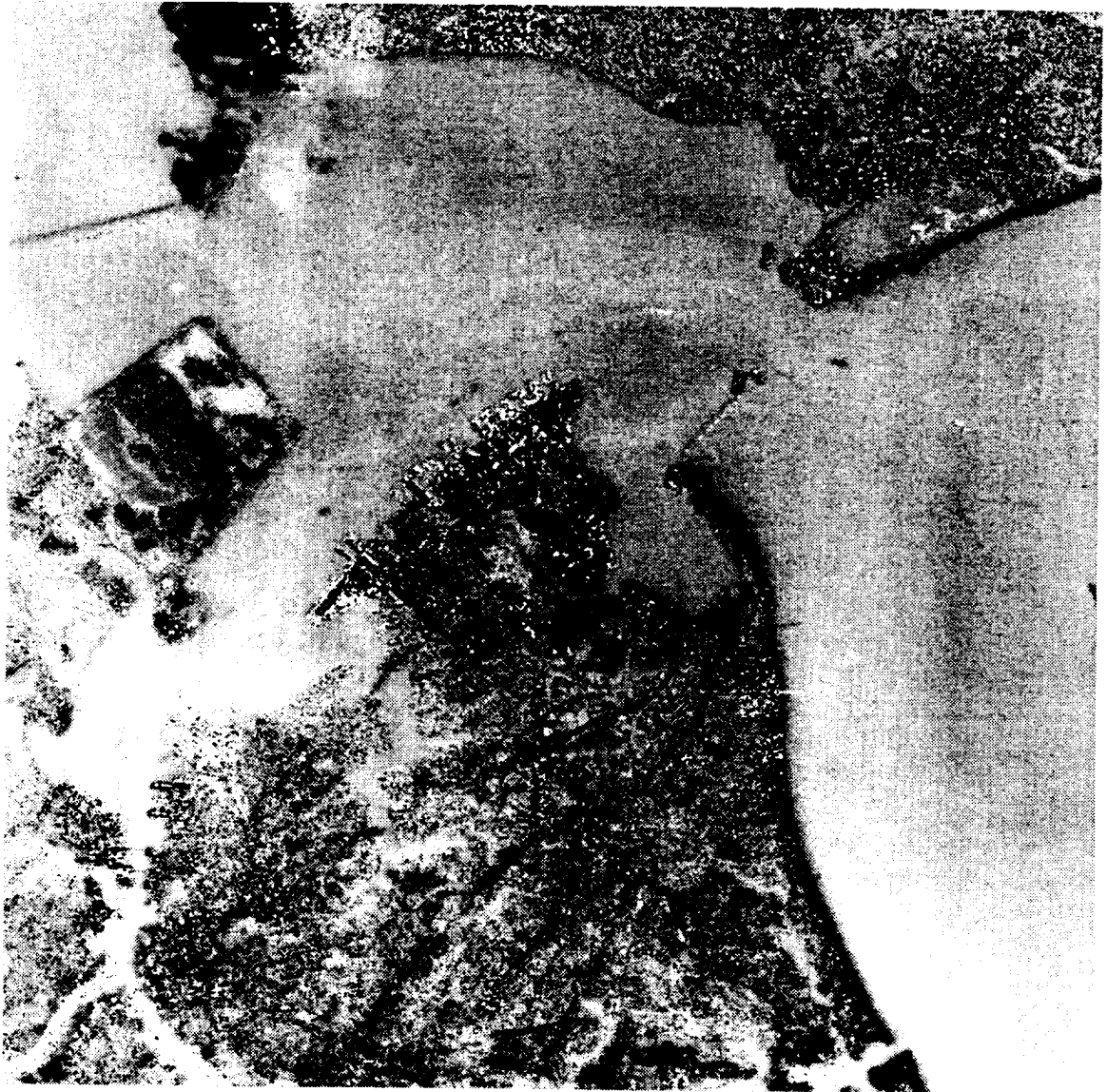
Figure 34: Third principal component image of Norfolk, Virginia. Input for principal component analysis was four radar bands and three visible color bands
