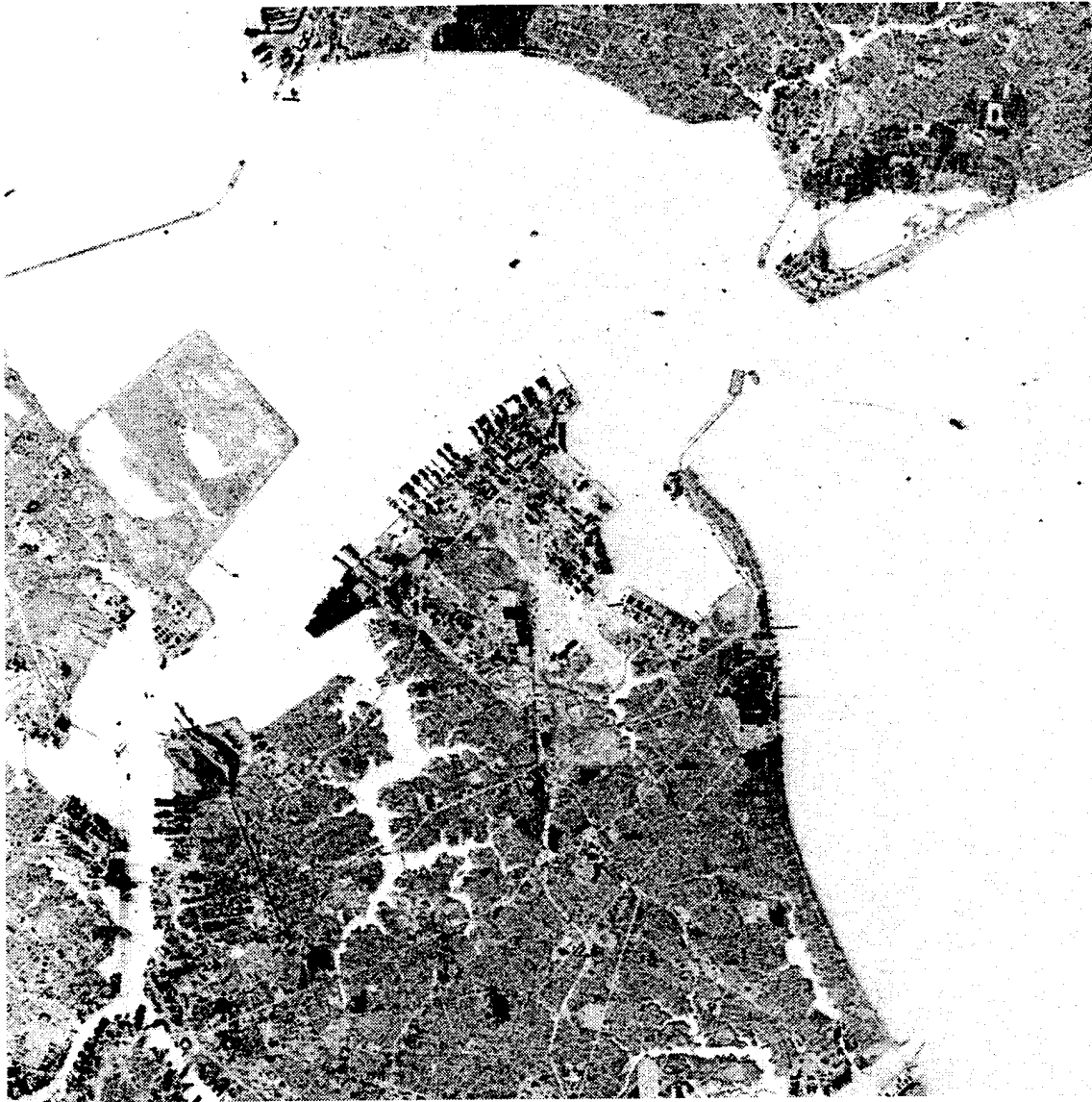
Figure 32: First principal component image of Norfolk, Virginia. Input for principal component analysis was four radar bands and three visible color bands
