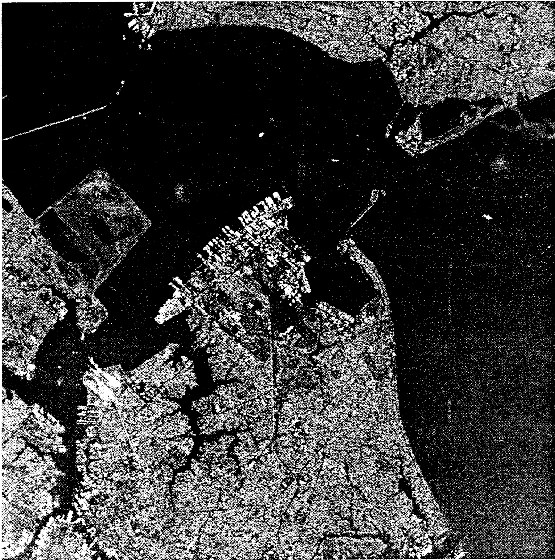
Figure 15: C-band HV polarization image of Norfolk, Virginia. Taken by the SIR-C Synthetic Aperture Radar on Space Shuttle mission STS-68 in October of 1994
