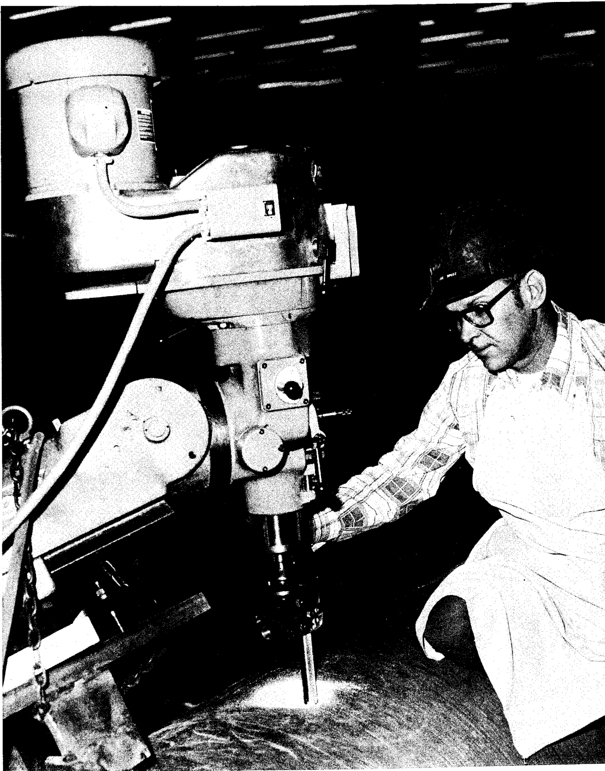
Figure 67. Machining Holes in Composite Spar for Hub Adapter Bolts.
