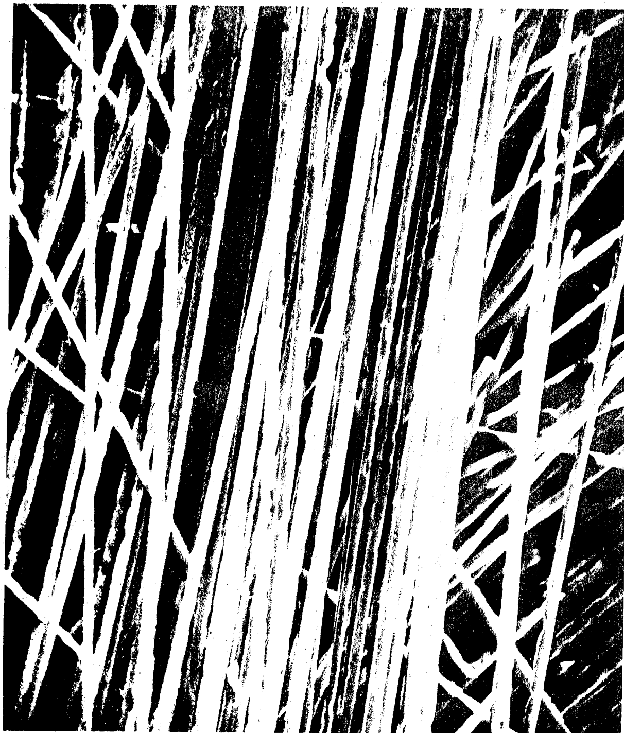
Fig. 5 SEM micrograph of carbon fibers [Thornel 300 (Union Carbide)] after exposure for 3.5 minutes at 1000°C.
