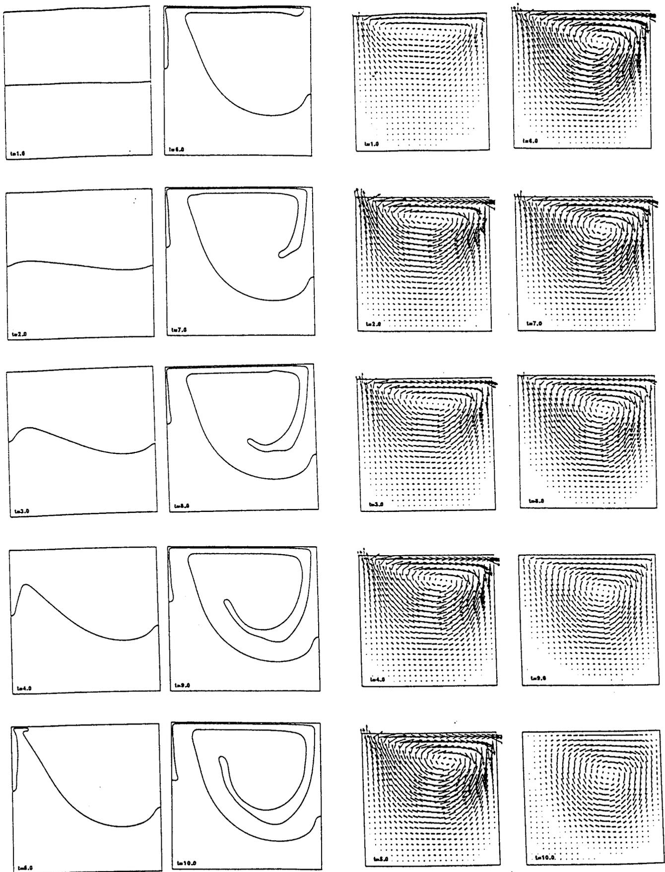
Figure 6. Interface location and velocity field for the driven cavity,  $Re=100$ , no-slip boundary conditions,  $\rho_f=0.9$ ,  $\mu_f=1.0$  and grid size of  $100 \times 100$ .
