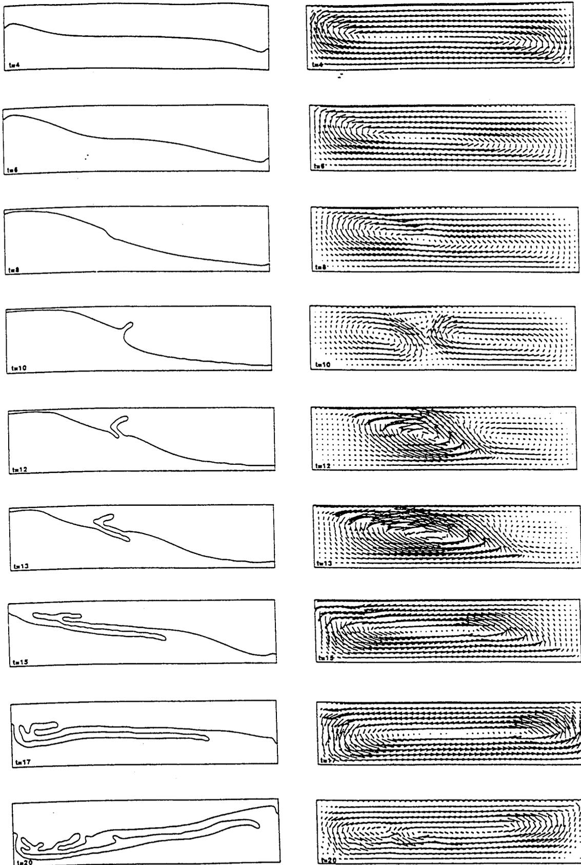
Figure 11. Interface location and velocity field for a rotating box,  $Re=100$ ,  $\theta_{rot}=30*\sin(0.315*t)$ ,  $\rho_f=0.5$  and  $\mu_f=0.2$ .
