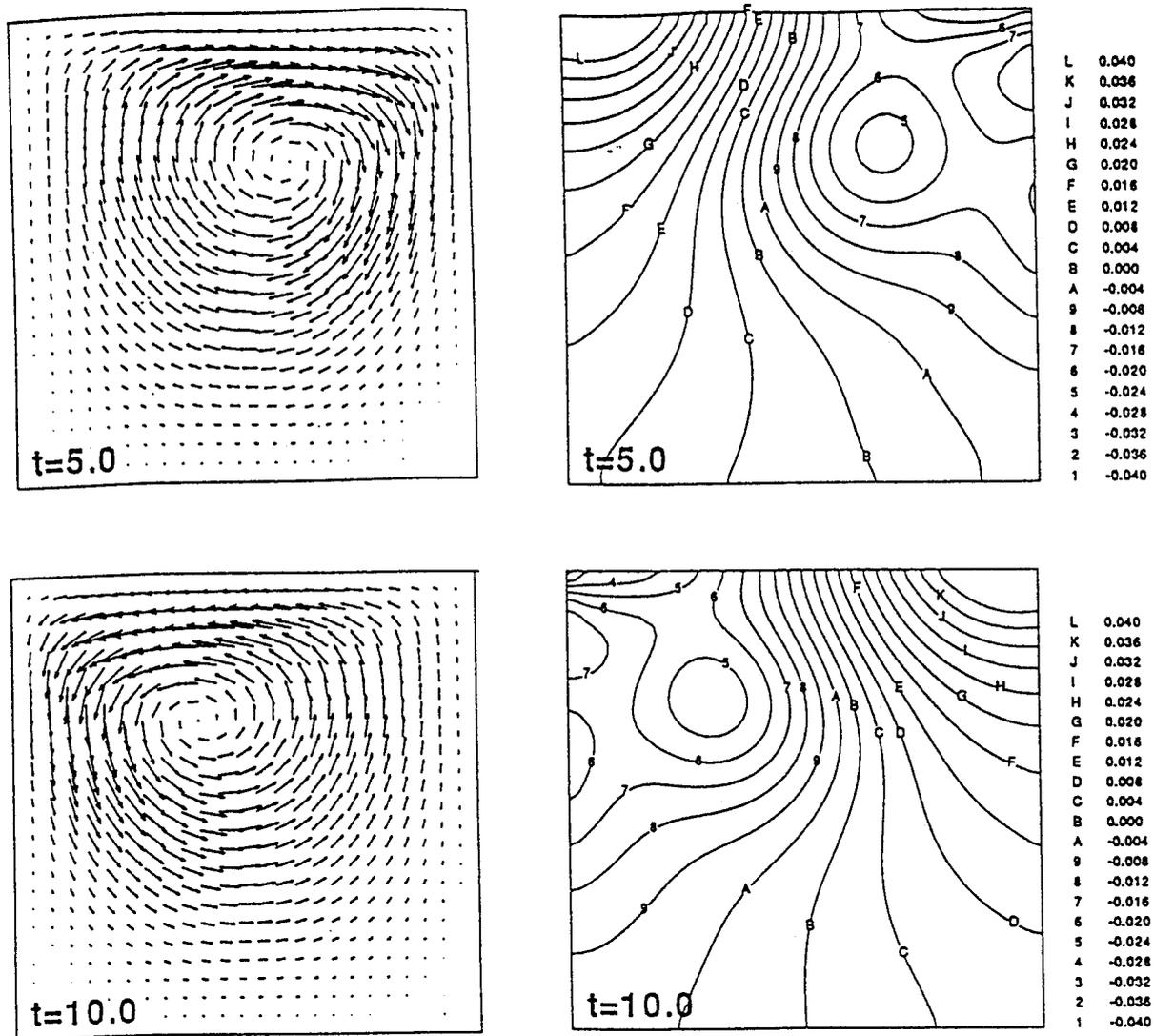
Figure 3. Velocity and pressure fields at  $t=5$  and  $t=10$  for a driven cavity,  $Re=100$ , no-slip boundary conditions and constant fluid properties.
