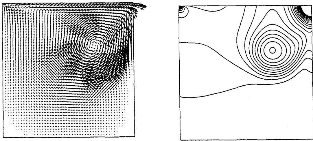
Figure 2. Velocity and pressure fields at  $t=4.9$  for a driven cavity,  $Re=1000$ , no-slip boundary conditions and constant fluid properties.
