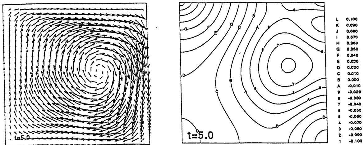
Figure 4. Velocity and pressure fields at  $t=5$  for a driven cavity,  $Re=100$ , slip boundary conditions and constant fluid properties.
