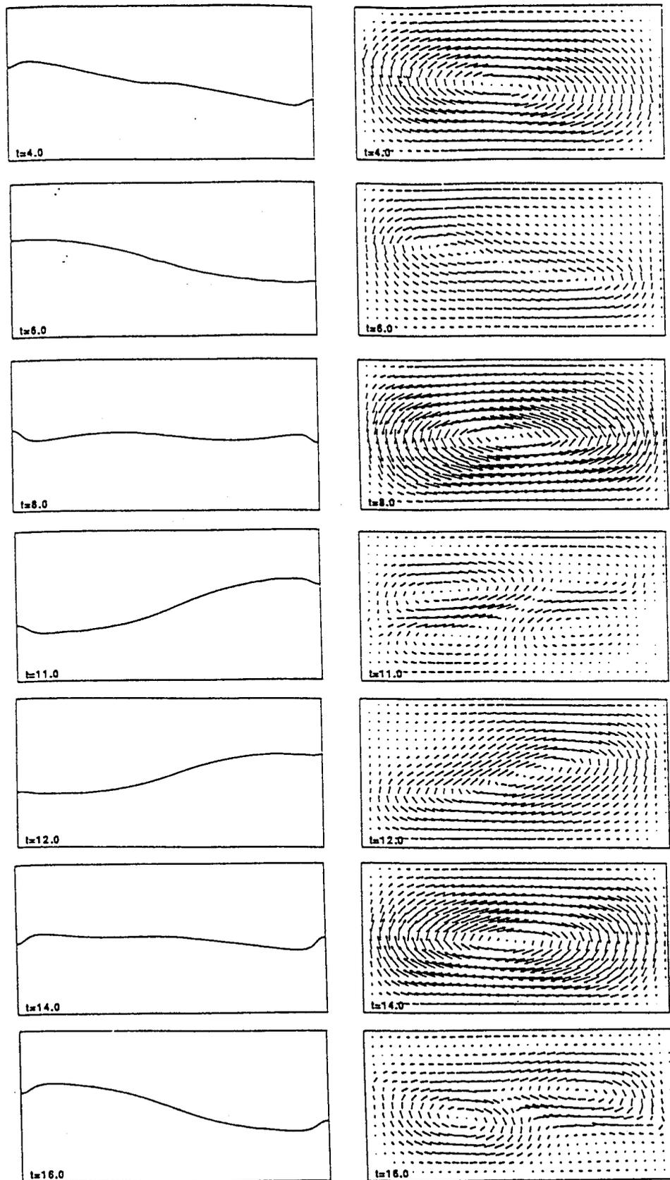
Figure 10. Interface location and velocity field for a translating box,  $Re=100$ ,  $u_0=0.25$ ,  $\rho_f=0.5$  and  $\mu_f=0.2$ .
