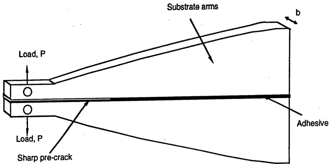
Figure 3.1 A sketch of the tapered-double cantilever-beam (TDCB) adhesively-bonded joint.
