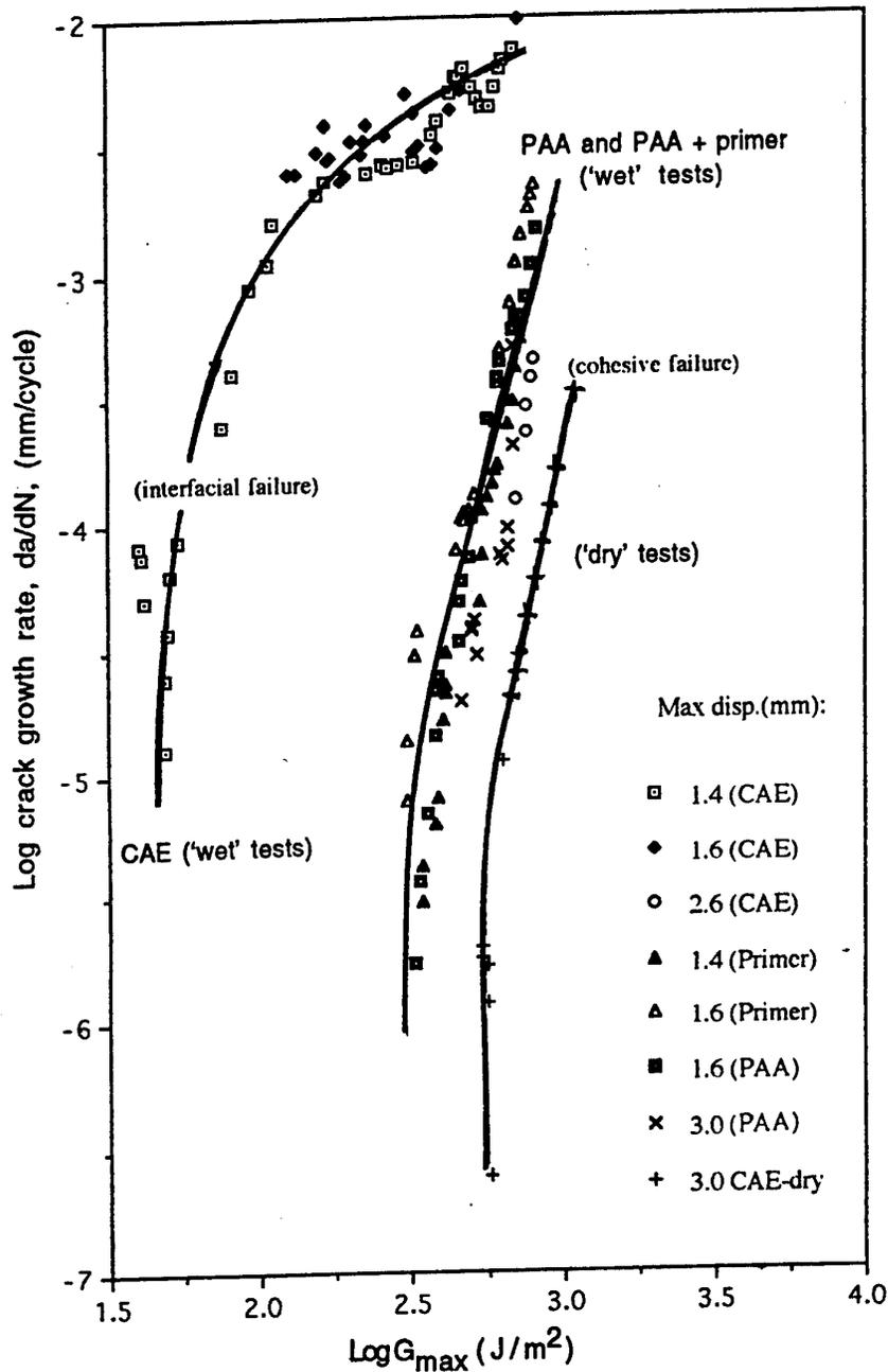
Figure 3.3 Logarithmic crack growth rate per cycle,  $da/dN$ , versus logarithmic  $G_{max}$  for all the different types of joints tested in both the 'dry' and 'wet' environments. The main type of joint and test environment associated with a given set of data are stated. (TDCB joint tests.)
