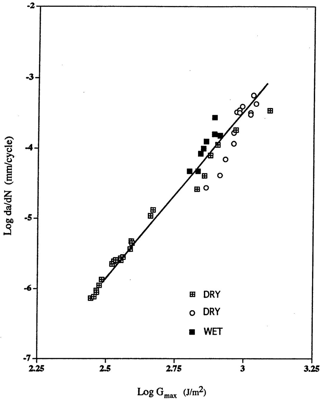
Figure 2.3 Log crack growth rate per cycle,  $da/dN$ , versus  $\text{log } G_{\text{max}}$  for the joints prepared using carbon-fibre/ PEEK substrates (corona treated) bonded with the epoxy film adhesive in the 'dry' and 'wet' environments. (DCB joints)
