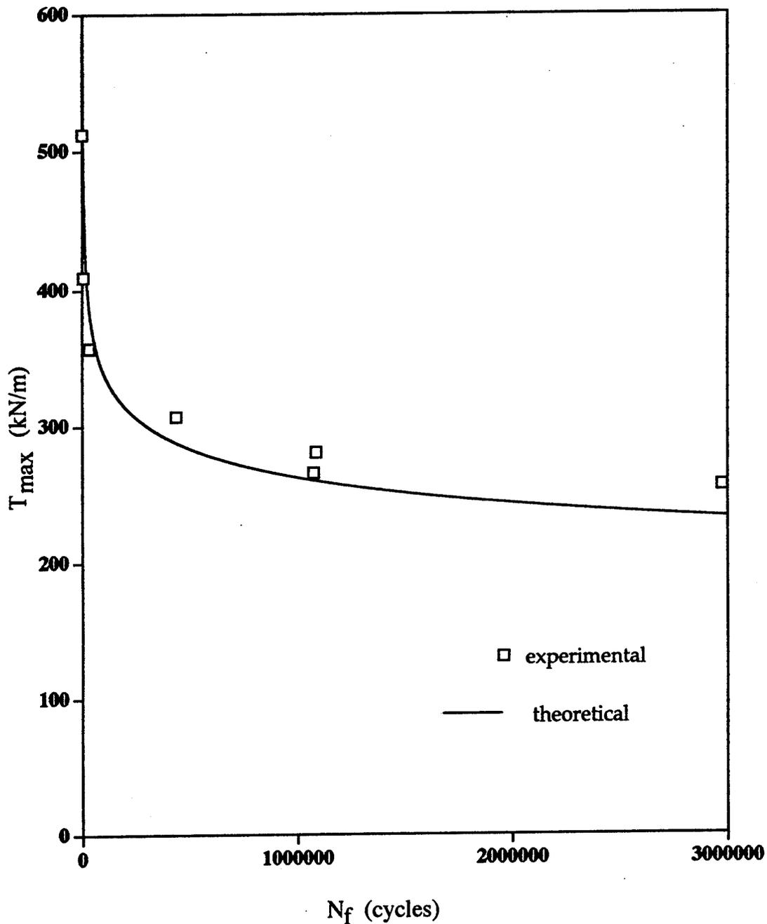
Figure 2.5 A comparison of the theoretical and experimental values for the maximum load per unit width,  $T_{max}$  applied in a fatigue cycle versus the number,  $N_f$ , of cycles to failure for the carbon-fibre/PEEK substrates (corona treated) bonded using the epoxy film adhesive. (Single lap joints)
