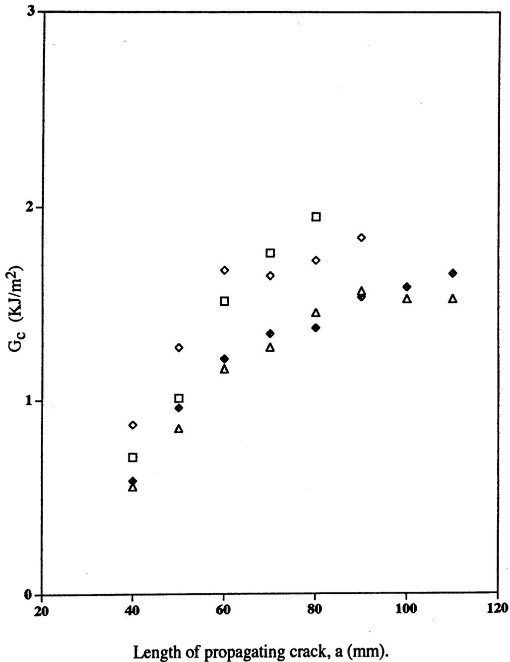
Figure 2.7 The adhesive fracture energy,  $G_c$ , versus the length,  $a$ , of the propagating crack for the joints consisting of the glass-fibre/PPS substrates (abrasion/solvent wipe treated) bonded using the epoxy film adhesive. (DCB tests.)
