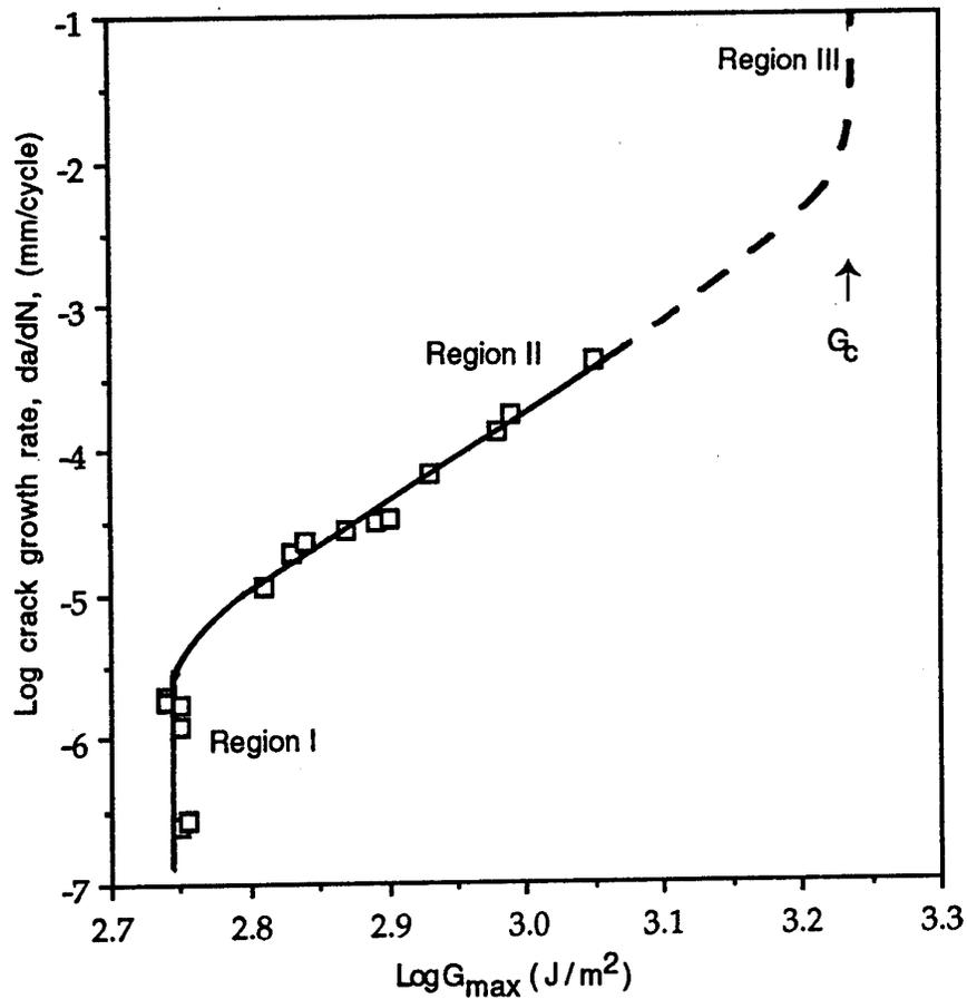
Figure 3.2 Logarithmic crack growth rate per cycle,  $da/dN$ , versus logarithmic  $G_{\text{max}}$  for the joints prepared using the CAE pretreatment for the aluminium-alloy substrates and bonded using the epoxy-film adhesive. The fatigue tests were conducted in the 'dry' environment of  $23^{\circ}\text{C}$  and 55% r.h. (TDCB joint tests.)
