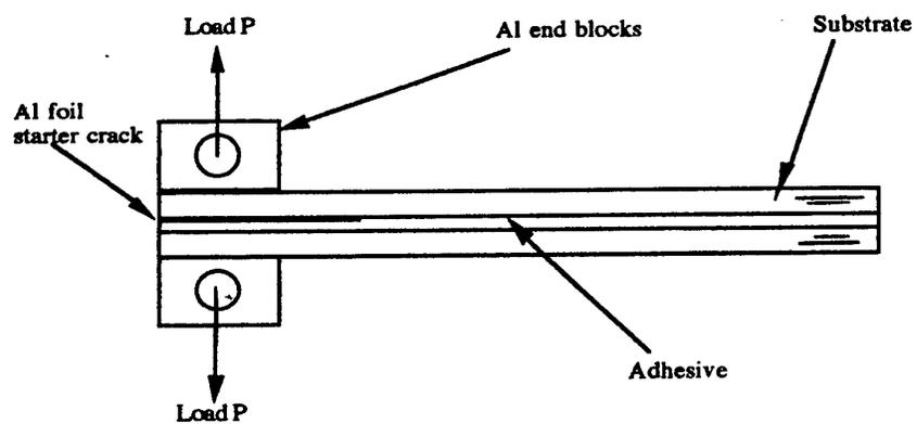
Figure 2.1 A schematic representation of the DCB joint.
