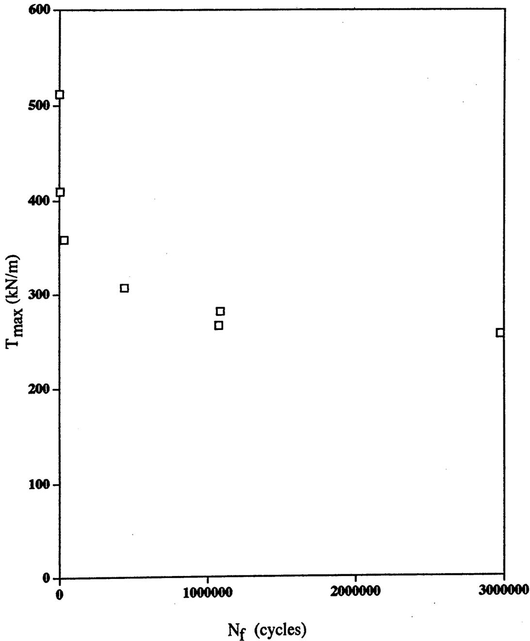
Figure 2.4 Experimental values for the maximum load per unit width,  $T_{max}$  applied in a fatigue cycle versus the number,  $N_f$ , of cycles to failure for the carbon-fibre/PEEK substrates (corona treated) bonded using the epoxy-film adhesive. (SLJ tests)
