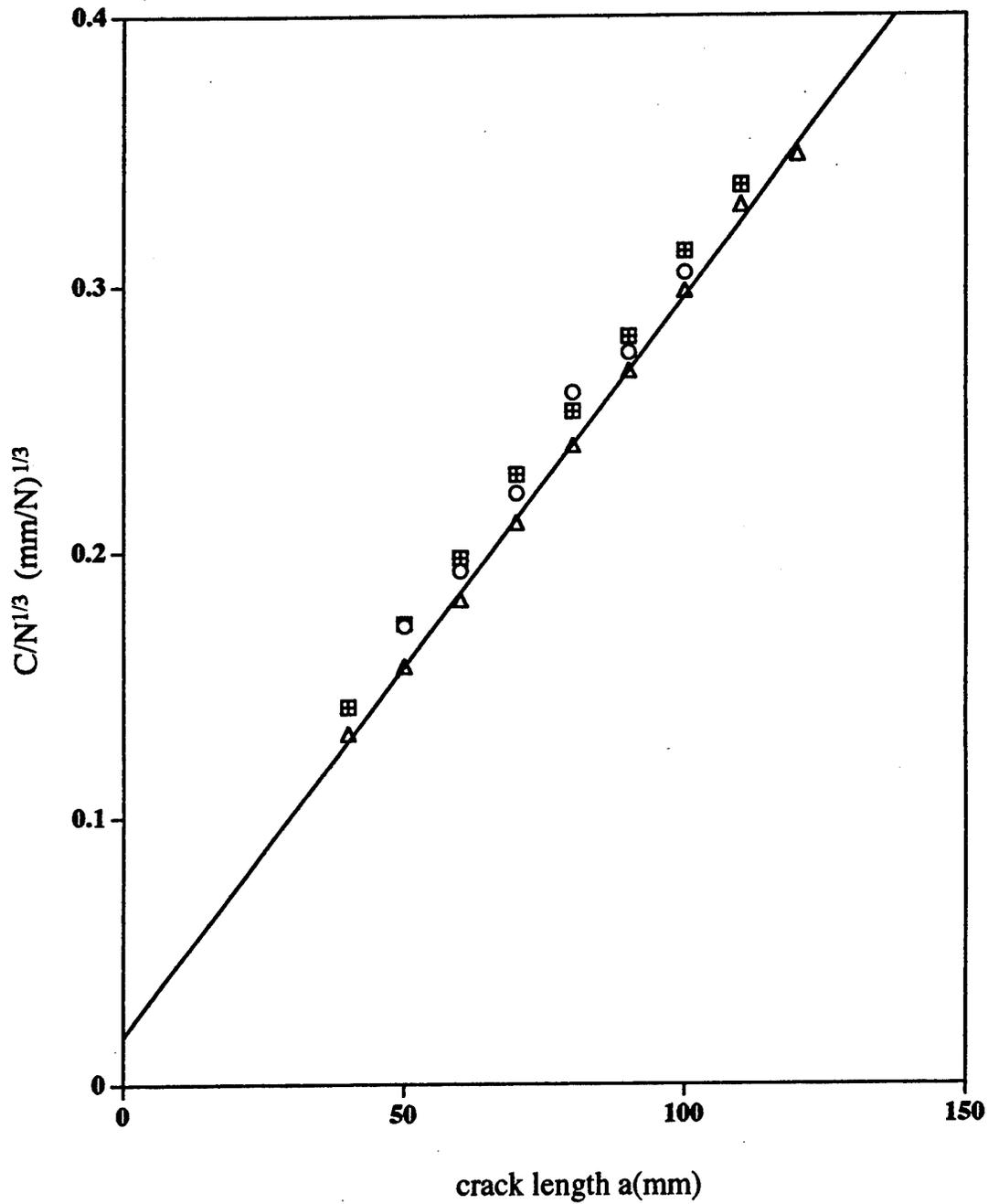
Figure 2.2  $(C/N)^{1/3}$  versus crack length,  $a$  for a DCB adhesive joint consisting of glass-fibre/PPS substrates bonded using the epoxy-film adhesive.
