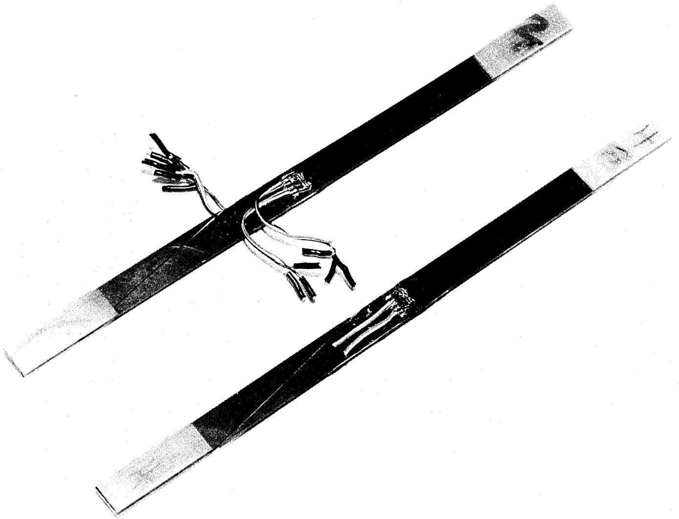
FIGURE 41 STRAIN GAGED INTRALAMINAR SHEAR STRENGTH SPECIMENS SHOWING TYPICAL FAILURE MODE
