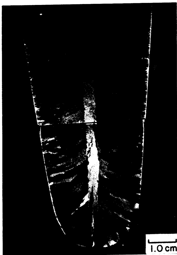
Fig. 2(a). 9 volume percent \delta , columnar \gamma crystals. Light micrograph, deposition color etch.
