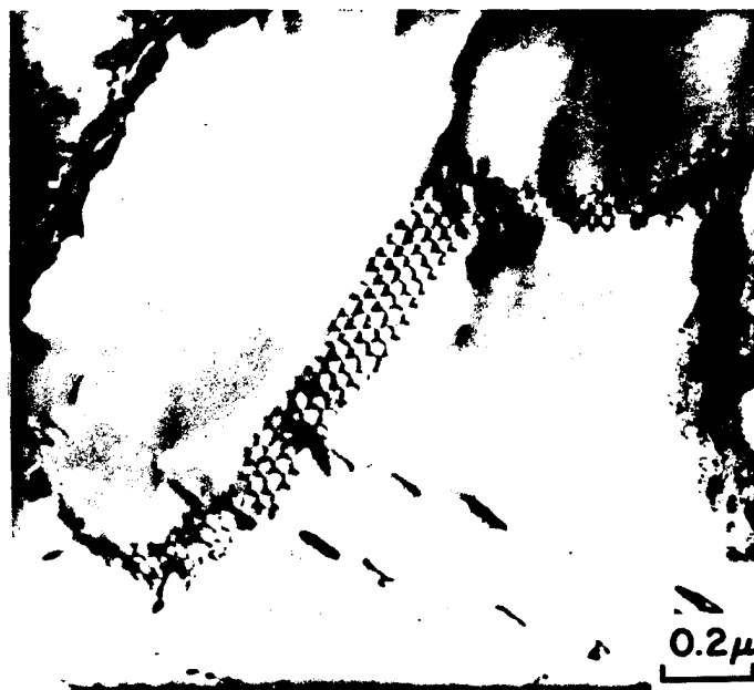
Figure 9(a) Nets of dislocations in subgrain boundaries, 1.1% \delta ; TEM (a) BF
