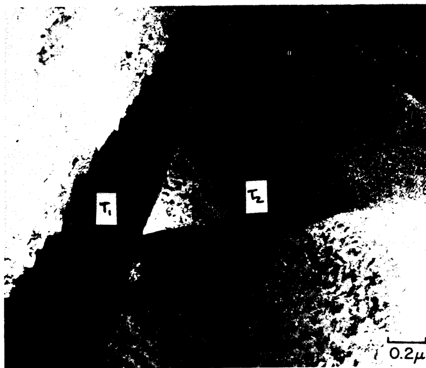
(c). Dark-field employing \delta matrix reflection.
