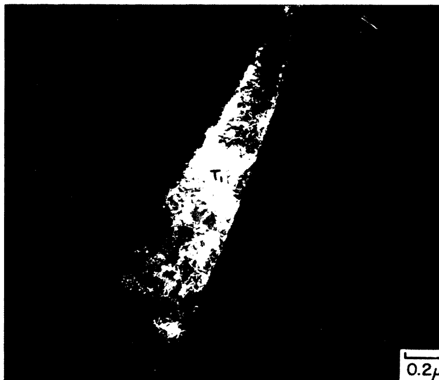
Fig. 28(b). Dark-field of T_1 employing twin reflection.
