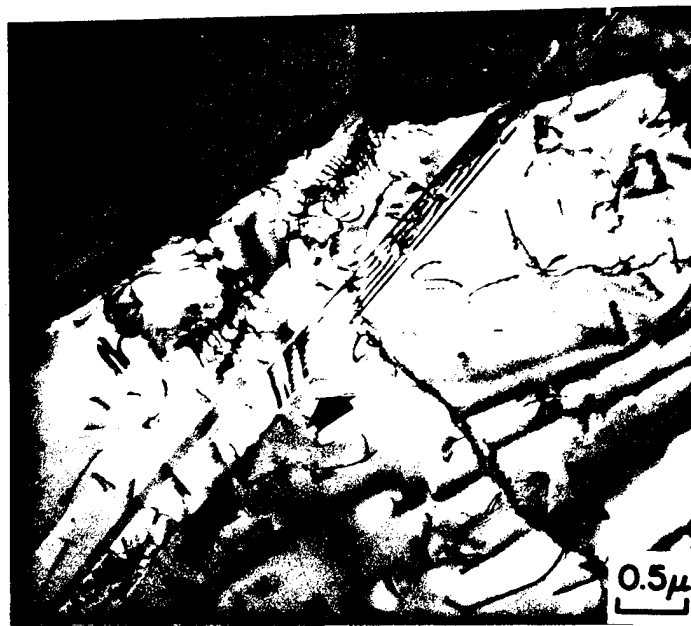
Figure 12(a) Faulting in \gamma ; TEM (a) Overlapping stacking faults
