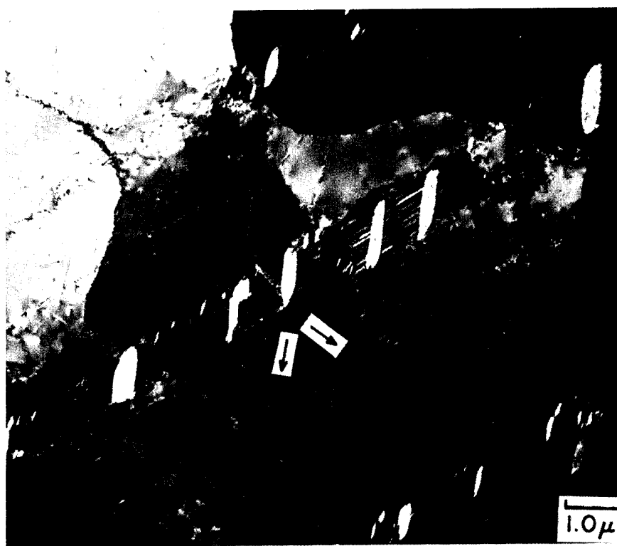
Fig. 21(b). Dark-field employing \alpha' reflection.
