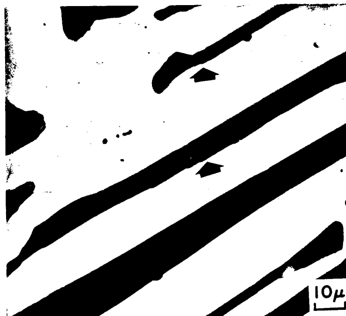
Figure 7 Residual \delta showing ledges on \delta/\gamma interface.
