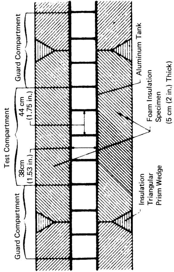
Figure 25. Cryogenic Insulation Configuration (Joint Wedges not Shown) — Dimensions are in Centimeters
