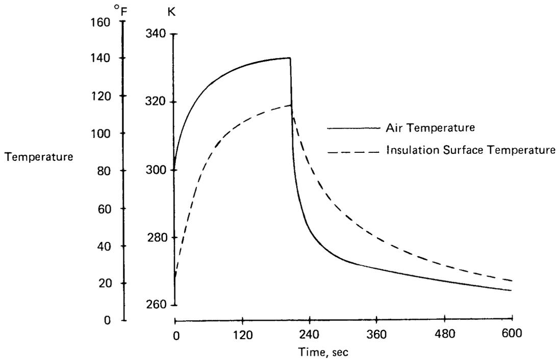
Figure 7. Air and Insulation Surface Temperature Histories for a Typical Test Cycle with Tank Wall at LH<sub>2</sub> Temperature
