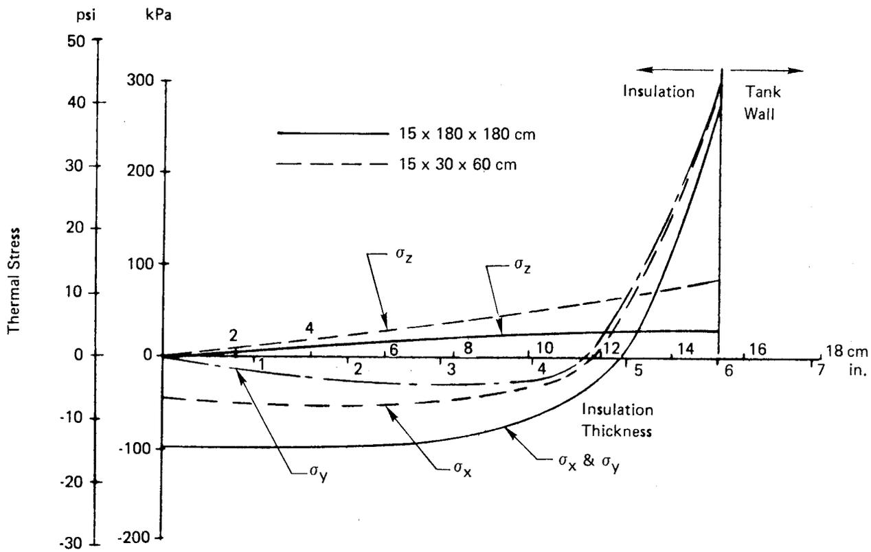
Figure 20. Thermal Stresses for Two Different Sample Sizes of Insulation, Rohacell 51
