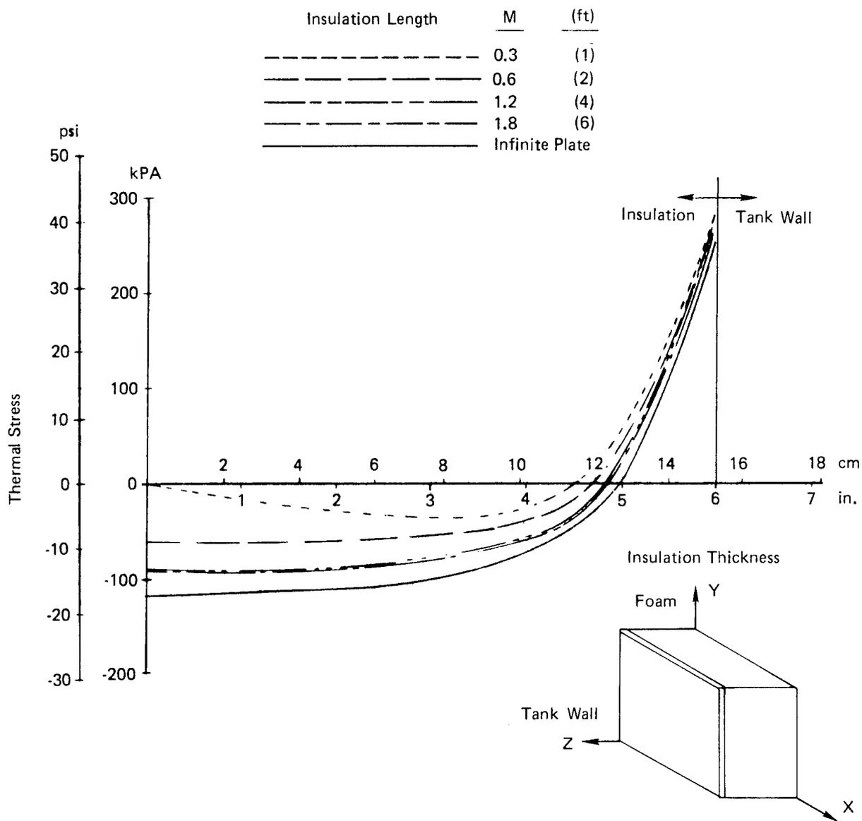
Figure 18. Maximum Inplane Thermal Stress Through the Insulation Thickness on a LH<sub>2</sub> Tank For Various Insulation Lengths and an Insulation Width of 60 cm (2 ft), Rohacell 51
