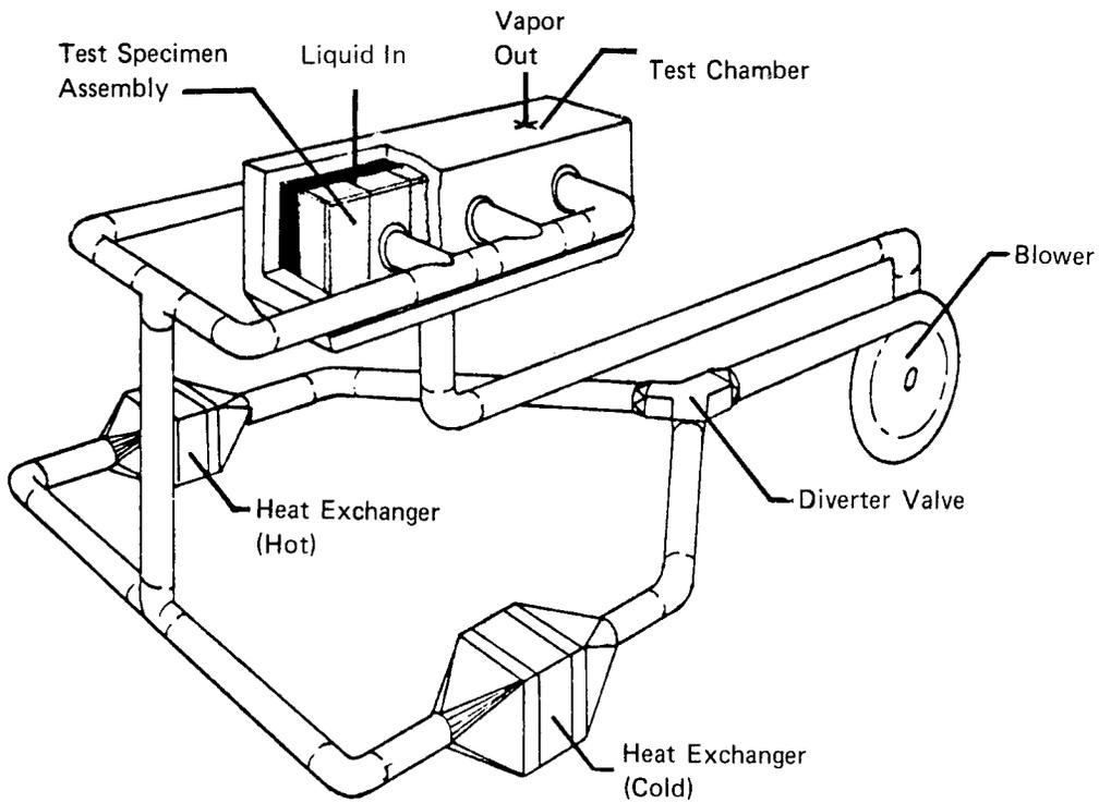
Figure 4. Cryogenic Insulation Test Apparatus-Environmental Control System.
