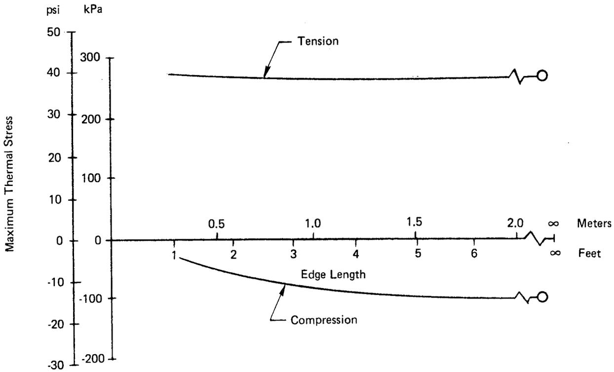
Figure 2. Maximum In-Plane Tensile and Compressive Thermal Stresses for Square, 15 cm (6 in.) Thick Foam Insulation Bonded to Aluminum at LH<sub>2</sub> Temperature.
