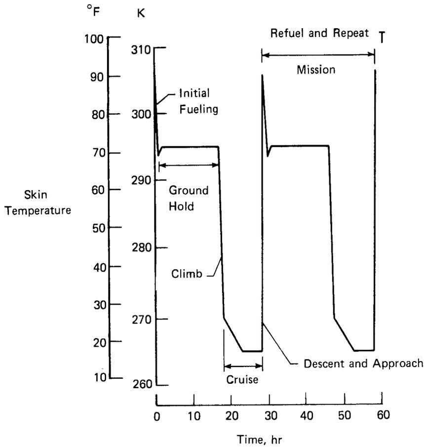
Figure 6. Cryogenic Insulation Surface Temperature for Typical LH<sub>2</sub> Fueled Subsonic Transport Mission Cycles 10, 180 km (5500 nm) Range, 152 mm (6 in.) Thick Insulation (Ref. 2)
