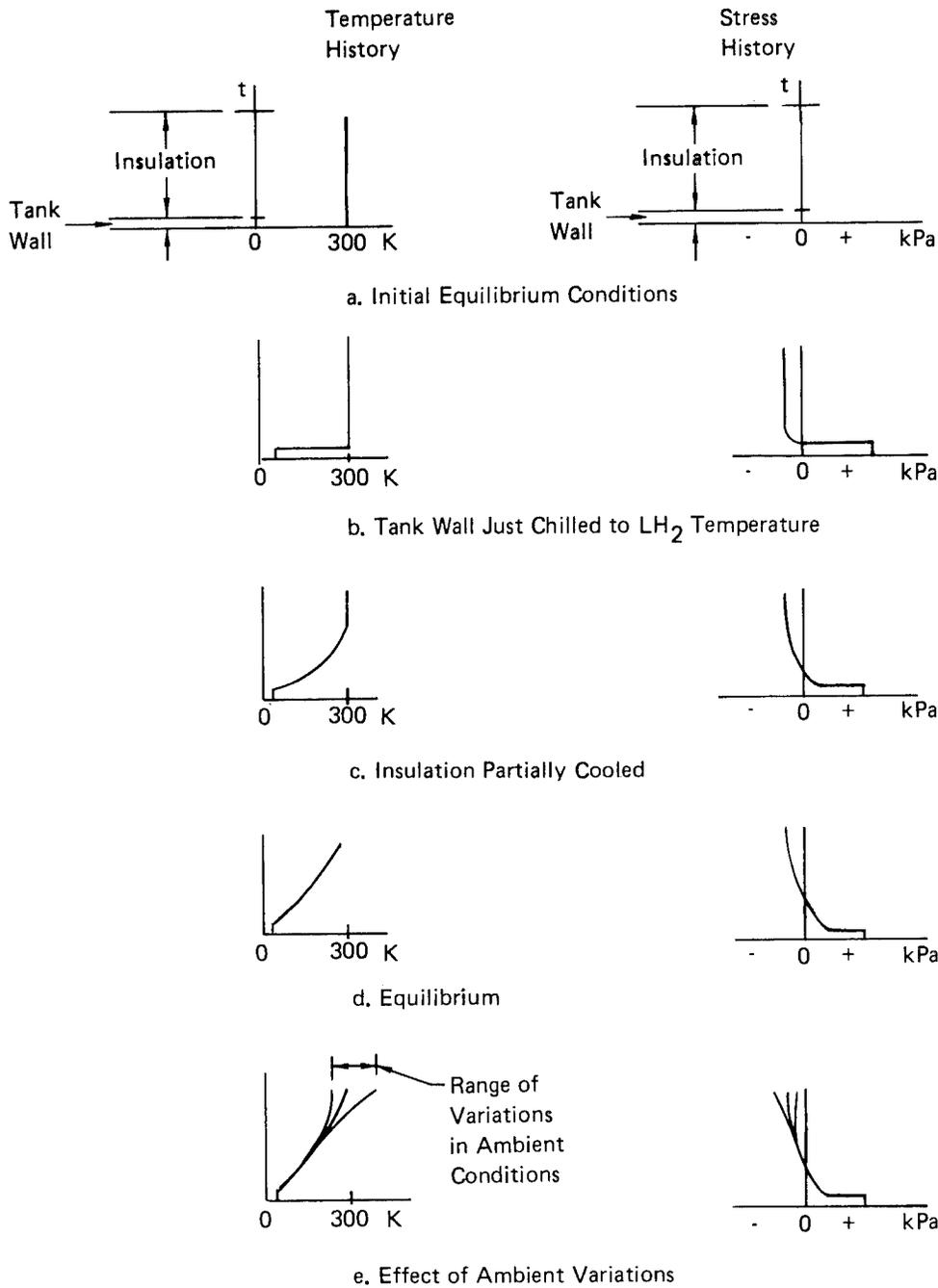
Figure 14. Temperature and Stress Histories During Cooldown and Operation of Insulated LH<sub>2</sub> Tank
