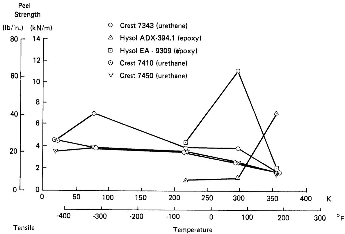
Figure 11. Peel Strength versus Temperature for Candidate Adhesives
