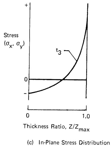
Figure 1. Conditions Found in Insulation Bonded to Aluminum Plate at LH<sub>2</sub> Temperature.
