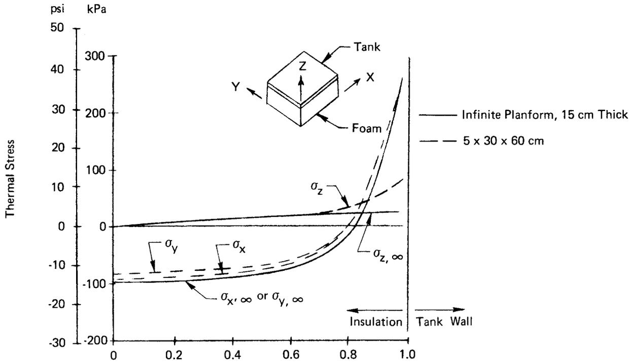
Figure 3. Comparison of Three Dimensional Thermal Stresses in Insulation Foam Bonded to an Aluminum Tank Wall at LH<sub>2</sub> Temperature.
