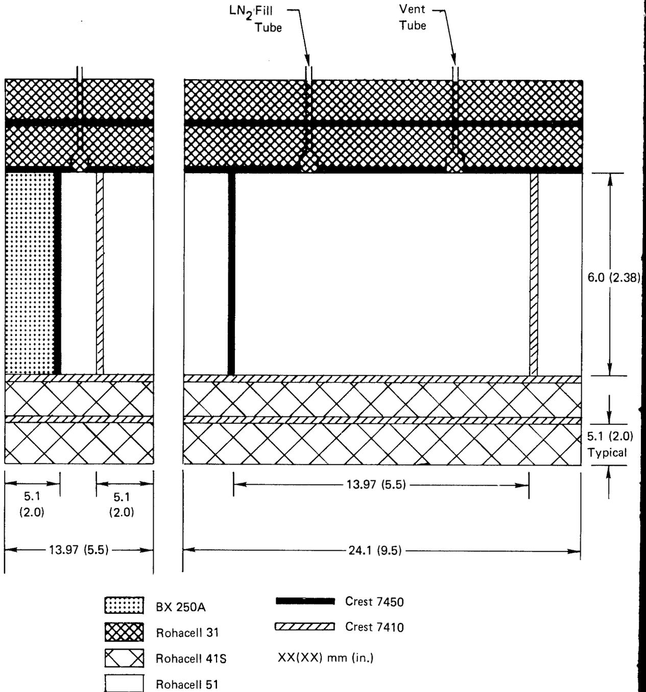
Figure 13. Insulation and Adhesive Test Configuration
