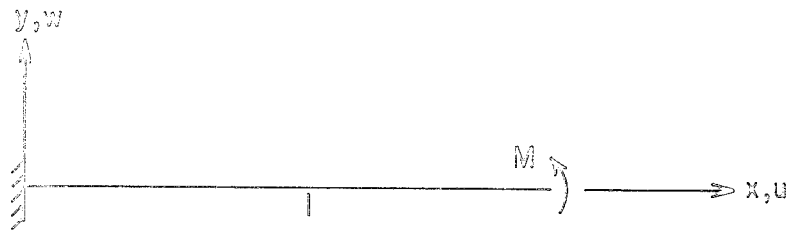
Figure 2a. A Cantilever Beam with a Moment at the Tip
