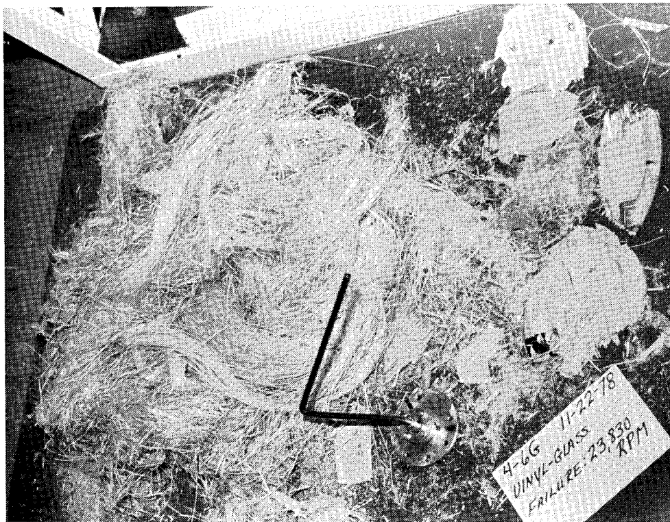
Fig. 25 Typical failure mode of vinyl-glass flywheel.
