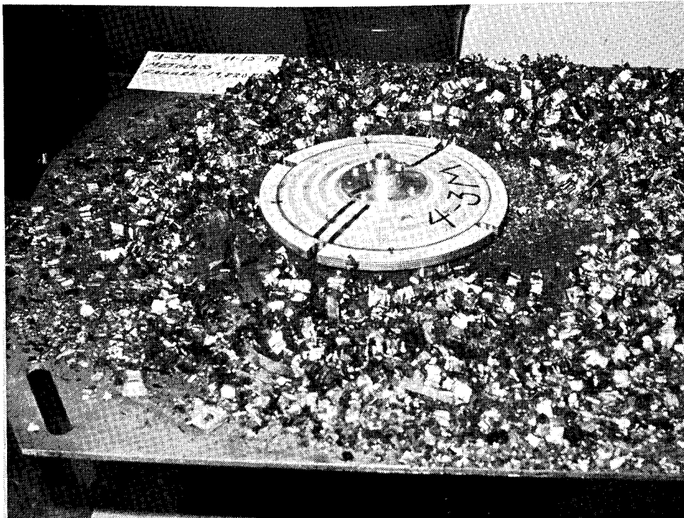
Fig. 36 Typical failure mode of the Metglas-ribbon flywheel.
