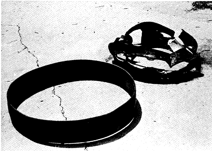
Fig. 18 Containment comparison between P-I disc and wound bare-filament flywheels.
