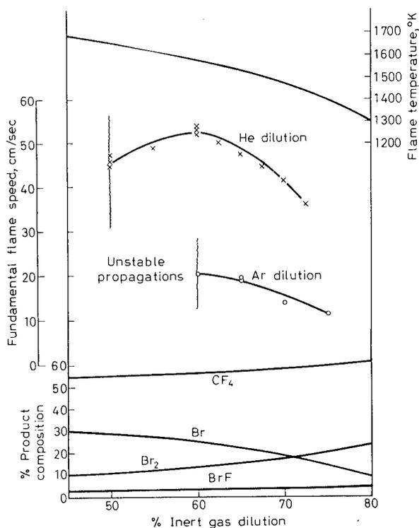
FIGURE 3. Burning velocities, equilibrium temperatures and non-inert product compositions of 65 per cent  $\text{CF}_3\text{Br}-\text{F}_2$  flames diluted with argon (lower curve, circles) and helium (upper curve, x's).
