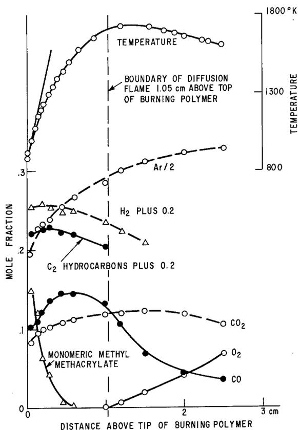
FIGURE 3. Gas composition and temperature along the central axis above a polymethyl methacrylate rod,  $0.36 \text{ cm}^2$  cross section, burning at 5 cm of mercury pressure in argon-oxygen, 20 percent  $O_2$ .
