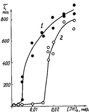
FIGURE 8. Induction period for polypropylene oxidation as a function of  $(\text{CH}_3)_2\text{Si}(\text{OC}_6\text{H}_4\text{HNC}_6\text{H}_5)_2$  concentration, for uniform (1) and nonuniform mixing (2) (200°C).
