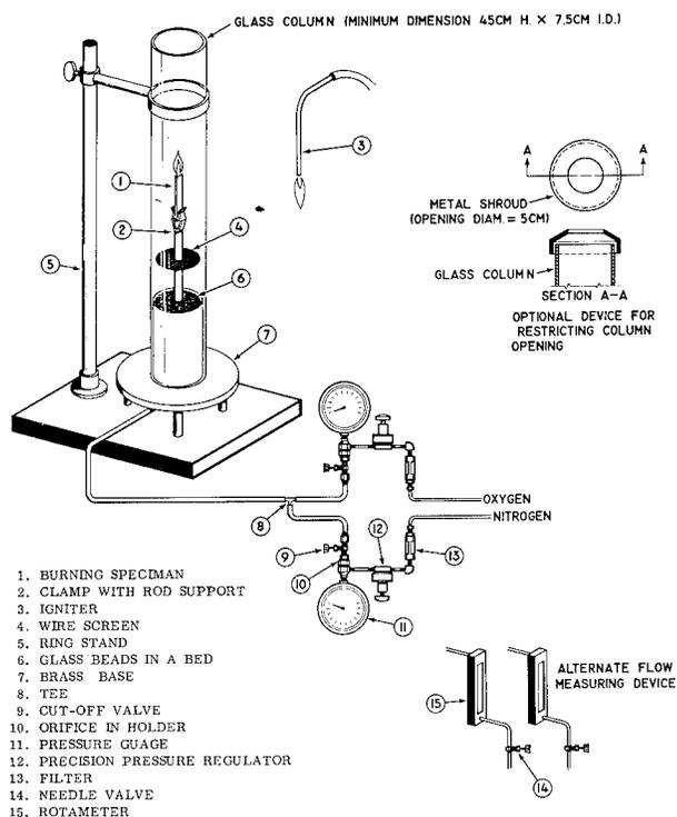
FIGURE 2. Typical apparatus for oxygen index determinations.
