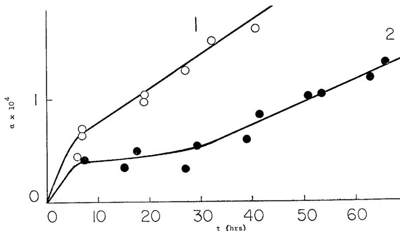
FIGURE 4.  $\alpha$  versus  $t$  for 1 mm Hg of  $\text{NO}_2$  at 35 °C with and without near uv irradiation (no  $\text{O}_2$ ), (1) without, (2) with irradiation.
