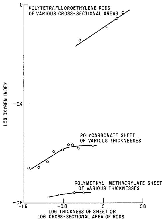
FIGURE 5. Effect of size of burning specimen.
