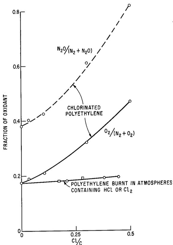
FIGURE 9. Inhibition by chlorine in chlorinated polyethylene.
