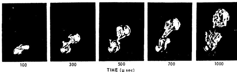
(a) TURBULENT FLAME BALLS 1 ATM STOICHIOMETRIC  $C_3H_8$ -AIR
