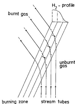
FIGURE 5. Diffusion of hydrogen in the burning zone of an ideally cone-shaped hydrocarbon-air flame.
