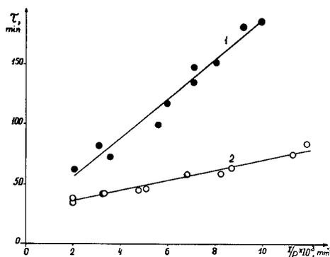
FIGURE 4. Induction period for polypropylene oxidation as a function of the oxygen pressure reciprocal ( $130^\circ$ ).
