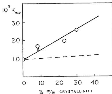
FIGURE 11. Experimental rate constants as function of crystallinity for isotactic polystyrene as function of percentage of crystallinity.
