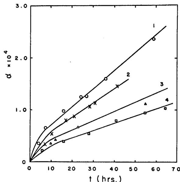
FIGURE 2. Degree of degradation  $\alpha$  of butyl rubber as a function of time for various NO<sub>2</sub> pressures in absence of air at 35°C:
