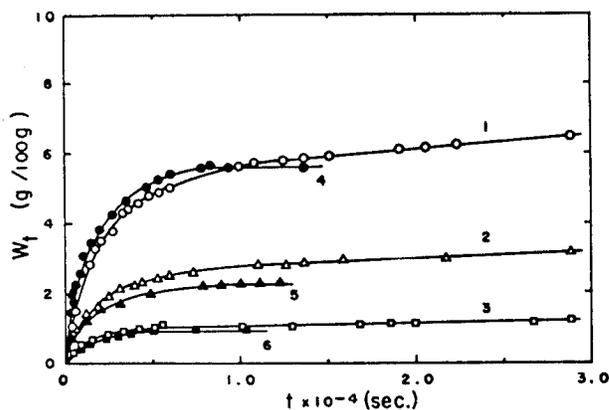
FIGURE 7. Sorption-desorption curves of  $(NO_2 + N_2O_4)$  for polystyrene at  $45^\circ C$ .
