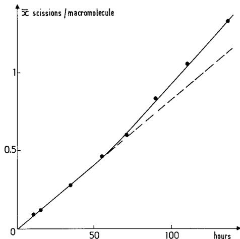
FIGURE 2. Random chain scissions in aqueous solution.
