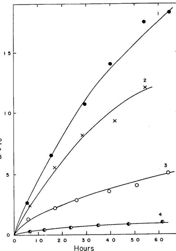
FIGURE 3. Degree of degradation of butyl rubber in presence of 1 atm of air at 35 °C as function of NO<sub>2</sub> pressure and time.
