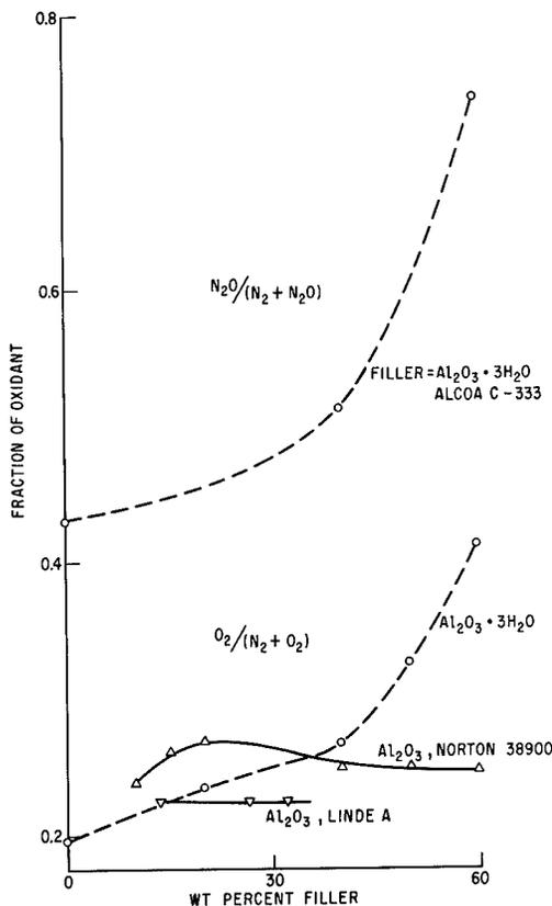
FIGURE 11. Inhibition by fillers in epoxy resin.
