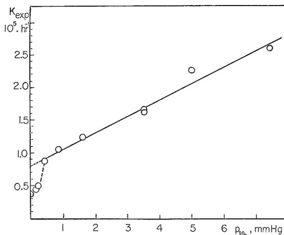
FIGURE 8. Experimental rate constants for isotactic polystyrene as function of sulfur dioxide pressure ( $15$  cm Hg of  $O_2$ ).
