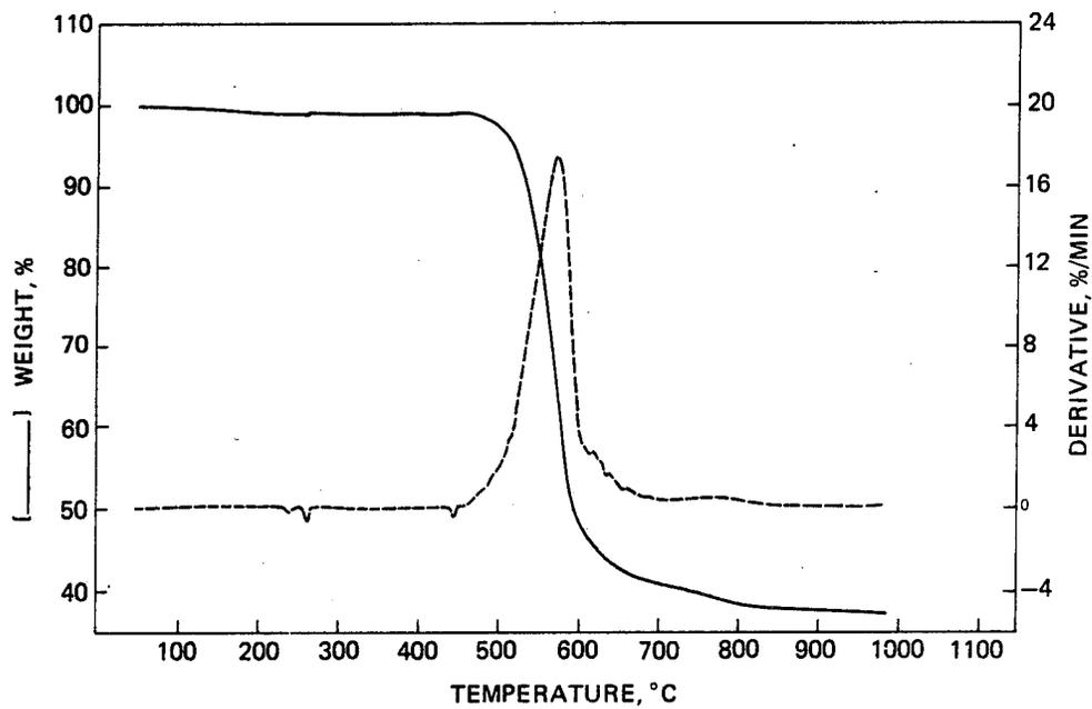
Figure 1 - TG analysis of molded PES 300P resin (in N<sub>2</sub>).
