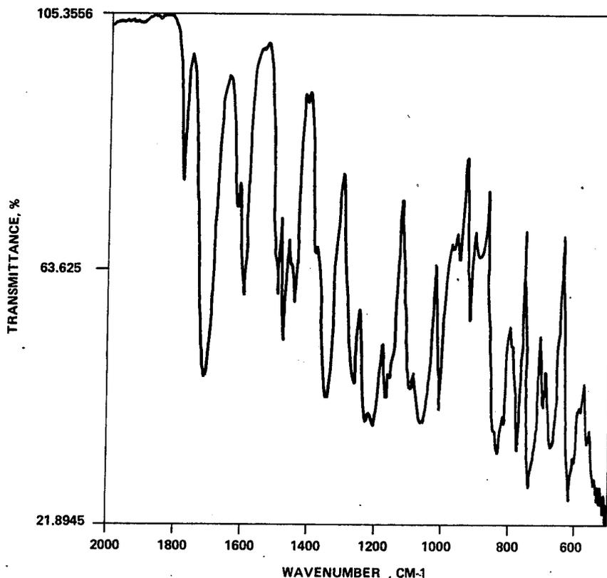
Figure 13 - ATR/FT-IR spectrum of molded PEI (neat).
