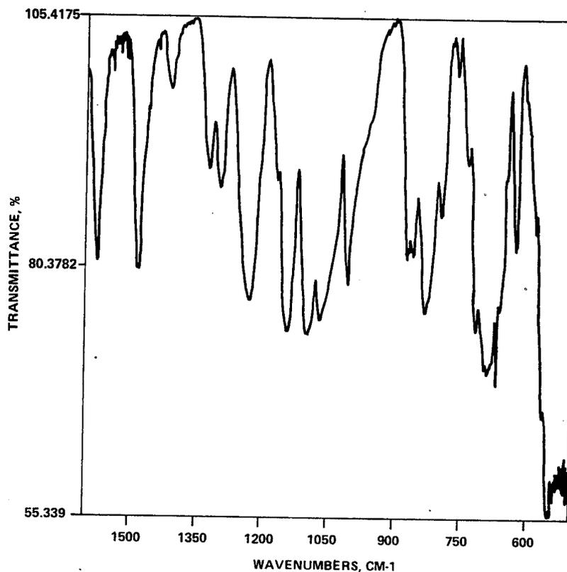
Figure 12 - ATR/FT-IR spectrum of molded PES (neat).
