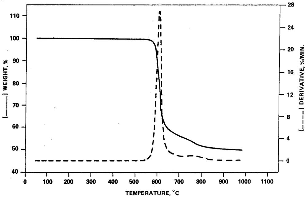
Figure 3 - TG analysis of neat molded PEEK (in N<sub>2</sub>).
