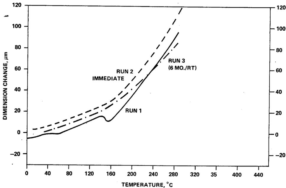
Figure 5 - TMA of molded PEEK (20% FG).
