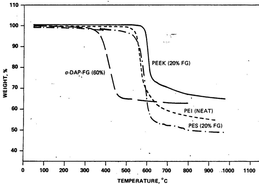
Figure 4 - TG analyses of molded fiberglass-containing resins: PEEK, PES, and o-DAP, and of PEI (neat) in N<sub>2</sub>.
