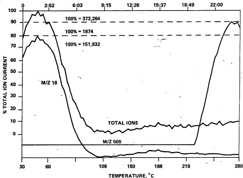
Figure 9 - DIP/MS of polyetherimide (neat).
