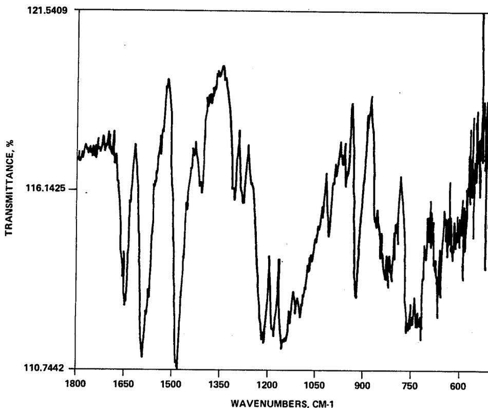
Figure 14 - ATR/FT-IR spectrum of molded PEEK (neat).
