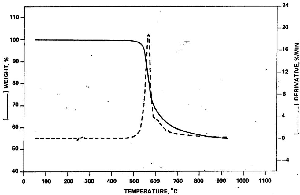
Figure 2 - TG analysis of neat molded PEI (in N<sub>2</sub>).
