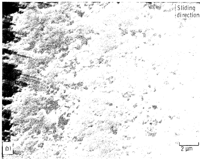
(a) As-received surface. (b) Wear track after 5 sliding passes (load, 1.0 N).
