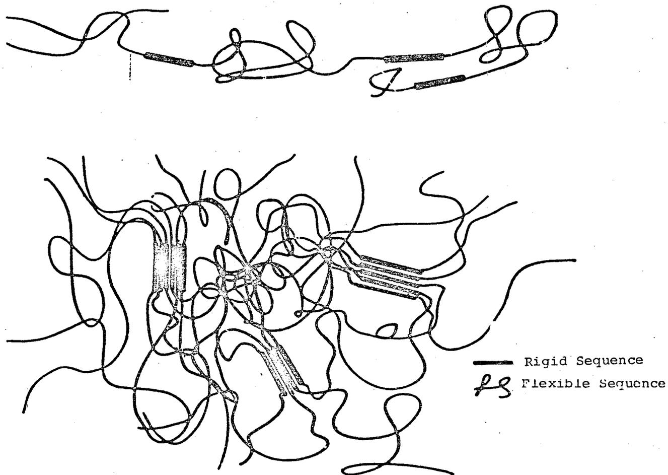
Figure 2 - Structural Model of a Polyurethane
