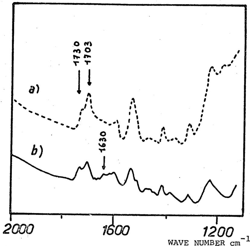
Figure 47 - IR Spectra of C-M400 Composite
