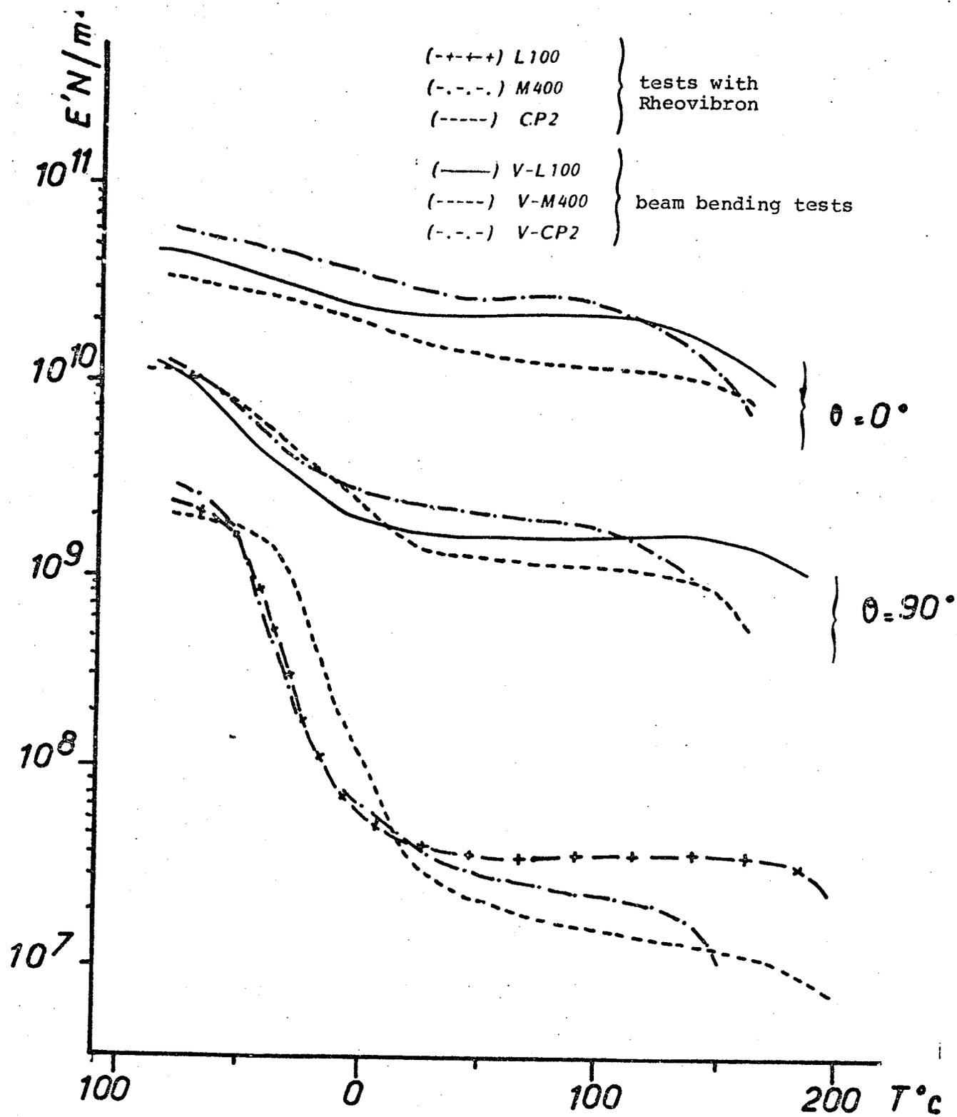
Figure 54 - Variation of the  $E_1$  and  $E_2$  moduli as a function of the temperature of composites V-L100 and V-M400 and V-CP2 (P109 oiling) under beam bending on 3 points, as well as the corresponding matrix, measured with Rheovibron.
