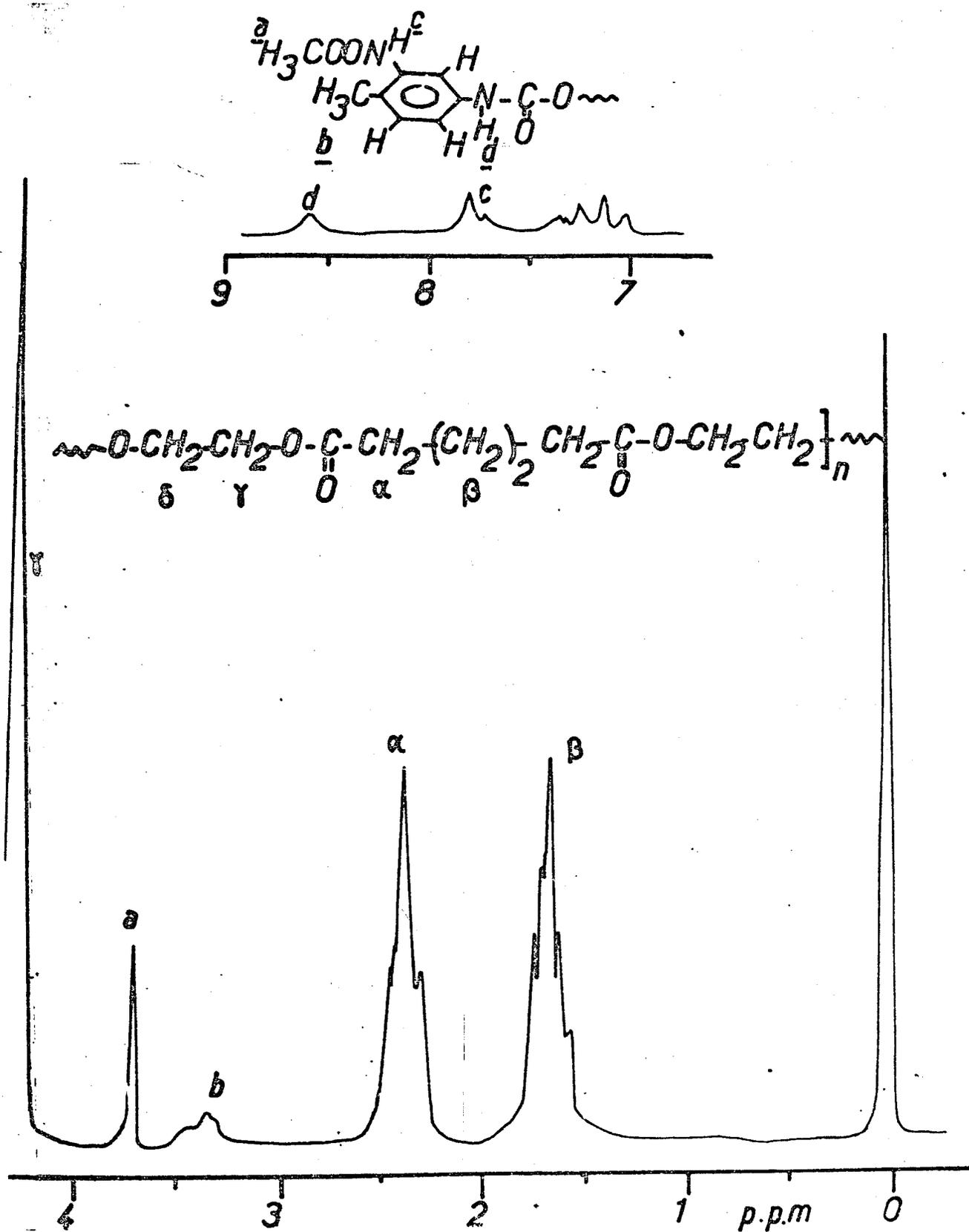
Figure 11 - RMN Spectrum of Cyanaprene A9
