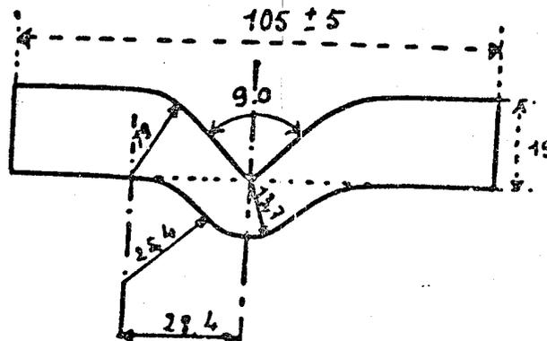
The curves giving the stresses as a function of the deformation are recorded. The curves showing the tensile or tearing properties of polyurethane, such as the modulus of elasticity ( $E_0$ ), the rupture strain  $\sigma_r$ , the elongation at rupture  $\epsilon_r$ , etc. are recorded.
