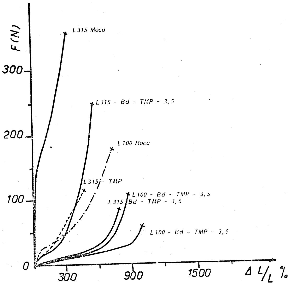
Figure 26 - Curves along the static mechanical properties for PUR -alcohols
