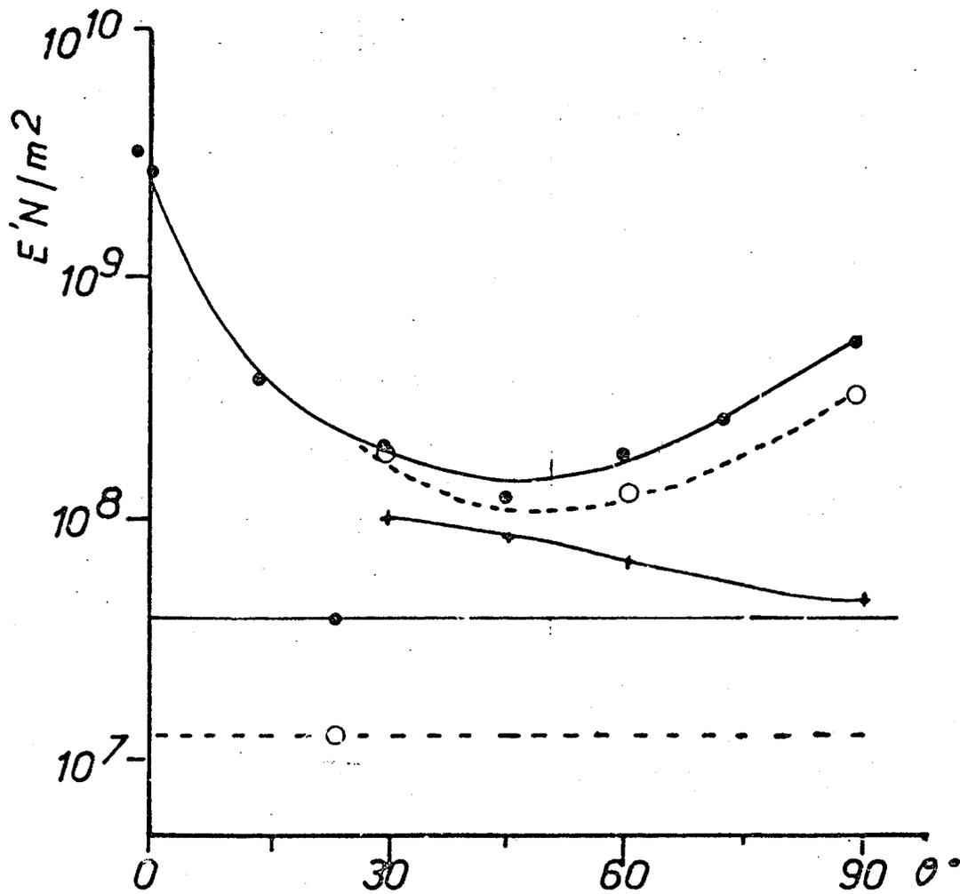
Figure 71 - Variations of the modulus  $E'$  at  $T \gg T_g$  as a function of the cutting angle. This V-L100 composite was prepared with the same V-P109 glass fabric, while depilating the weft.
