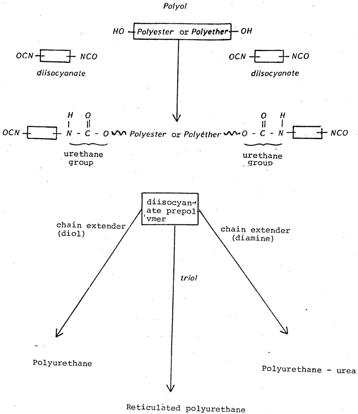
Figure 87 - Obtaining a PUR - General Diagram
