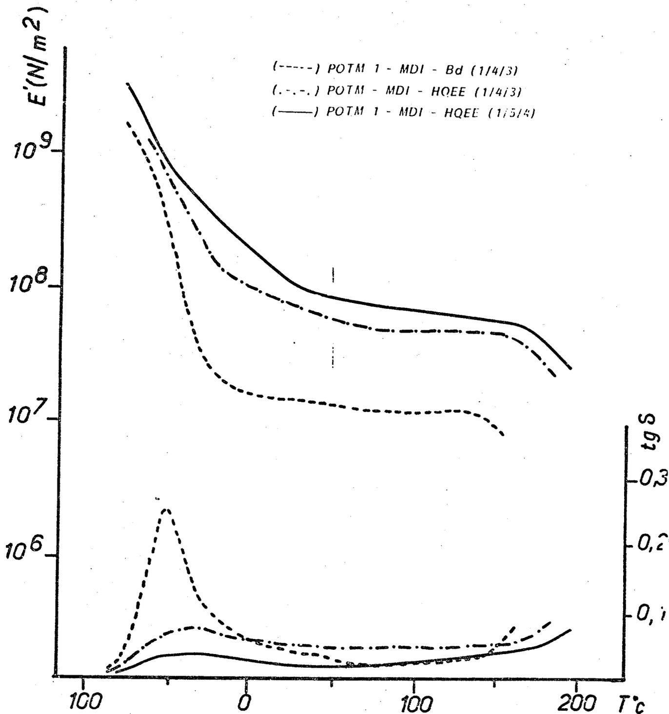
Figure 9 - Curve of modulus  $E'$  and of  $\text{tg } \delta$  as a function of the temperature at 11 Hz for POTM1-based polyurethanes. Comparison between two hardeners: Bd and HQEE.
