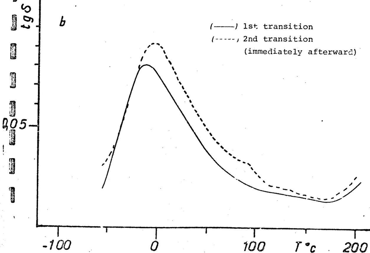
Figure 75 - Behavior of V-L100 composite with layers of fabrics crossed at 90° ( = ± 45°)
