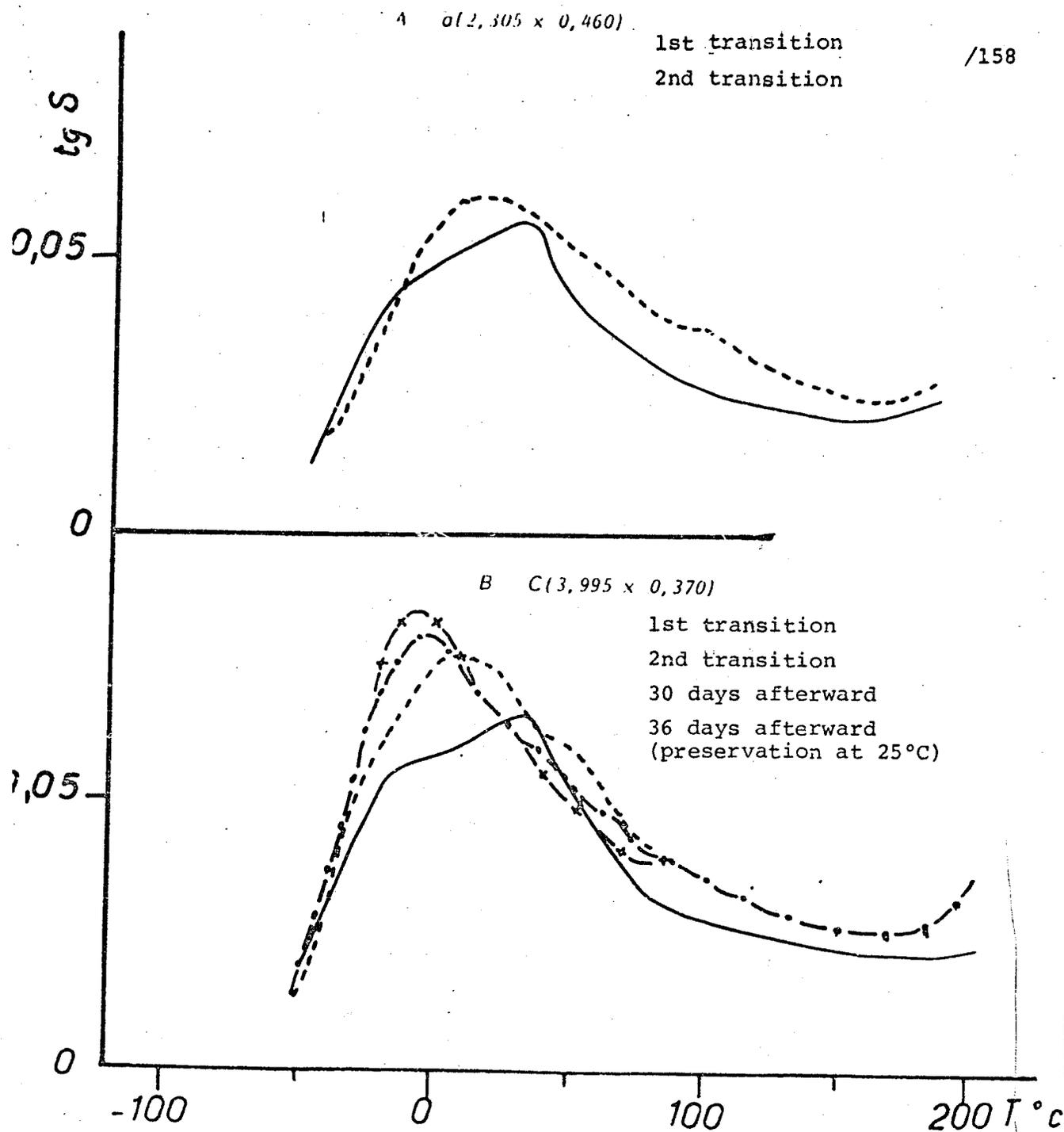
Figure 73: Annealing impact on samples cut out at 60°
