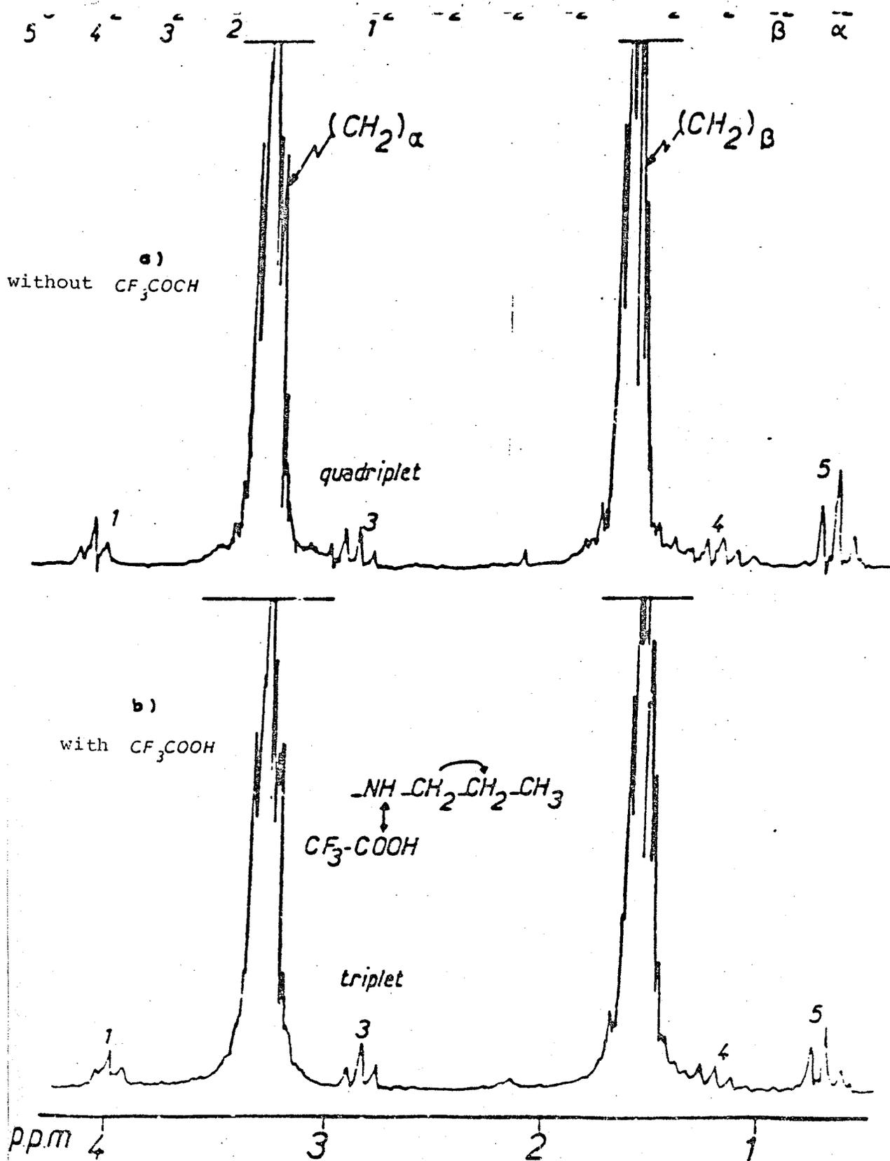
Figure 86 - RMN  $^1H$  spectrum of a glycol polyoxytetramethylene after reaction with n-propylisocyanate.
