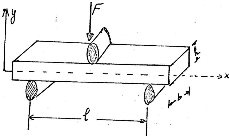
Figure 88 - Bending Test on 3 Points
