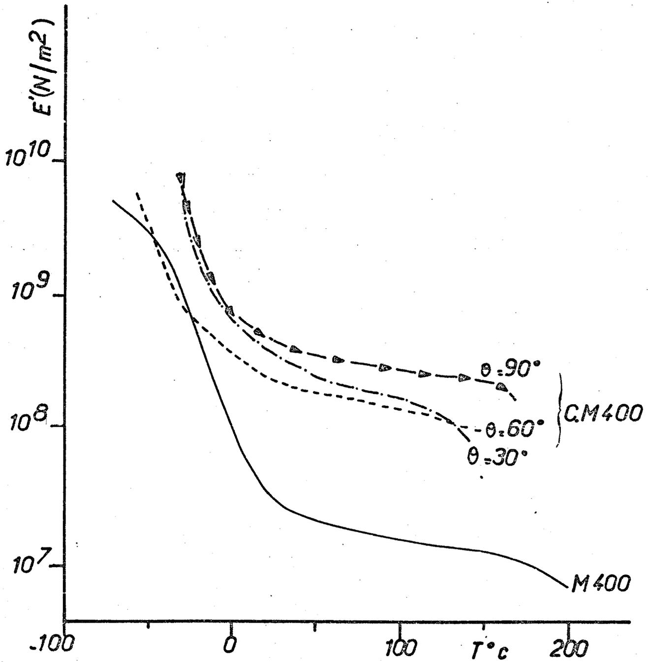
Figure 82 - Curves giving  $E'$  as a function of the temperature for PUR-M400 (—) and C-M400 composite according to various angles  $\theta$ .
