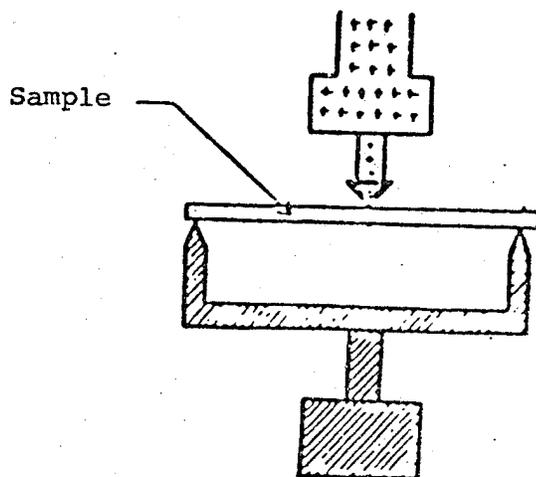
Figure 64 - Dynamic mechanical properties under beam bending forces.
