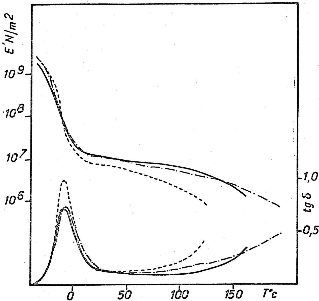
Figure 5 - Variation of  $E'$  and  $\text{tg } \delta$  as a function of the temperature for PURs prepared from Bd (-----), from HQEE (——) and xylene diol (-.-.-.).
