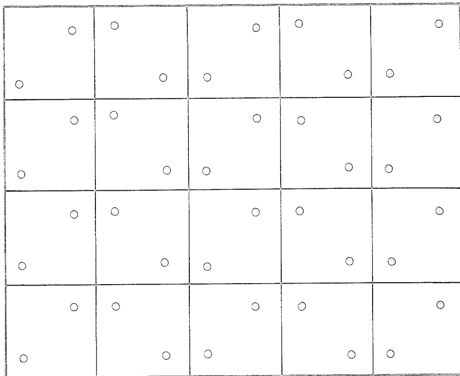
Figure 2.- Evaluation points for alternate two-point integration.
