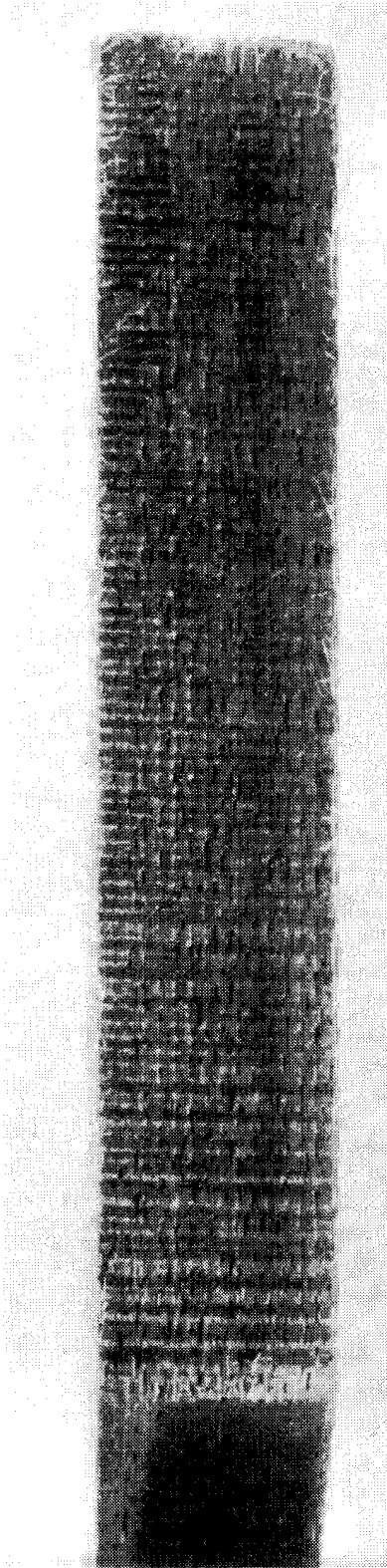
Figure 5. Contour Stepping Problem with 0.0254-mm Input Resolution
