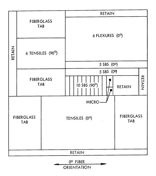
FIGURE 7 TEST SPECIMEN LAYOUT FOR LAMINATE VI.
