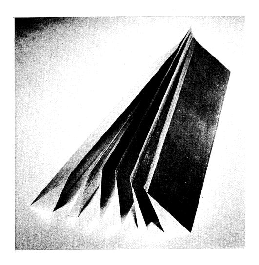
Figure 12. Blade Root Wedges Ready for Priming.
