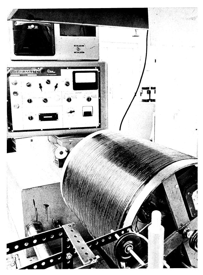
Figure 9. Glass/Graphite Hybrid Prepreg.
