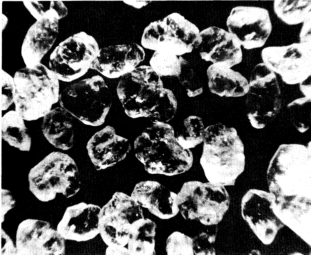
Figure 7. Photomicrograph (x90) RDX, Type B, Class A >#200 Mesh
