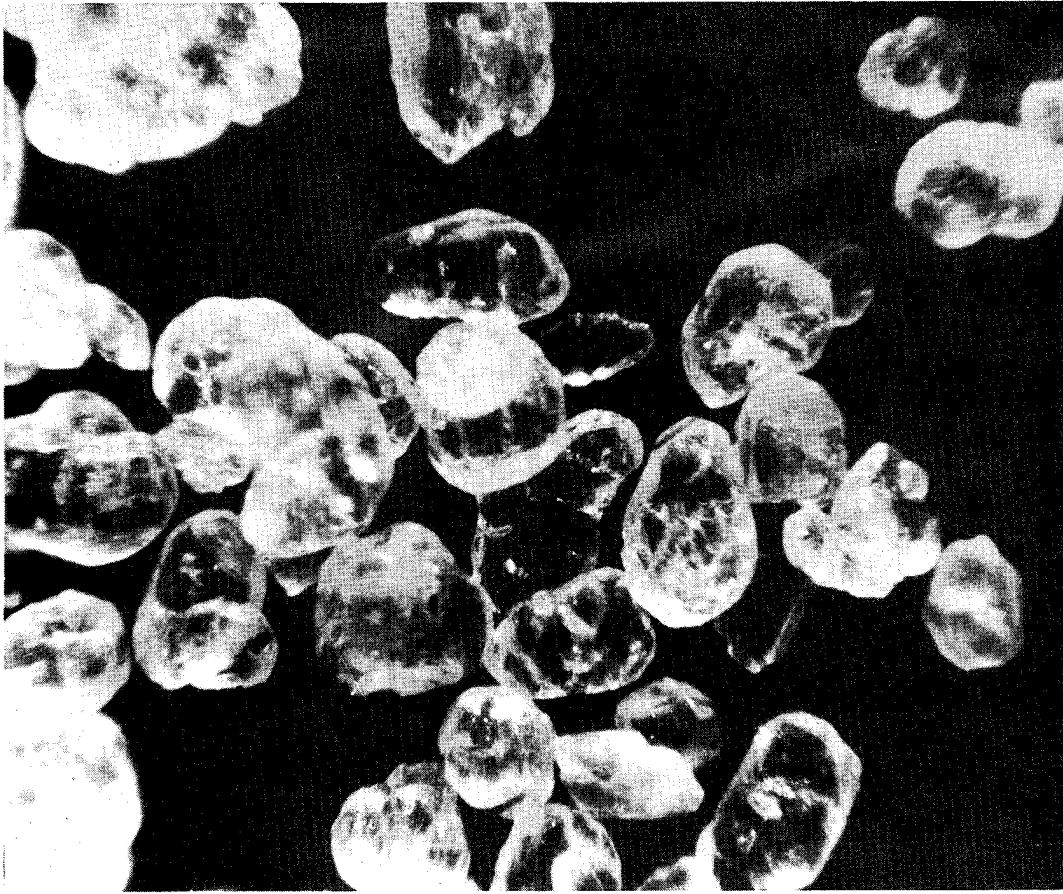
Figure 8. Photomicrograph (x90) RDX coated with 1.5% Parylene C
