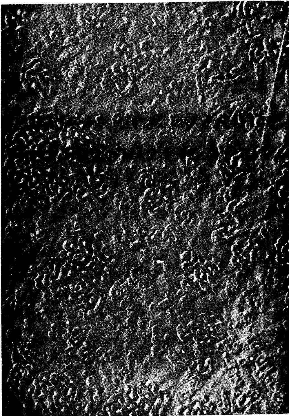
Figure 7 - Electron micrograph of a surface replica of an alternating styrene-2-vinyl pyridine block copolymer film (R-29).
