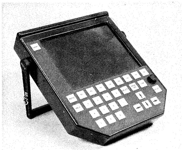
Figure 2. Demonstration System Portable Maintenance Aid
