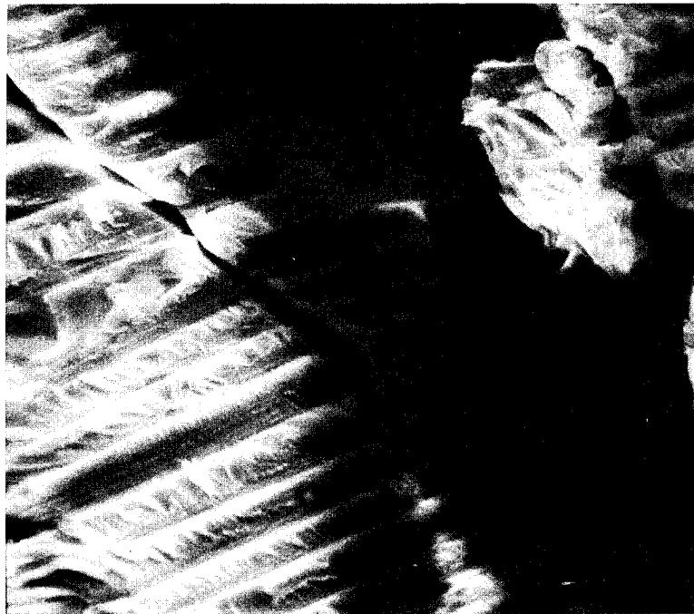
(b) Specimen No. 8, 1 x 1010 Rads Dose at 120°C, Tested In Vacuo
