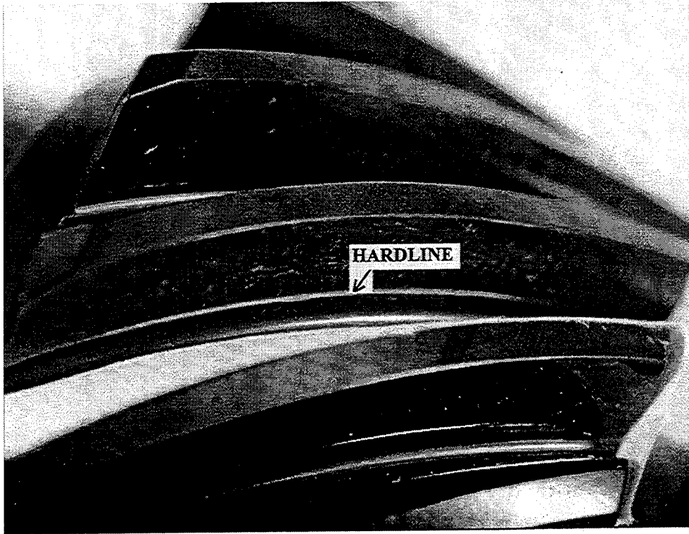
FIGURE 86: HARDLINE IN FLANK OF CONF. #3C SPIRAL BEVEL PINION AFTER 180 HR PITTING/BENDING TEST
