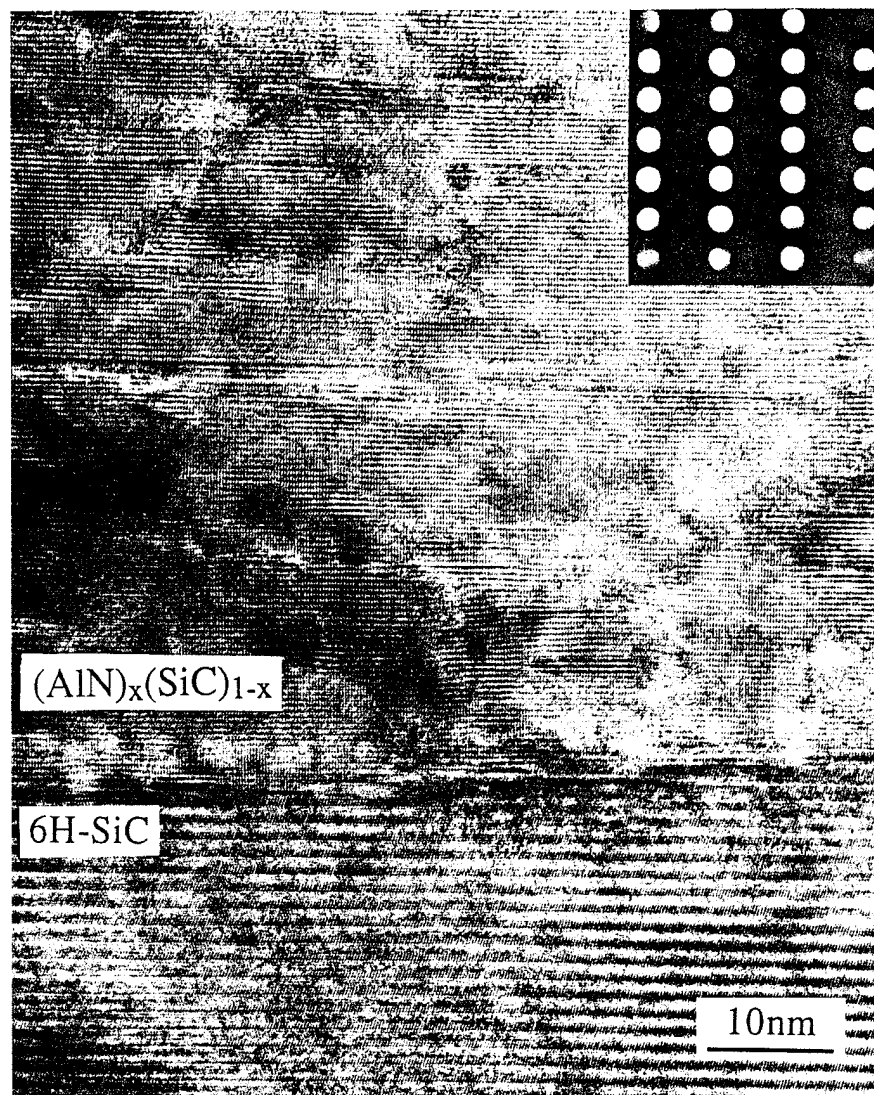
FIG. 2. High-resolution transmission electron micrograph of the 2H (\text{AlN})_x(\text{SiC})_{1-x} thin film grown on an \alpha (6H)-SiC(0001) substrate and used to obtain the Auger depth profile in Fig. 1. The inset shows the micro-diffraction pattern of this 2H film taken along the [11\bar{2}0] zone axis.
