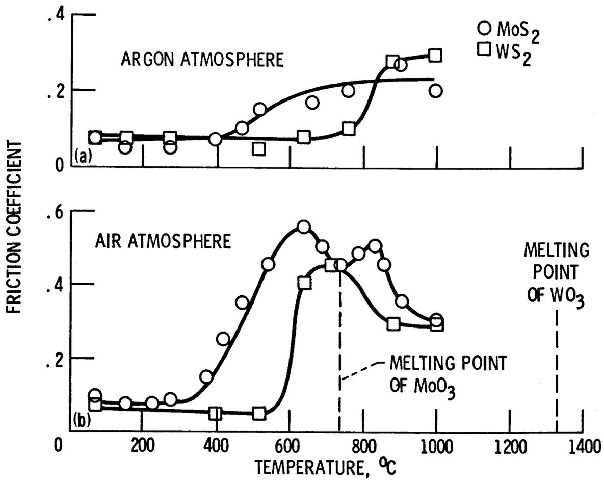
Figure 12.- Friction characteristics of MoS<sub>2</sub> and WS<sub>2</sub> in argon and in air.
