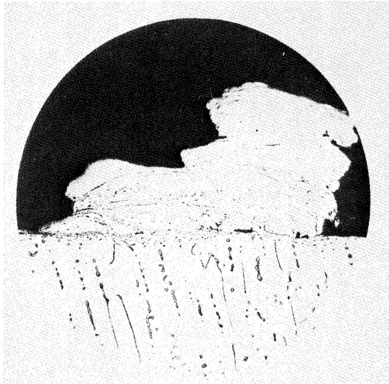
Figure 1.- Severe surface welding resulting from unlubricated sliding (2% Al-Ni alloy from 10<sup>-9</sup> mm Hg vacuum experiment).
