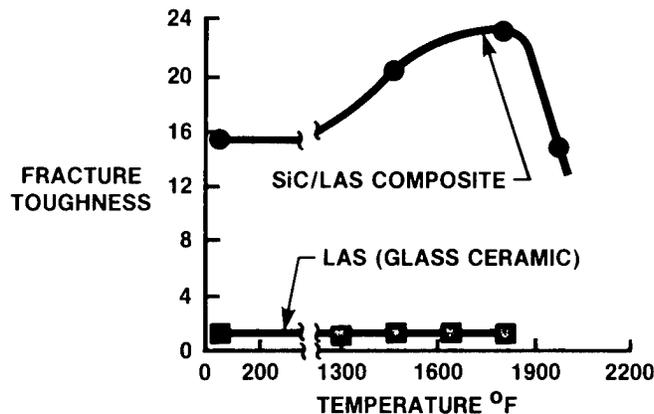
**BUT, HIGHER TEMPERATURE CERAMIC MATRIX COMPOSITES DEGRADE DURING FABRICATION DUE TO—**
