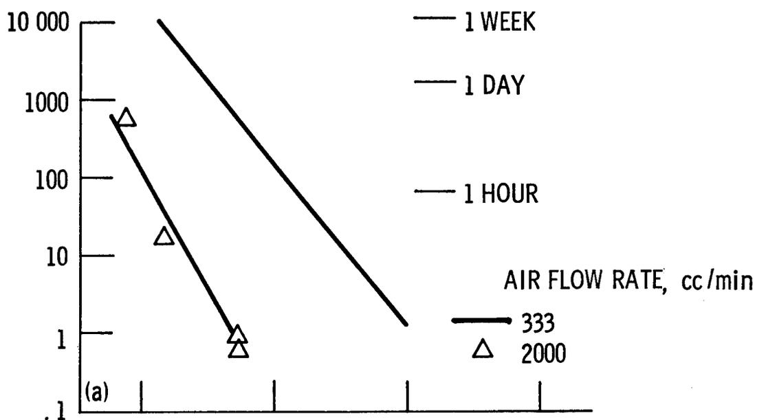
(a) Oxidation characteristics of MoS<sub>2</sub> at two air flow rates.
