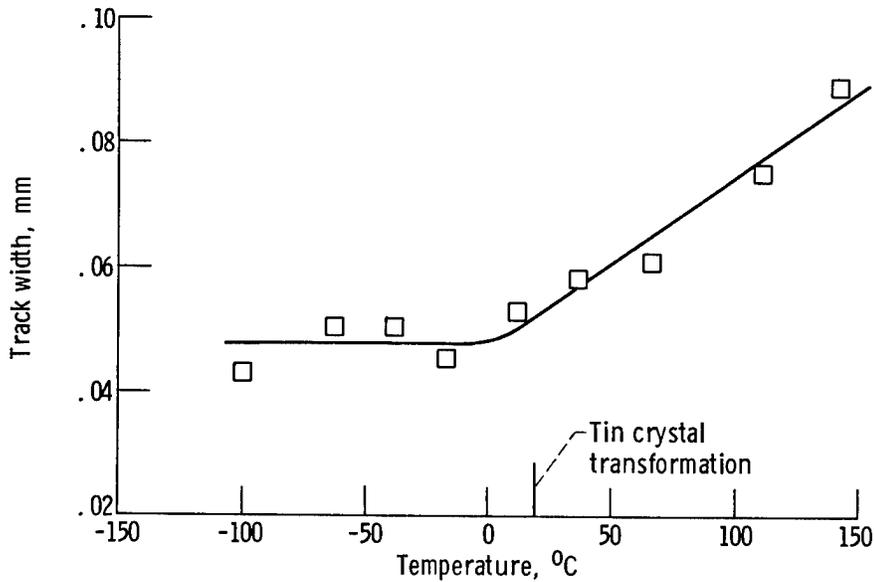
Figure 6.- Track width on tin single-crystal surface as function of temperature. Sliding velocity = 0.7 mm/min; load = 10 g; pressure =  $10^{-8} N/m^2$  ( $10^{-8} N/m^2$ ); rider = iron (110); single pass.
