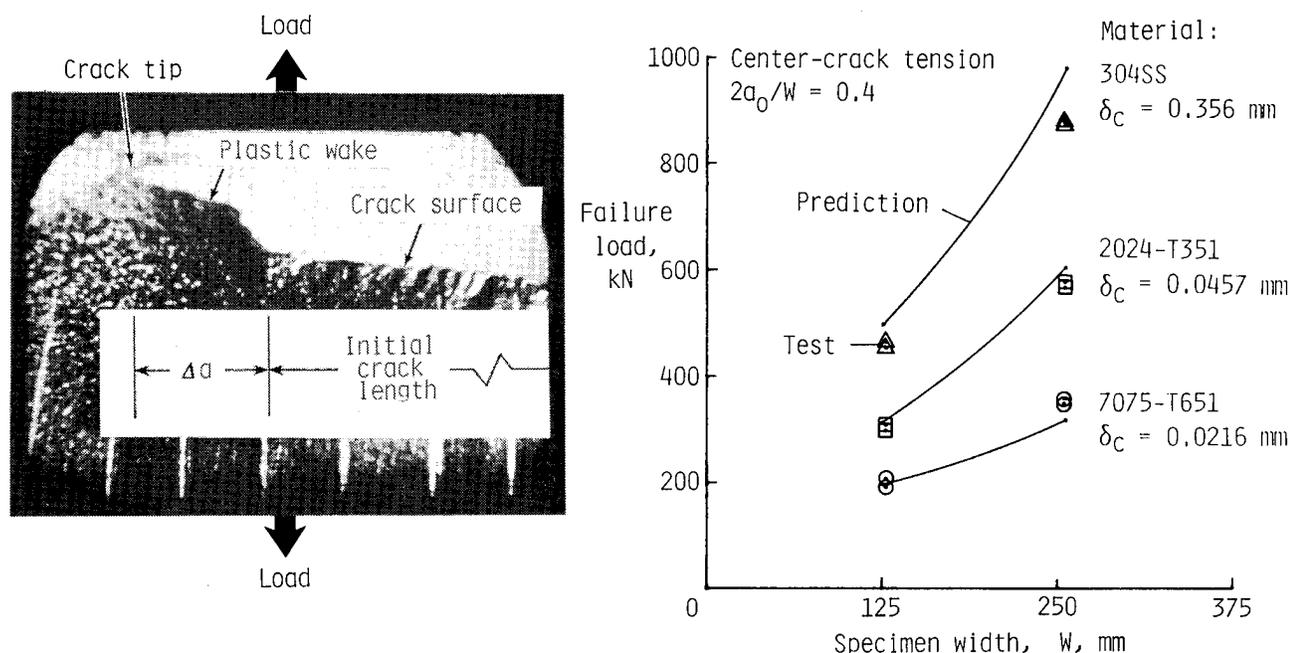
Figure 7.- Plastic-wake concept: test and finite-element predictions.
