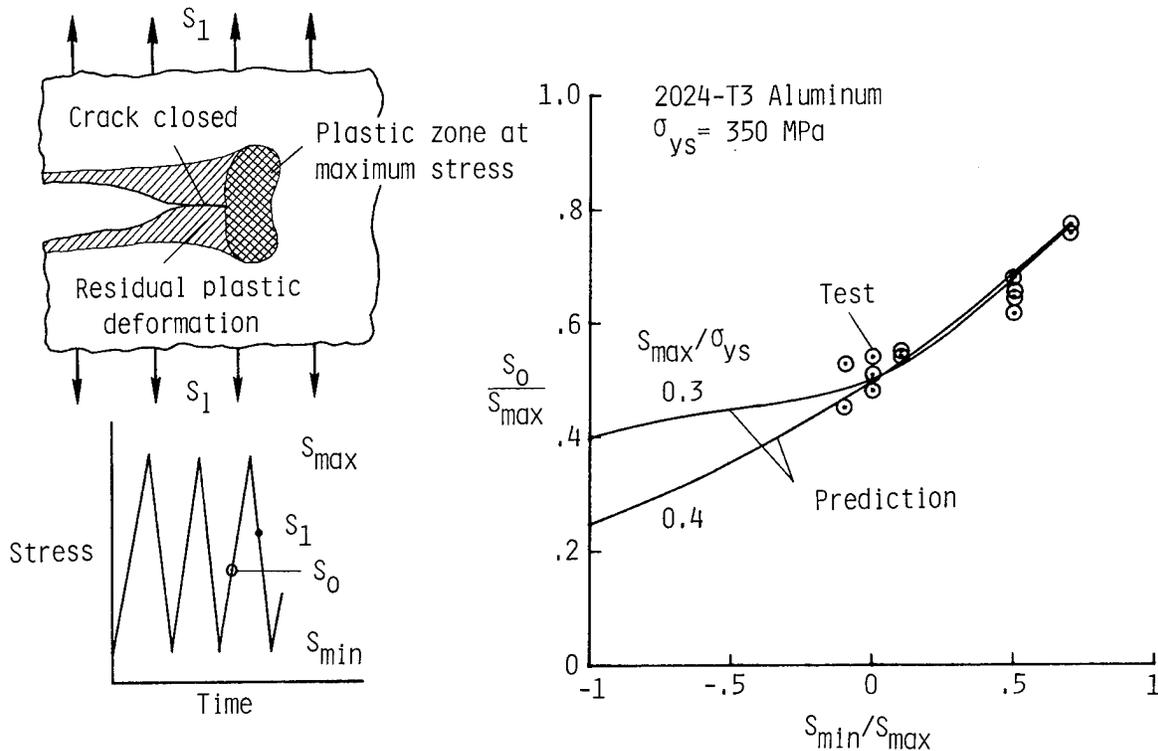
Figure 4.- Fatigue crack closure concept: test and analysis.
