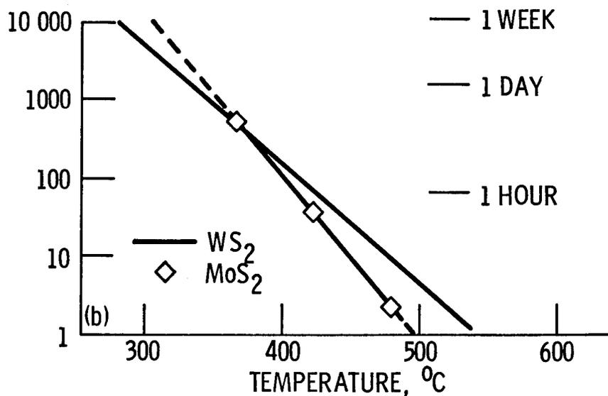
(b) Comparative oxidation of WS<sub>2</sub> and MoS<sub>2</sub> air flow rate, 1/3 L/min.
