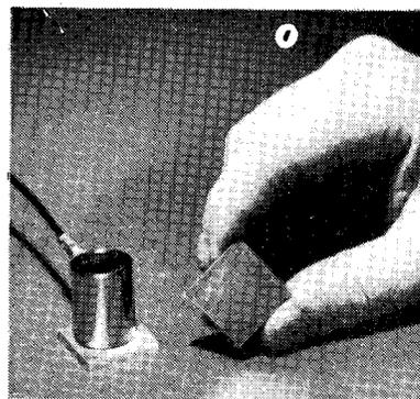
*In many cases, destructive fracture toughness tests require huge specimens. LeRC's new ultrasonic technique uses only a small metal sample.*
