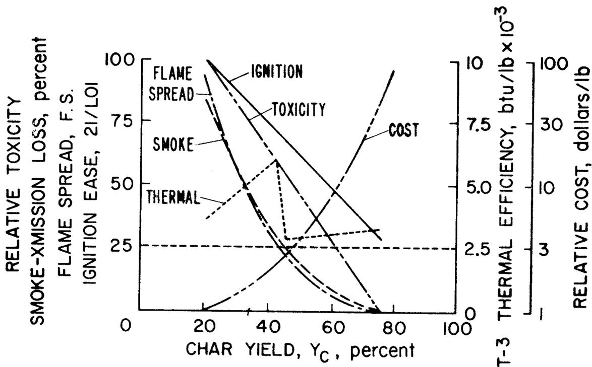
Figure 2.- Summary of properties of char-forming foamed polymers.
