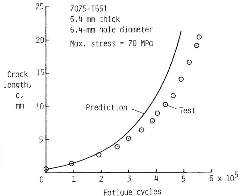
Figure 3.- Wing failure due to corner crack at hole and experimental verification of analysis.
