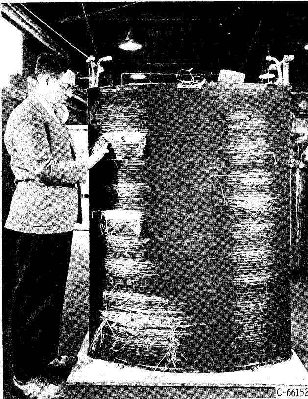
Figure V-12. - Insulation system 1 after being subjected to simulated launch tests. Maximum surface temperatures unknown.
