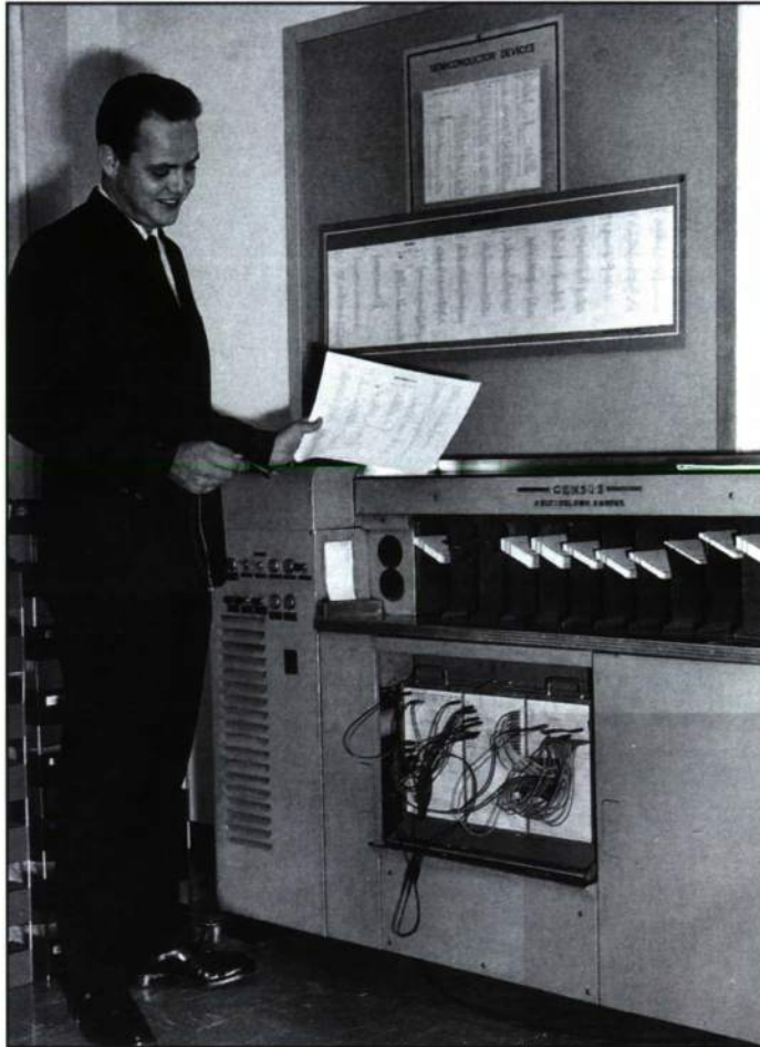
This punch card sorter, programmed with a plug board, was part of the automated data processing system from the mid-1960s through the early 1970s.
