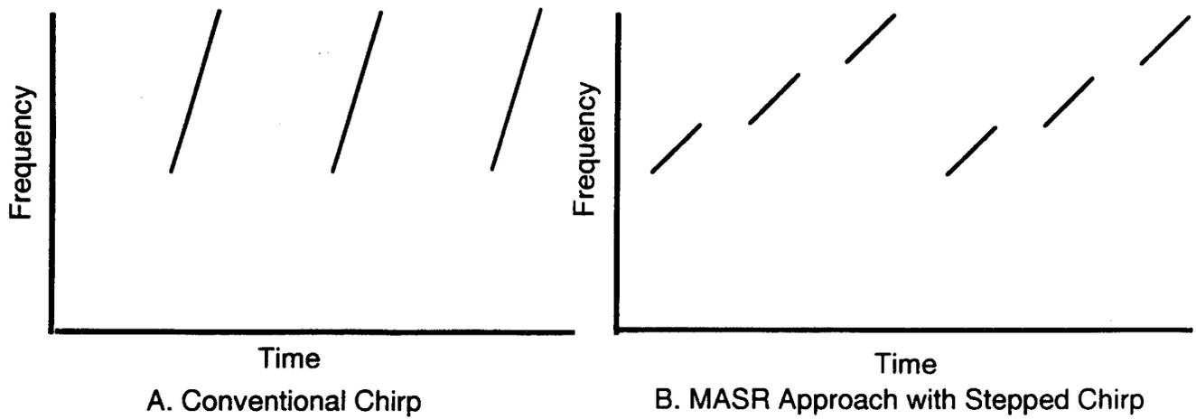
Figure 3.3 Transmitted Waveforms for Fine Range Resolution
