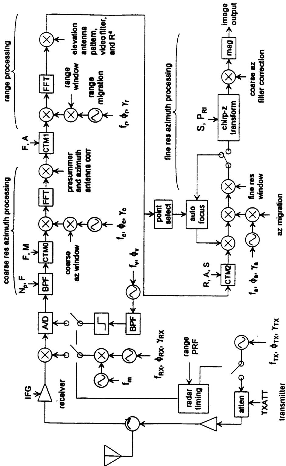
Figure 4.2. SAR-P Radar Signal Flow Diagram
