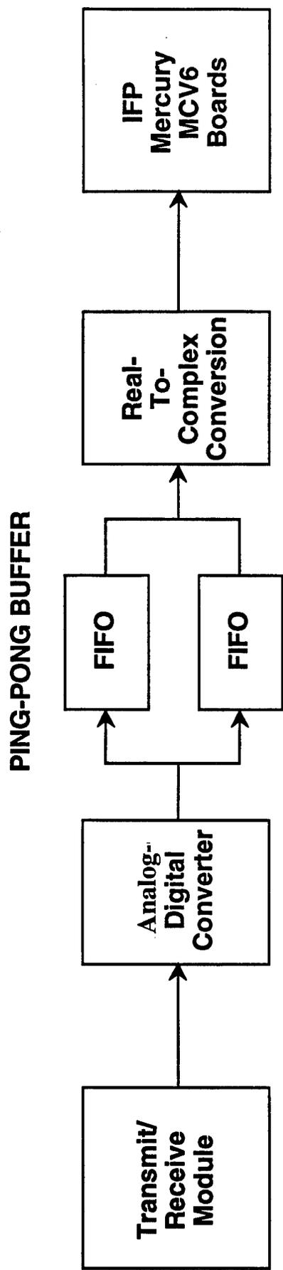
Figure 3.13. MASR H/W Block Diagram
