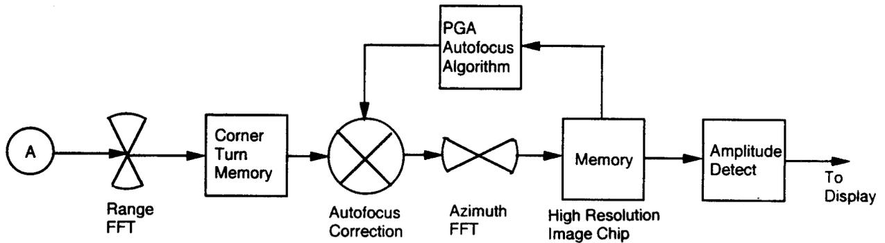
Figure 3.8c MASR Fine Resolution Processor Block Diagram
