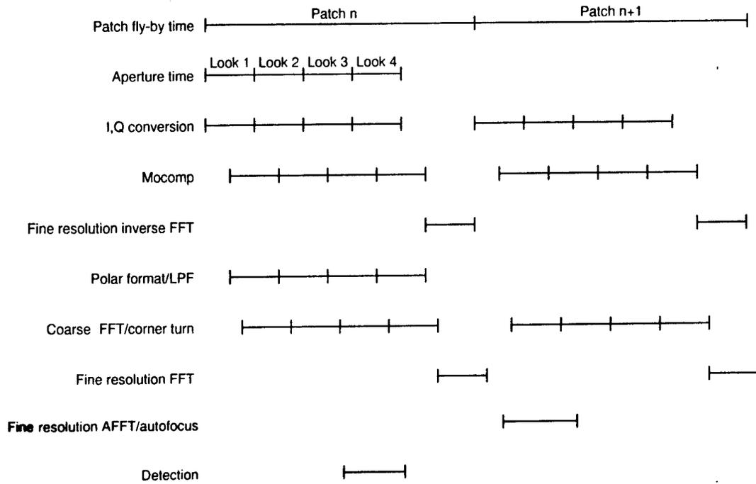
Figure 3.10 Macro Timing Diagram
