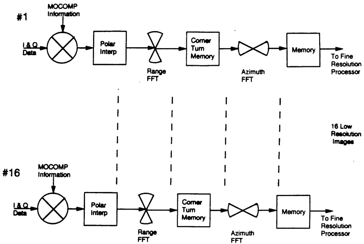
Figure 3.8b. MASR Coarse Resolution Processor Block Diagram
