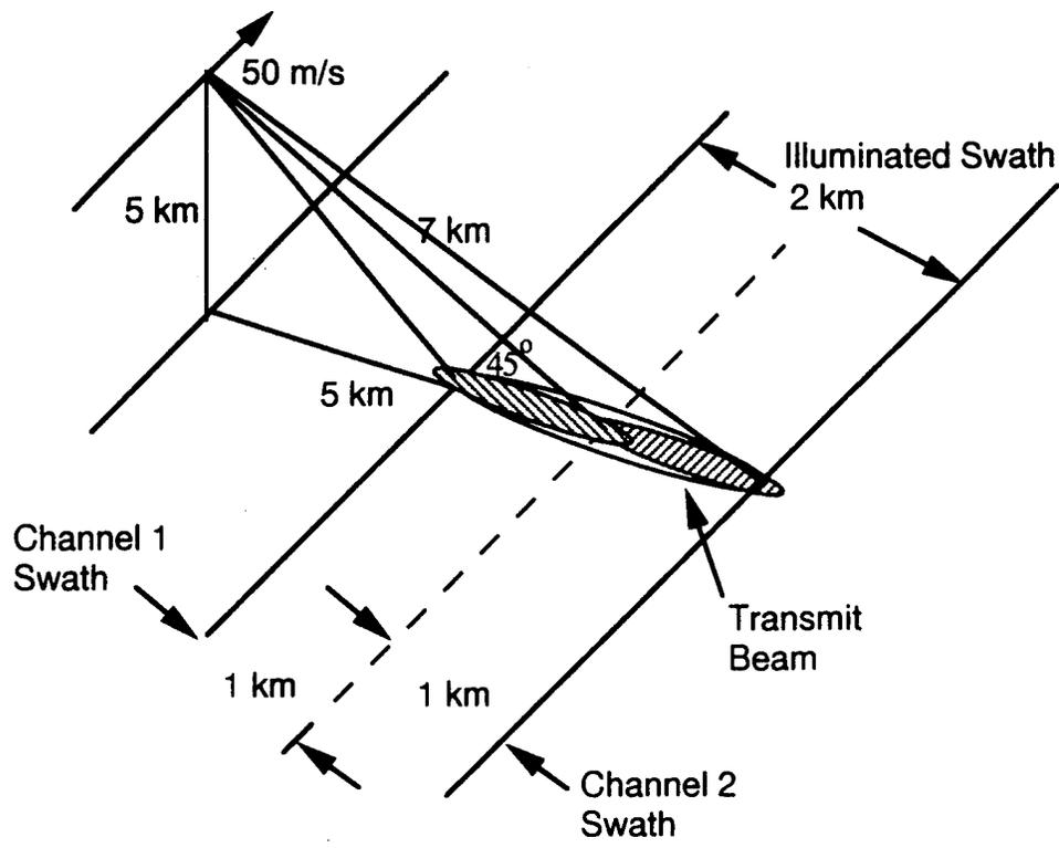
Figure 3.7 Geometry for MASR Point Design 2
