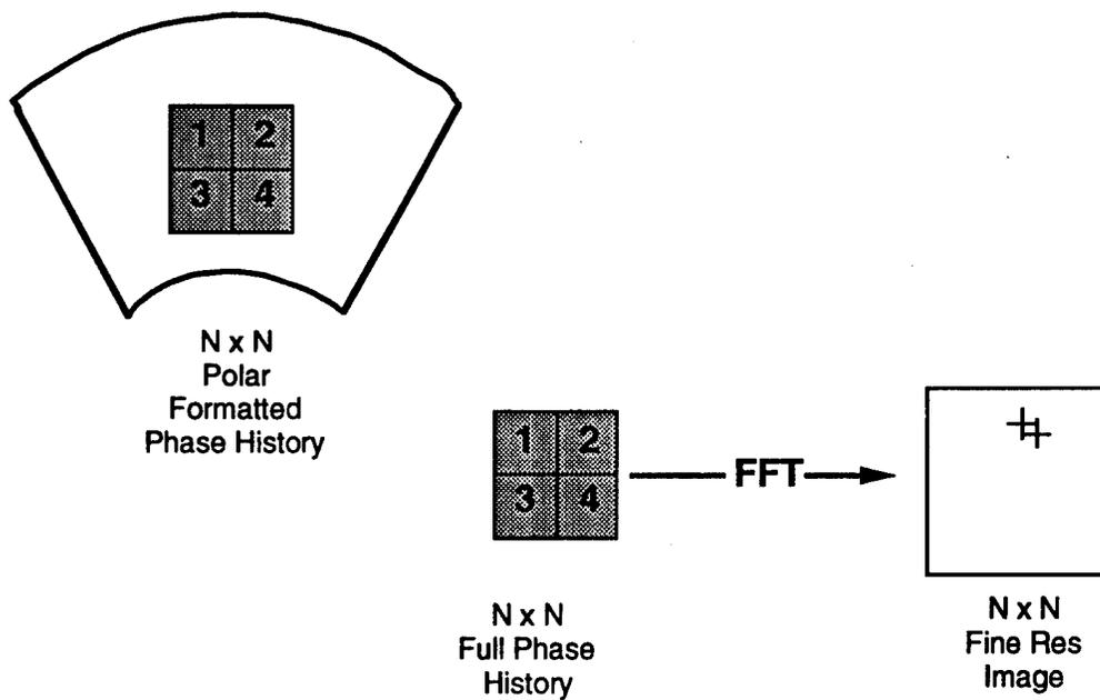
Figure 3.4 Fine Resolution by Conventional Processing Approach
