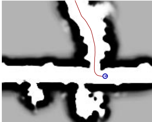
Figure 14: Example of the XAVIER robot leaving a room. The two-dimensional occupancy map (bird's eye view of the robot's environment) has been constructed previously, based on sonar sensor information. Bright values correspond to free space, and dark values to occupied regions.
