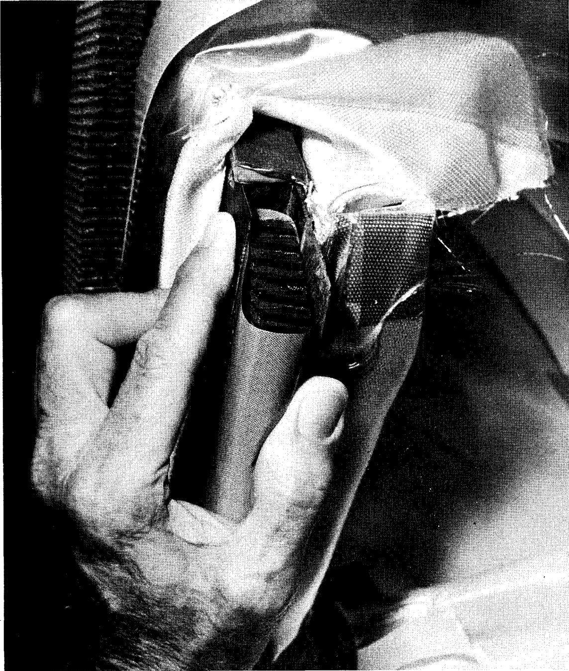
Figure 206. Honeycomb Inserted in TDS Cover Open Channel Closeout
