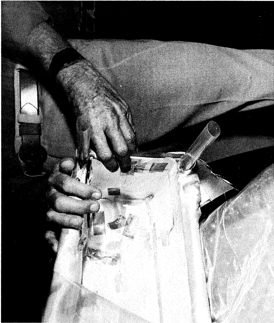
Figure 211. Teflon Tubes Inserted in Aft Open Channel Closeouts
