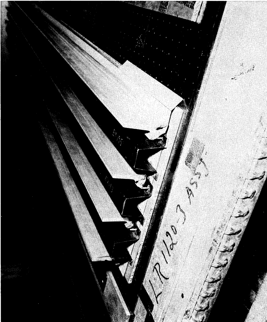
Figure 115. Hat Stringer in Position on Skin With "1" Pressure Cauls Installed
