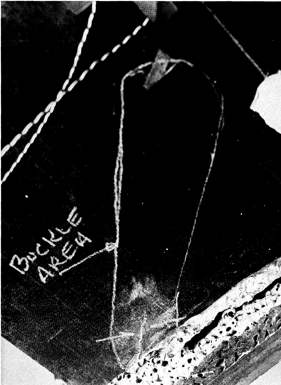
Figure 155. "Hat" Element EX195-3A, Local Skin Compression and Buckling Failure, 316°C (600°F) Test, Aged Condition.
