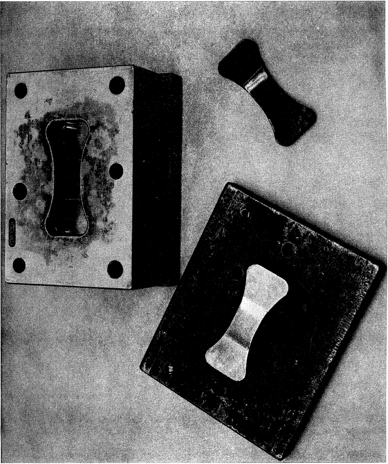
Figure 103. ASTM D647 Tensile Mold and Molded ASTM D651 Tension Coupon
