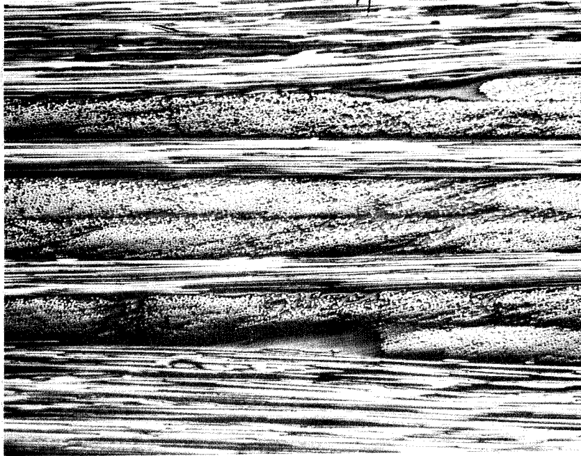
Figure 22. Specimen A-8-17, +45^\circ Ply Drop-offs: Outside -45^\circ Plies (Ply Nos. 12 and 19) Dropped Off.
