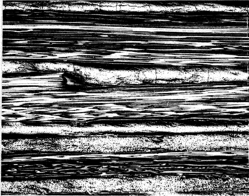
Figure 17. Specimen A-6-1, 0° Ply Drop-offs: Upper Region Shown (Ply No. 9 Dropped Off).
