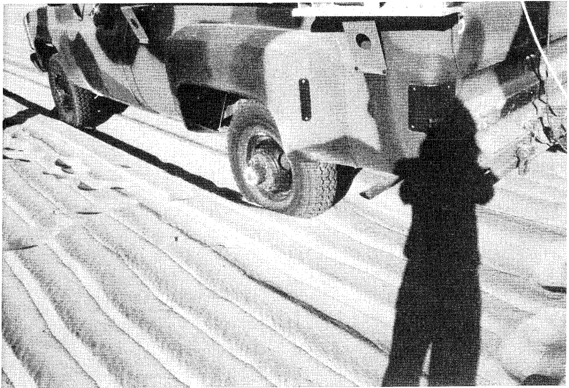
a. M1028 with 33X12.5R16 tires at 30 psi inflation pressure.
