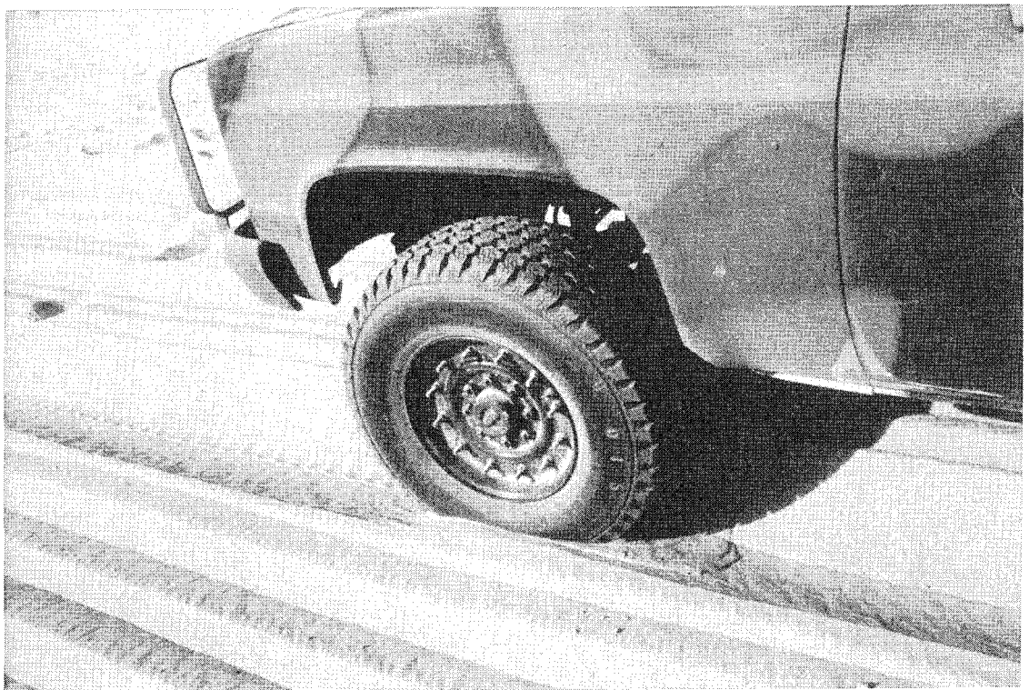
b. M1028 with 33X12.5R16 tires at 25 psi inflation pressure.
