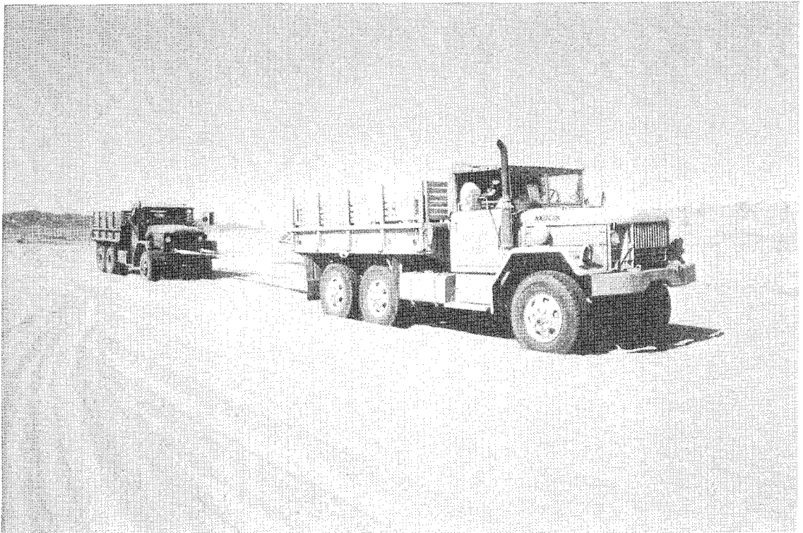
f. M35A2 with singles at beginning of DBP test.
