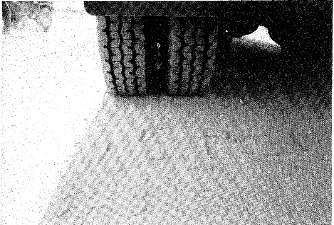
c. M54A2 with 11.00R20 tires at 15 psi inflation pressure.
