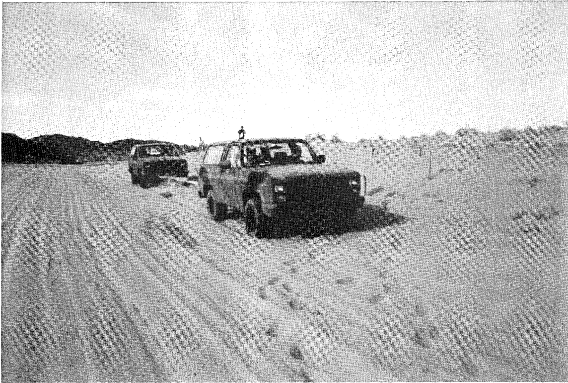
c. M1009 at during DBP test.
