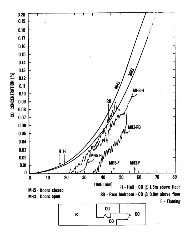
Figure 7. Calculated and measured CO concentrations for a chair smoldering in a closed mobile home.
