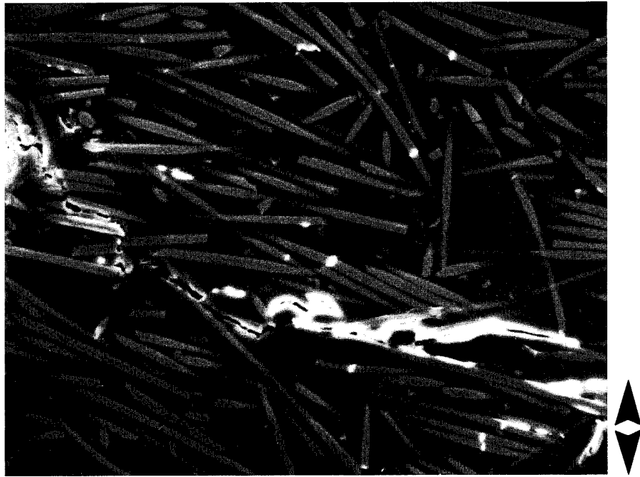
Figure 10. (a) Crack propagation from the notch tip (far left arc) is mainly along the interface in the case of the T-specimen. Matrix crazing is the joining mechanism of pre-existing interface cracks.
