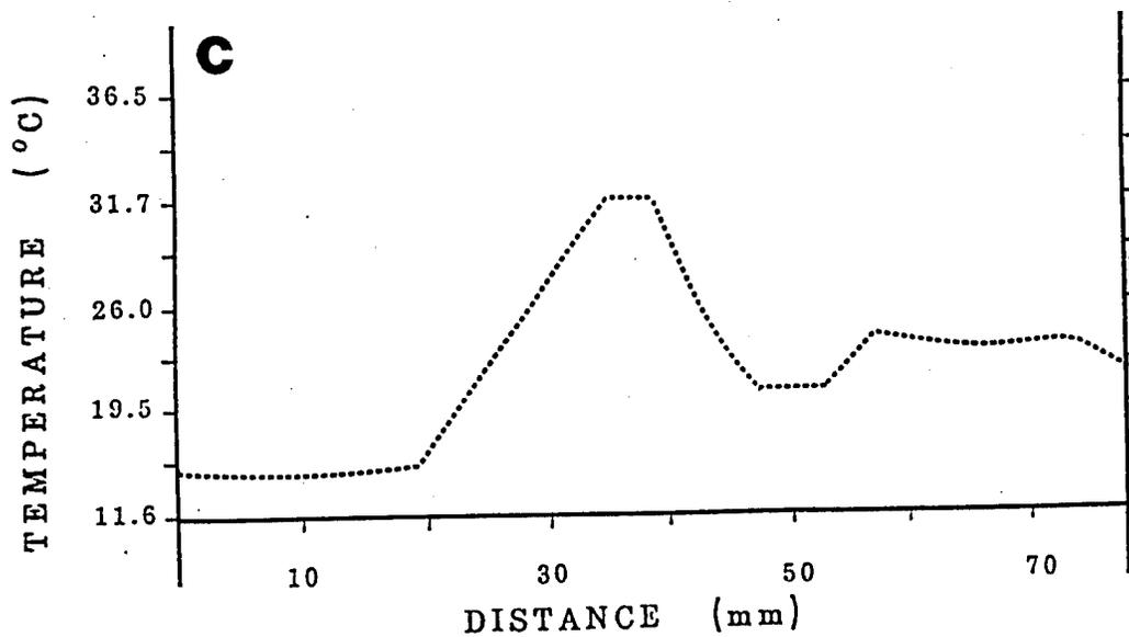
Fig. 4 Temperature images and graphs of profiles of the heating of the corneal phantom by the focused beam of millimeter waves from the antenna.
