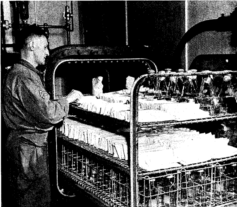
FIGURE 113.—Autoclave being loaded with bottled solutions and equipment for collection of blood, European Theater Blood Bank, 1944.
