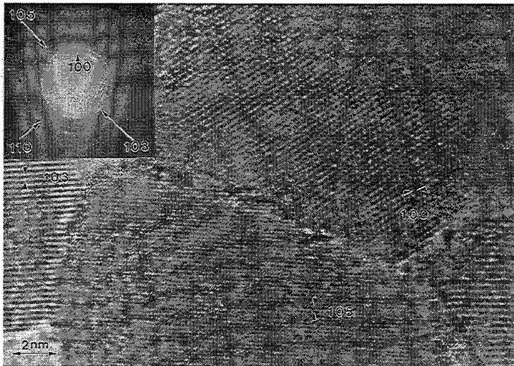
Fig. 3. Particles which show the (103) and (105) fringes and which dominate the morphology of an AT film annealed to 500–550°C in an UHV environment. The relative intensities of the corresponding rings in the inset diffraction pattern are proportional to their population density.
