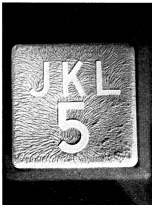
Fig. 9. Polyacetal specimen after outdoor exposure for two summers. (P. G. Kelleher, unpublished results.)
