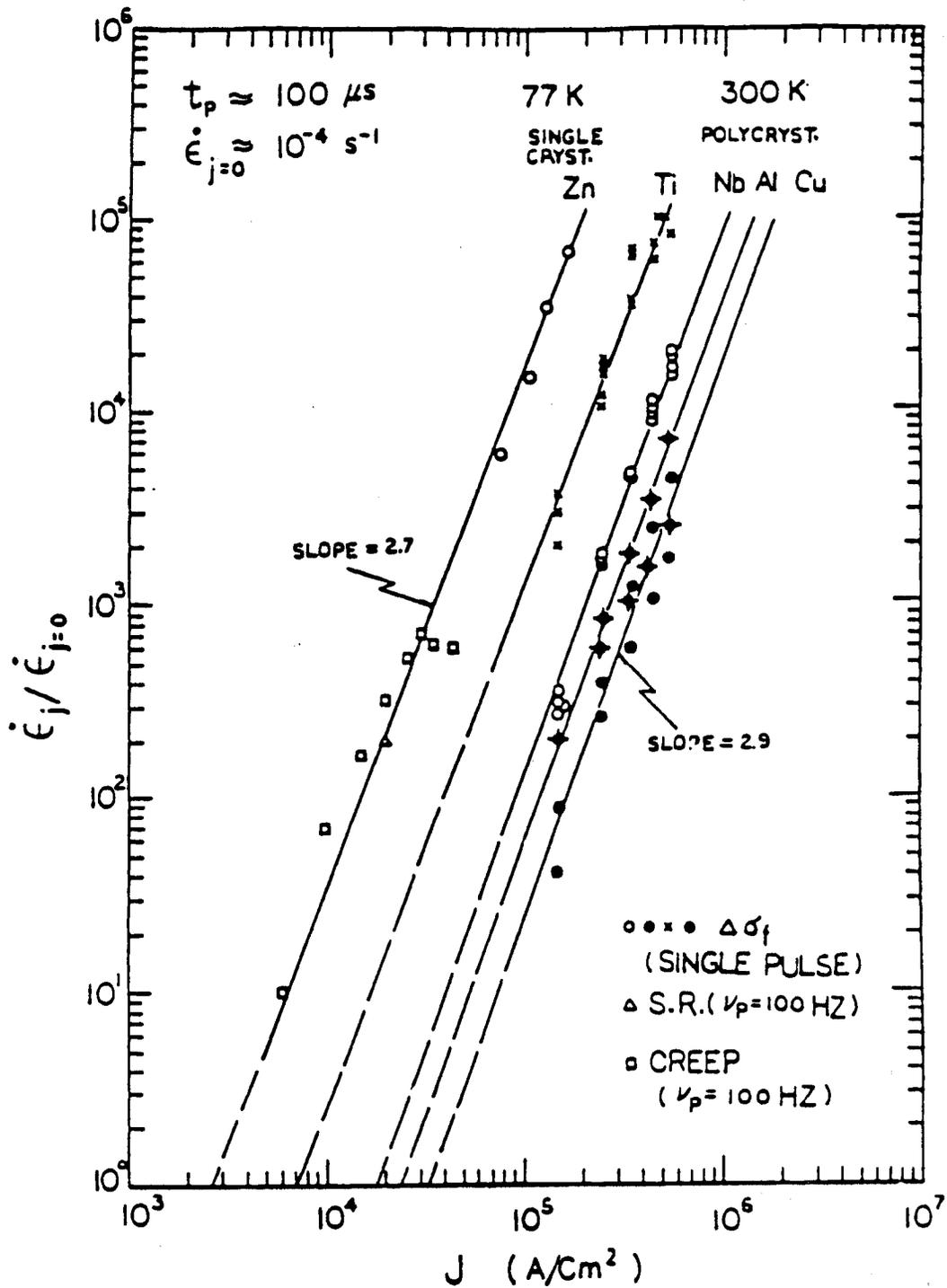
Fig. 2 - Log-log plot of the ratio of the plastic strain rate  $\dot{\epsilon}_j$  produced by an electric current pulse to the applied strain rate  $\dot{\epsilon}_{j=0}$  prior to the pulse for Zn single crystals at 78K and a number of polycrystalline metals at a 300K. Test methods include constant strain rate test to yield the drop in flow stress for a single pulse  $\Delta\sigma_f$ , stress relaxation S.R. and creep tests with 100 pulses per second.
