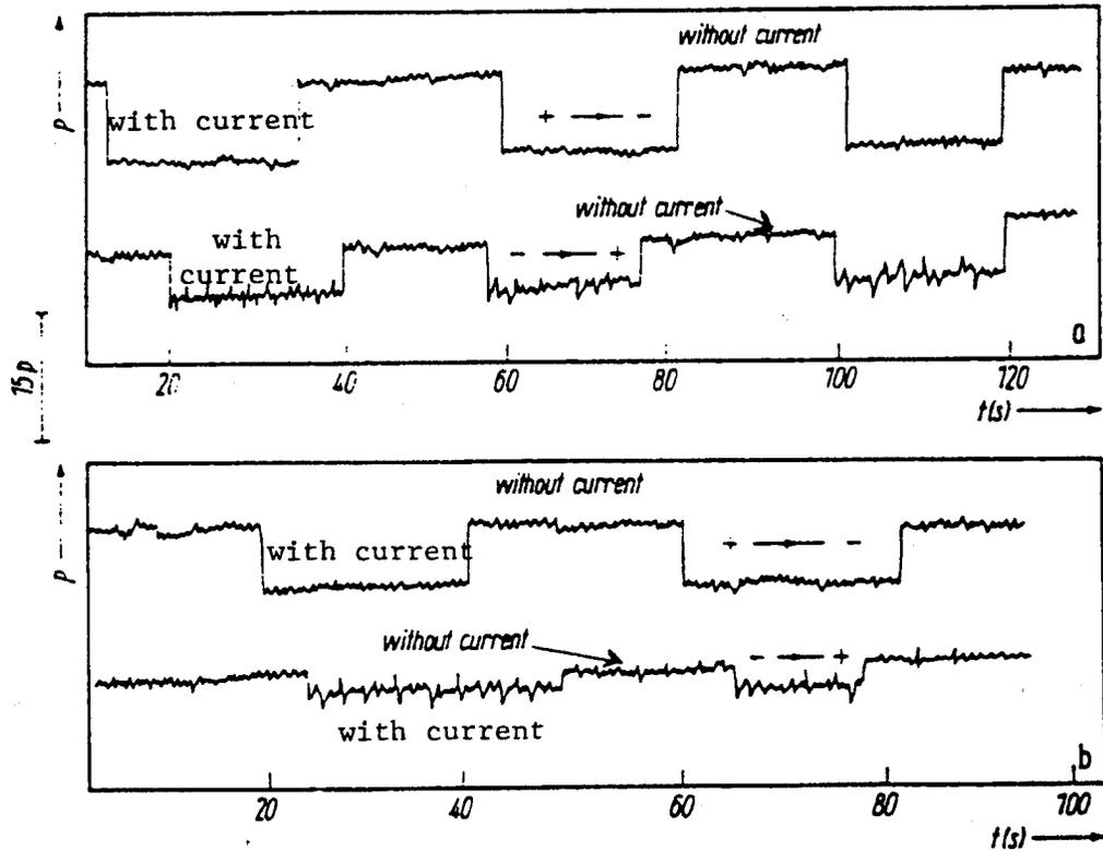
Fig. 4 - Typical diagrams of the drawing force reduction of copper wire 60  $\mu\text{m}$  in diameter with and without the application of an electric current to the deformation zone: mean effective current density  $J_{\text{mean,eff}} = 3.5 \times 10^5 \text{ A/cm}^2$ ; wire movement rate = 0.45 m/s; reduction ratio = 16.1%: (a) pulsed current with a frequency of 10 kHz and a pulse duration of 60  $\mu\text{s}$ ; (b) direct current with fluctuation not exceeding 10%.
