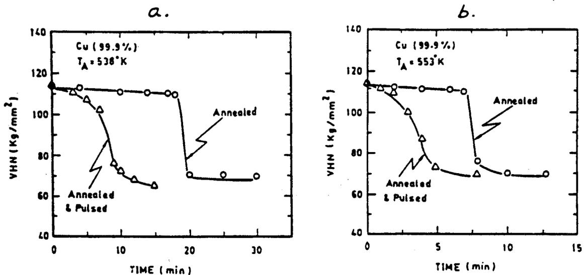
Fig. 6 - Effect of high density ( $j = 8 \times 10^4 A/cm^2$ ) electric current pulses ( $t_p = 90 \mu s$  and  $v_p = 2 Hz$ ) on the hardness of cold worked (~50% R.A.) copper wire vs annealing time: (a)  $T_A = 538K$  and (b)  $T_A = 553K$ .
