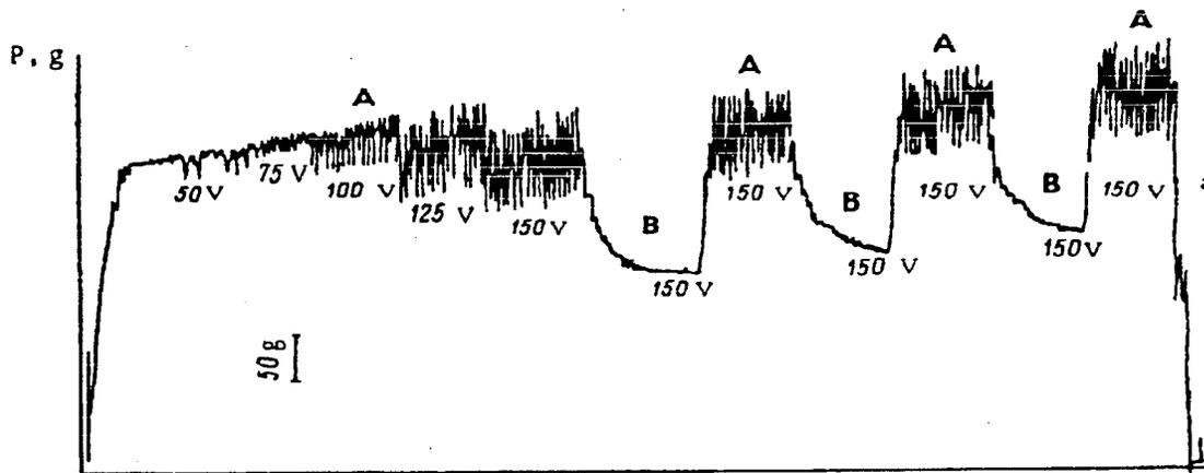
Fig. 1 - Load vs. extension diagram for a zinc crystal in uniaxial tension at 78K with a strain rate of  $1.1 \times 10^{-4} \text{ s}^{-1}$  showing load drops resulting from the application of d.c. pulses produced by discharging capacitors with the voltages indicated ( $100\text{V} - 1.5 \times 10^5 \text{ A/cm}^2$ ). Regions A correspond to constant extension rate. Regions B to stress relaxation (i.e., the test machine was off). From Troitskii (1).
