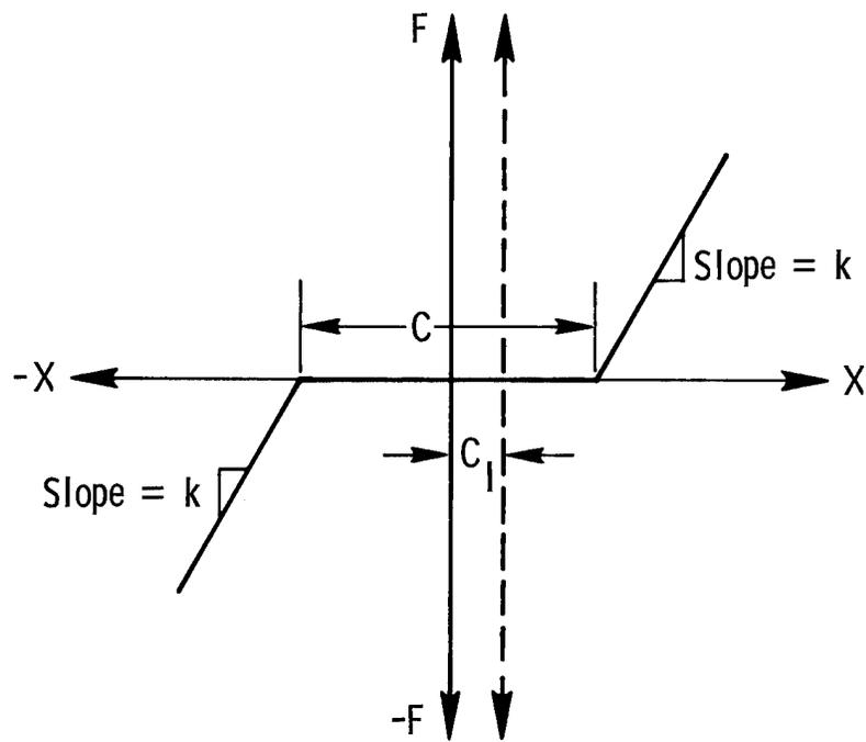
Figure 8. Load-deflection behavior with joint dead band.
