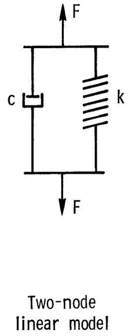
Figure 10. General models for joint simulations.
