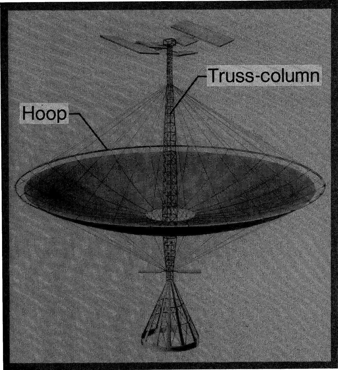
Figure 1. Hoop-column antenna.
