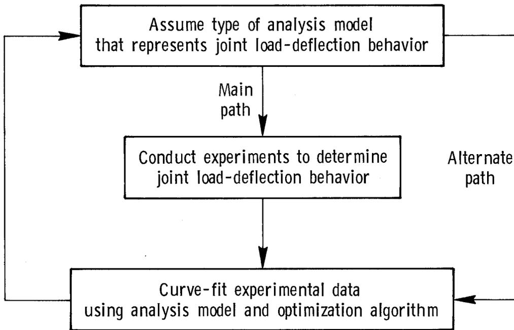
Figure 4. Flowchart for empirical joint model development.
