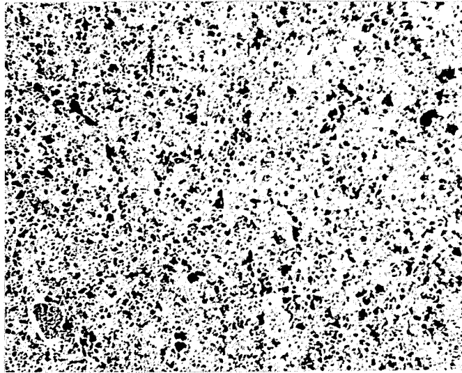
Figure 2. Photomicrograph of Rotating Band Blank Showing Representative Porosity. Unetched 100X
