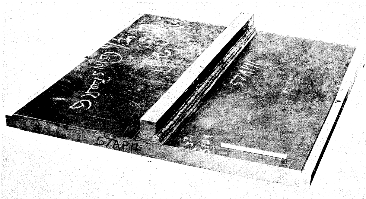
Figure 1. Tee-Welded Fatigue Specimen
