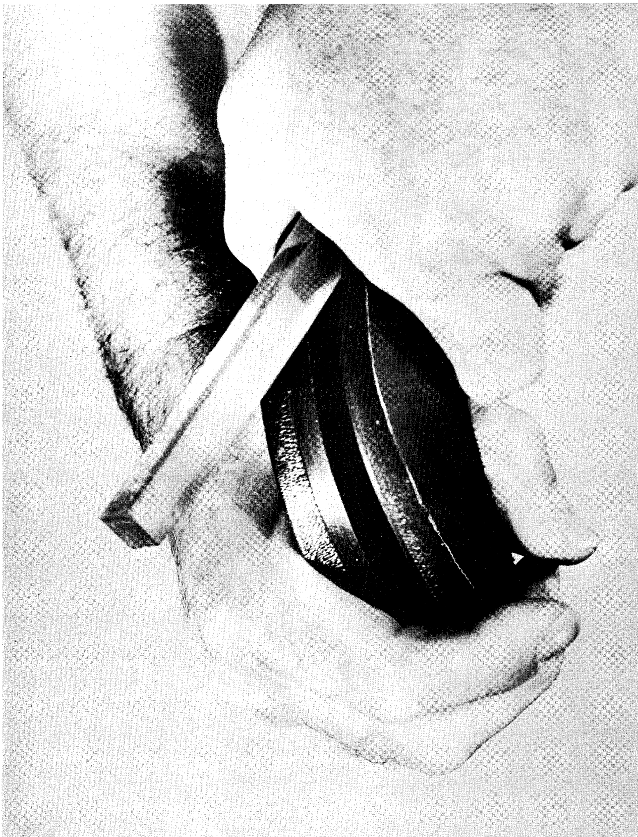
Photo #347. Flexible urethane molds are excellent for casting epoxies and phenolics. The "URALANE" 8118 shown above is a unique example. The removal of an epoxy part is illustrated.
