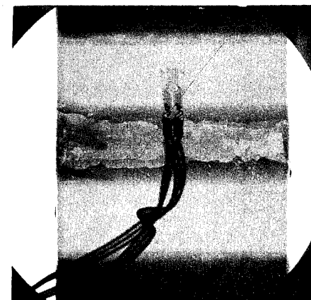
Figure 23. Delamination Growth in Specimen 4284-27; Laminate A; Test Series 4; S=0.47 .
