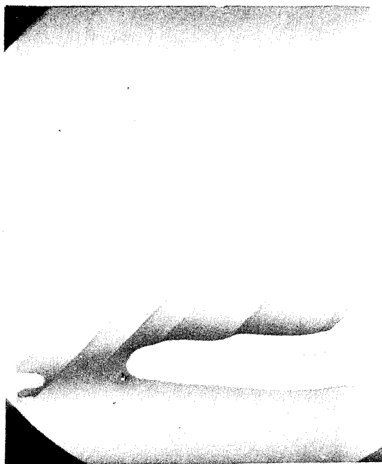
Figure 44. Delamination Growth in Specimen 4256-40; Laminate B; Test Series 14; S=0.66 ; Radiographs Taken with a 9.12 kN Load
